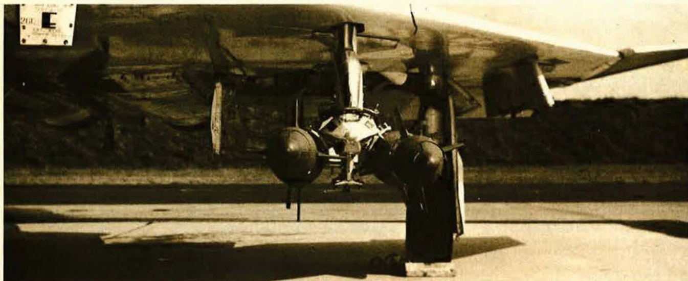
This laser guidance unit can be used with a variety of currently stocked bombs—a step toward the economy of modular munitions.
