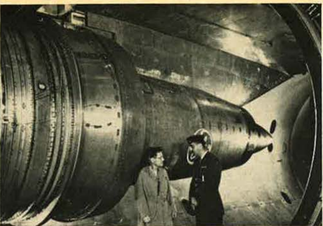
AFSC's Arnold Engineering Development Center sets up its J-1 high-altitude engine test cell, to qualify a GE TF39 engine for the Air Force's C-5 Galaxy transport program.
