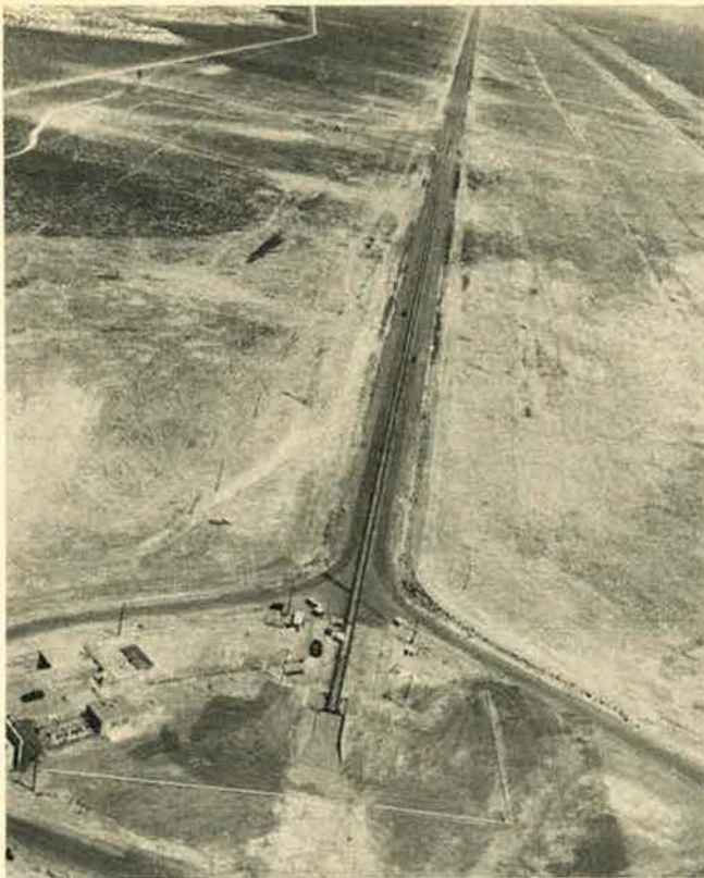
At Holloman AFB, N.M., is this 35,000-foot high-speed test track, an Air Force Missile Development Center facility that is in frequent use, testing the latest in equipment.
