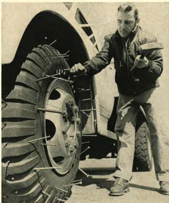
A new Goodyear tire shows that it can still function after suffering multiple punctures. It is being developed by Aeronautical Systems Division, Wright-Patterson AFB, Ohio.
