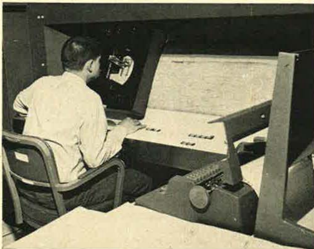
A civilian ACIC employee uses an automated name-placement machine in his cartographic work. It is one of many sophisticated pieces of equipment used by ACIC.
