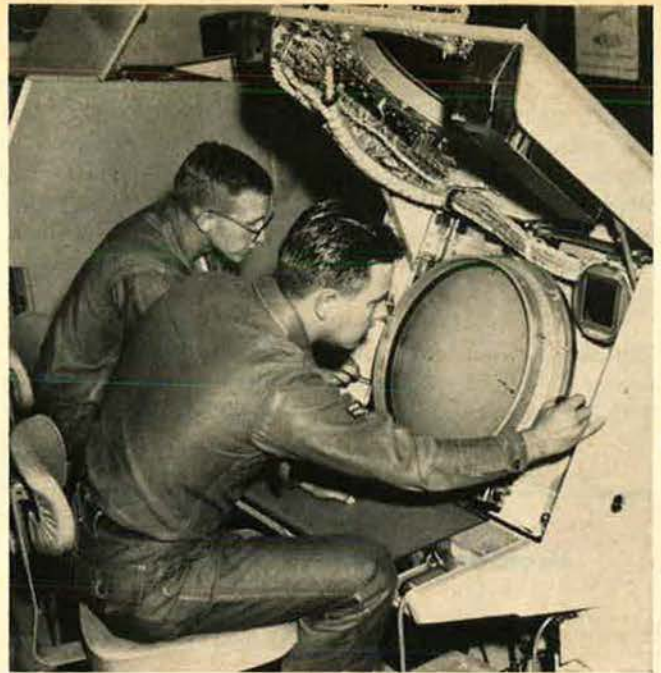
Students in ATC's Electronic Digital Data Processing Repairman course learning to adjust the cathode-ray tubes that are basic components of situation display consoles.
