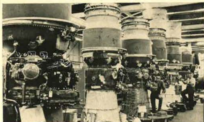
More than 100,000 pounds of thrust are represented in these six J57s at OCAMA's Jet Engine Overhaul Facility.
