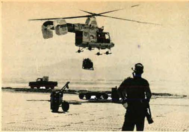
An HH-43 Huskie of the Aerospace Rescue and Recovery Service, with "Sputnik" fire-fighting equipment, takes off.
