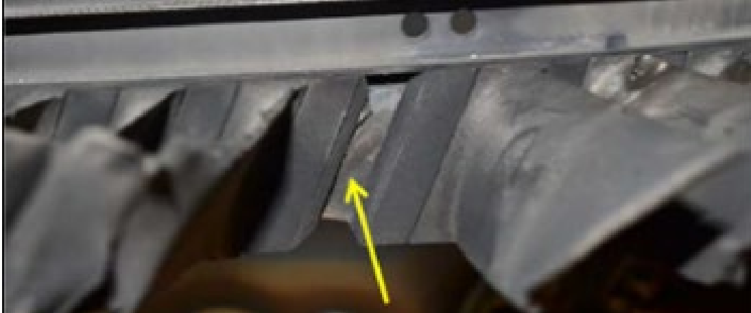
Figure 9. Fifth stage separated (or “fractured”) HPC blade (Tab J-75)
