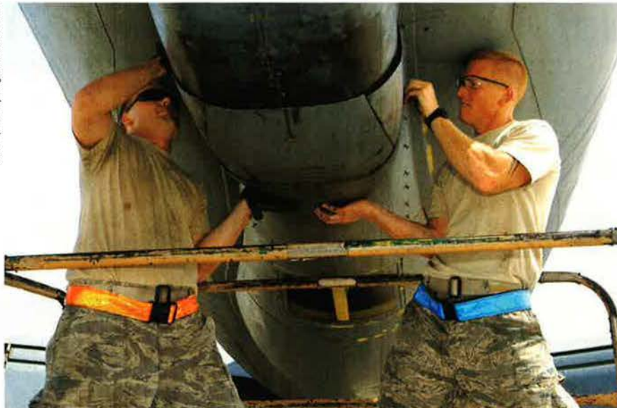
TSgt. Todd Clow (l) and SrA. Christopher Hughes anchor a boom pod fairing panel on a KC-135 tanker at a base in Southwest Asia.
