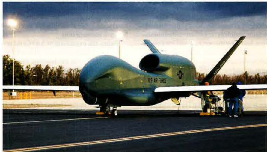
Maintenance workers prep a Global Hawk for a test mission. Global Hawks are rated Level Four on the Air Force's nine-level autonomy scale.
