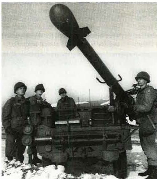
The Davy Crockett nuclear weapon could be launched from either a light vehicle or a stable tripod.
