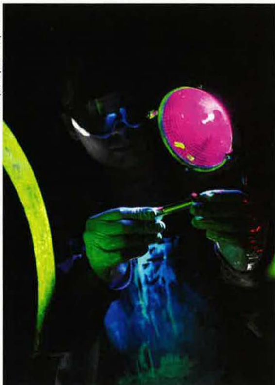
Left: SSgt. Richard Mabry carefully inspects a B-1 wheel bolt for cracks. Above: TSgt. Jesse Maddox installs an air-conditioning "splitter" on a B-1. The device allows the aircraft to only use one air-conditioning unit instead of several.
