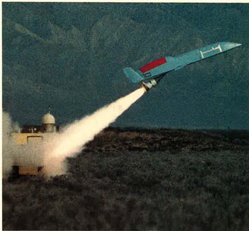
A Teledyne Ryan Model 324 Scarab UAV takes to the air from its ground launcher in the Mojave Desert. Egypt contracted with the US company to develop this remotely piloted jet aircraft. Twenty feet long with a twelve-foot wingspan, it can fly as fast as Mach 0.8 and deploys a parachute and an air bag to land.
