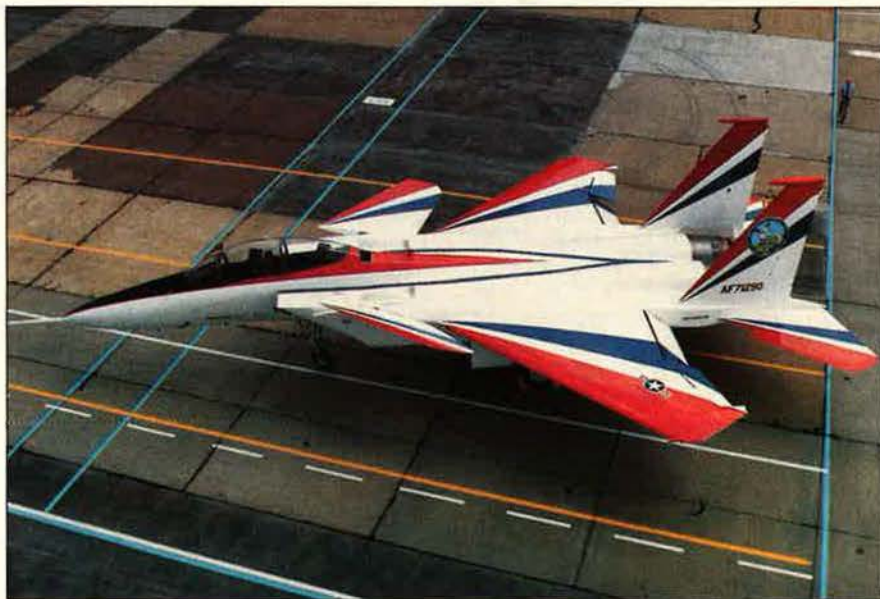
Resplendent in its new paint scheme, the McDonnell Douglas F-15B (short takeoff and landing) and Maneuvering Technology Demonstrator (SMTD) sits on the tarmac at the company's plant in St. Louis, Mo., prior to its first flight on September 7. The modified F-15B will go through a series of flights before being fitted with two-dimensional, thrust-vectoring nozzles later this year.
