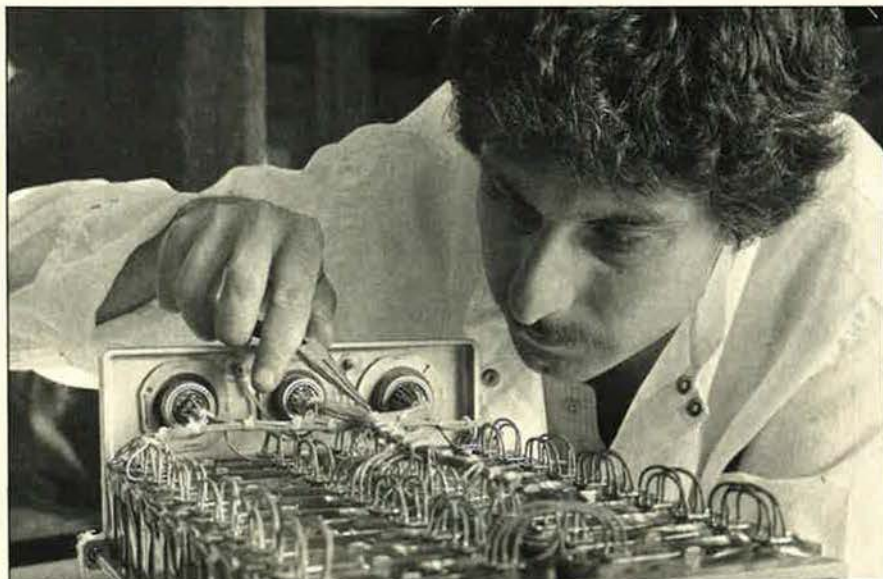
Lockheed electronic equipment mechanic Scot Vann tightens a wiring bundle on a solar-rechargeable satellite battery. Three of these batteries can provide all the electricity needed to operate a satellite. It takes two weeks to build one of these power packs in the company's Sunnyvale, Calif., plant.
