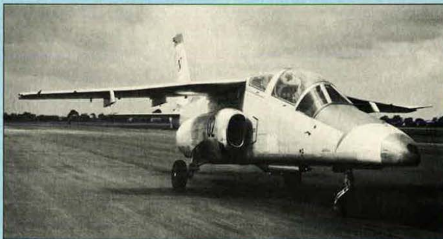
The PZL I-22 jet trainer and light attack aircraft is intended to replace the familiar TS-11 Iskra
