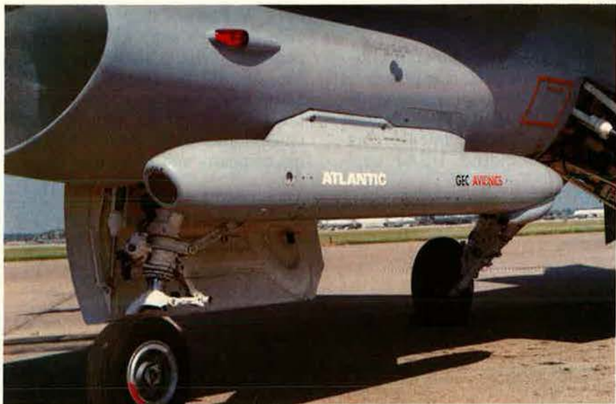
Transatlantic cooperation extends across a broad group of mission areas. One of those fields is in electro-optics, an example of which is this GEC Avionics's Atlantic FLIR (Forward-Looking Infrared) pod fitted to a USAF F-16B for compatibility trials. In addition to being mounted near the intake, the pod can also be fitted underwing.
