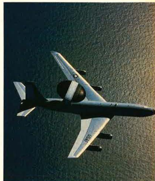
ABOVE: An Air Force operator keeps track of airborne traffic displayed in the OTH-B radar operations center at the Maine ANG base in Bangor. BELOW: E-3A Airborne Warning and Control System (AWACS) aircraft such as this will work with OTH-B radars and North Warning System (NWS) radars in the air defense mission.
