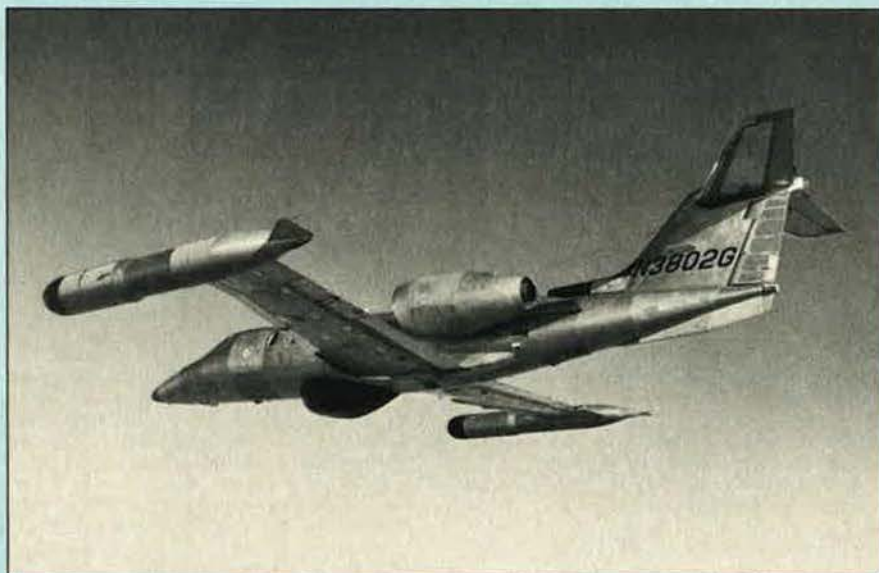
Enlarged wingtip tanks identify the customised Learjet U-36A supplied to Japan's Maritime Self-Defence Force. This aircraft can simulate sea skimming missiles in training missions against naval vessels
