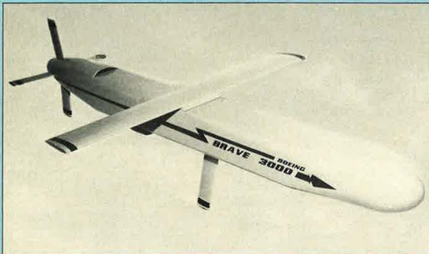
Boeing Brave 3000 in flight configuration, after jettisoning booster rocket
