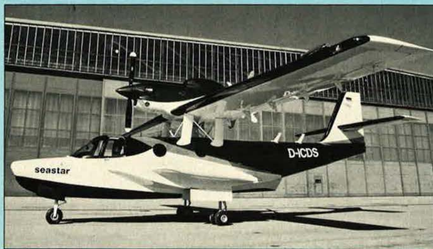
Claudius Dornier Seastar CD2 has an all-composites cantilever wing, instead of the strut-braced metal wing of the VT 01 prototype
