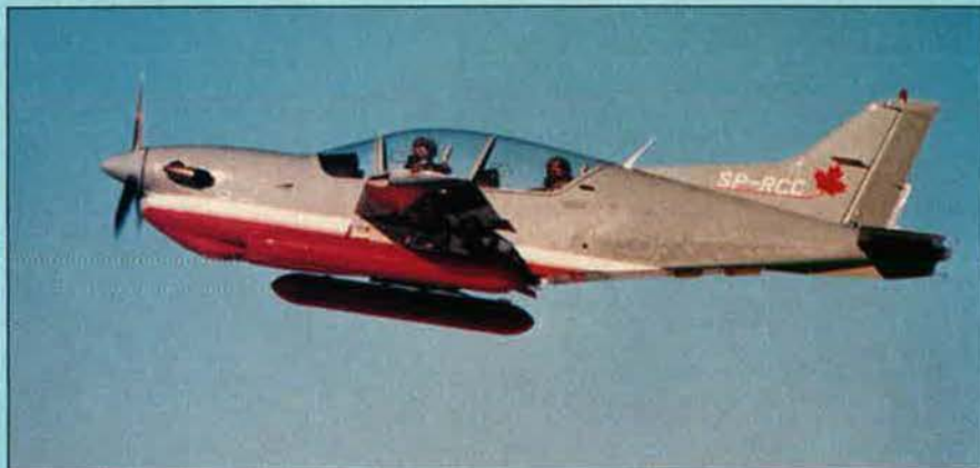
PZL Turbo Orlik basic and advanced trainer (Pratt & Whitney Canada PT6A-25A turboprop)
