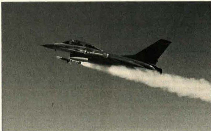
In early June, an AGM-45 Shrike antiradar air-to-surface missile was launched for the first time from an F-16. The test, part of a program to increase the F-16's defense-suppression capabilities, was conducted by the Air Force Flight Test Center at Edwards AFB, Calif. Maj. Tom Darner and Capt. Carl Walz crewed the mission, which was flown over the Naval Weapons Center at China Lake, Calif. (USAF photo by Tom Reynolds)
