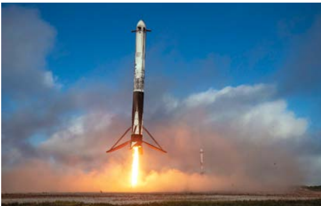
SpaceX's Falcon Heavy rocket uses twin, reusable side boosters, shown here landing after the system's first National Security Space Launch at the Kennedy Space Center's Space Launch Complex in, 2022. The rocket's two side boosters were used again in January 2023. The Eastern Launch Range is the only place the Falcon Heavy can operate today.
