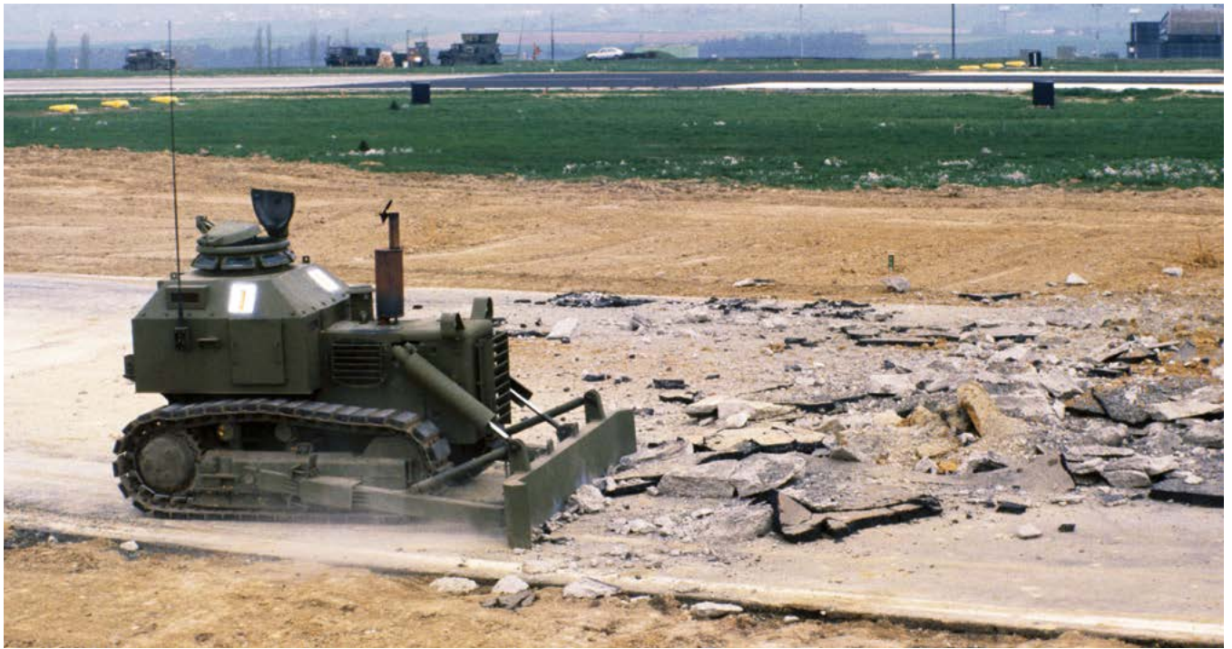
An armored bulldozer operated by the 7007th Explosive Ordnance Disposal Flight clears debris and unexploded ordnance from the runway after a simulated air attack during Exercise SALTY DEMO '85. Air base survivability exercises evaluate passive and active defenses, aircraft operation and generation, and base recovery systems.
