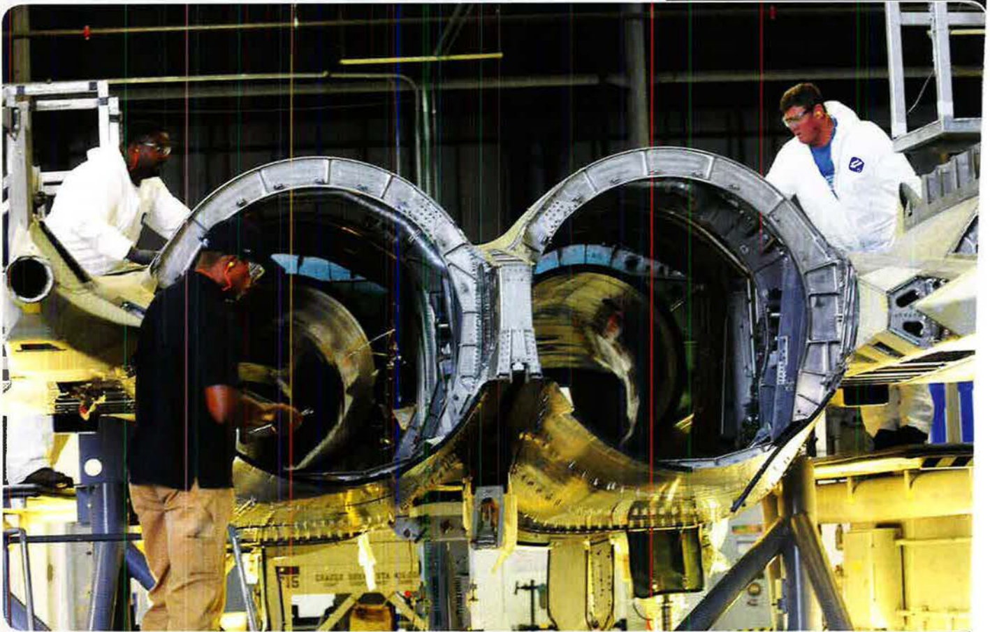
Civilian maintainers work on a replacement aft fuselage after the original one was damaged by a bird strike. Sequestration has caused a depot maintenance backlog that only time will clear.
