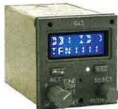
CMA-5025 Control Panel
