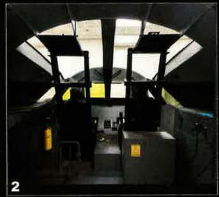
1/1 The Air Force named most B-2s after states, along the lines of the old Navy battleships. Here, AV-16, Spirit of Hawaii, is illuminated by ceiling lights in its custom hangar (both front and back doors are open for engine runs). 1/2 The B-2 egress trainer gives pilots periodic refreshers in how to exit the airplane in an emergency. It can be filled with smoke and has all the lights and caution signals of a real cockpit. That training was used only once, in 2008, when the B-2 Spirit of Kansas crashed in Guam. The pilots survived a low-altitude ejection without major injury. 1/3 Air traffic control apprentice A1C Chanel Johnson checks the runway from Whiteman's tower. 1/4 Call sign Dexter, the supervisor of flying, acts as the operations group commander's eyes and ears in the tower, monitoring weather and area flight ops. 1/5 Spirit of Hawaii looms in its hangar. 1/6 During an annual inspection, Spirit of Alaska has its stealth materials scrutinized by techs from the 509th Maintenance Squadron and the 131st Maintenance Squadron, an Air National Guard unit. On the fuselage are SSgt. Joshua Fleshman (left) and A1C Steven Sahn.
