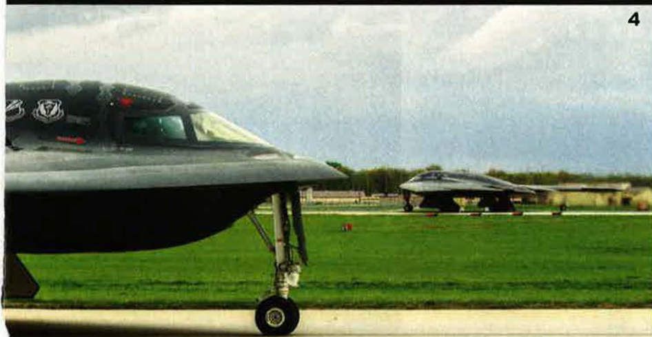
/1/ Spirit of Indiana lowers its landing gear. Having no vertical control surfaces, the B-2 relies on deflecting its tail/wing flaperons for yaw control. Seen deflected at the aircraft's rear, they can also function like a speed brake. Computers make the split-second calculations needed to keep the B-2 stable in flight. /2/ SrA. Steven Lee of the 309th Operations Support Squadron adjusts an oxygen mask for a waiting pilot. /3/ A1C Jared Schanen of the 509th OSS performs maintenance on a parachute to be carried in a T-38 ejection seat. /4/ Spirit of Indiana taxis as Spirit of Missouri, in background, starts down Runway One at Whiteman. /5/ Above the Truman Military Operating Area, a pair of 394th T-38s fly in formation.
