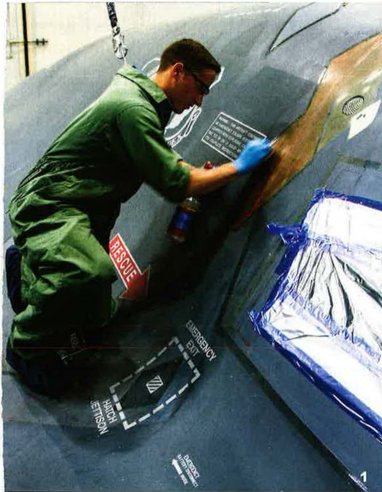
/1/ Sahd, a low observables tech with the 131st, applies stealth coatings. Note his boot covers, protecting the B-2's stealth finish. For large applications and repair, Whiteman has a specialized stealth coatings facility. /2/ The B-2s share Whiteman with A-10s of the 442nd Fighter Wing, an Air Force Reserve unit. /3/ The 394th's T-38s are serviced under sun shades on the tarmac. /4/ Spirit of Indiana and a T-38 chaser make a low sunset pass over Whiteman.
