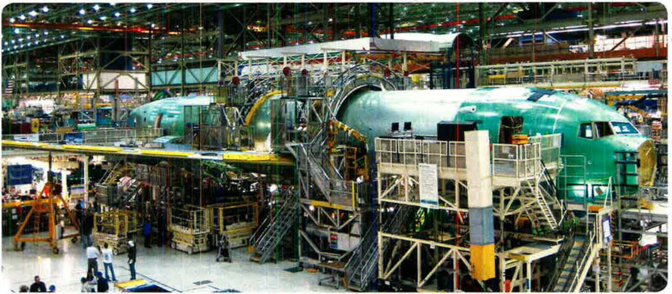
Major sections of what will be the first KC-46 are joined at Boeing's plant in Everett, Wash.
