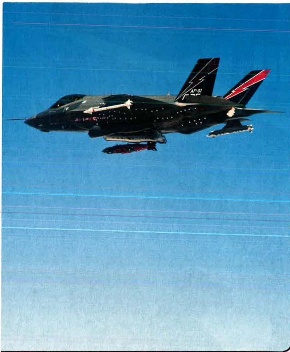
Maj. Eric Schultz, flying a conventional takeoff and landing F-35A (the Air Force variant), conducts a weapons separation test with a 2,000-pound Joint Direct Attack Munition at Edwards AFB, Calif.
