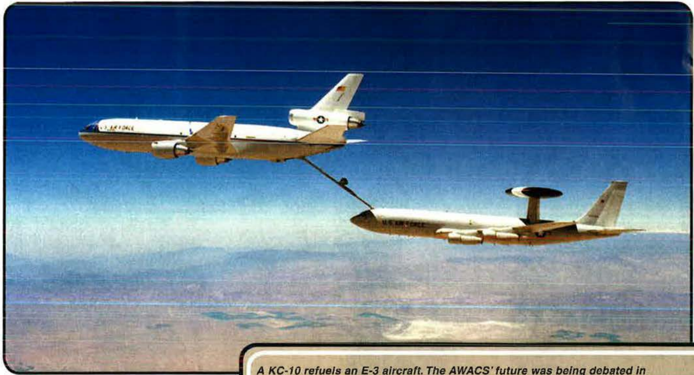
A KC-10 refuels an E-3 aircraft. The AWACS' future was being debated in Congress until Piotrowski recognized the potential of the concept to direct and control friendly aircraft and pushed hard to keep the airplane in the fleet.
