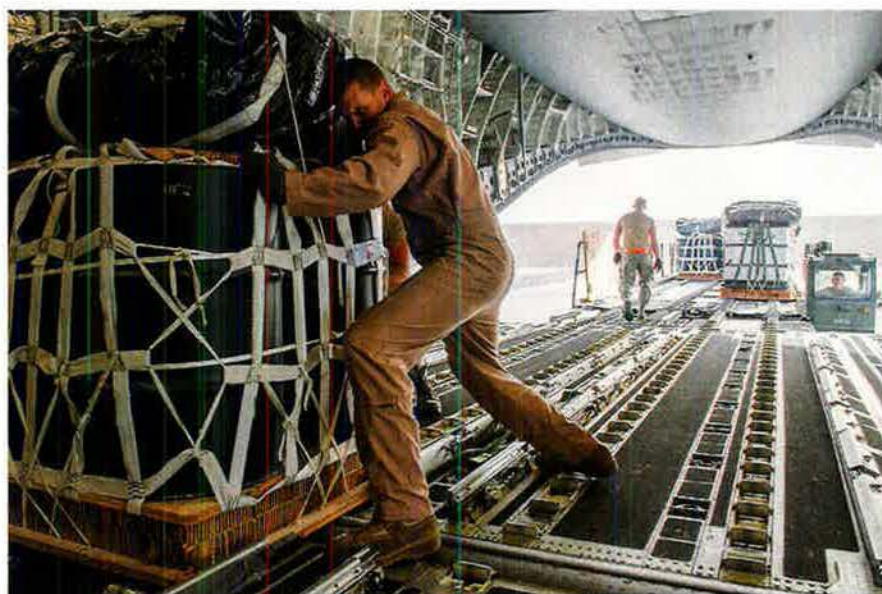
Step Right Up To See the Strong Man: SSgt. Travis Miller gives a pallet of supplies a strong heave-ho, aided by rollers in the C-17’s floor. Miller and other loadmasters were preparing the transport to airdrop cargo over Afghanistan. Miller is deployed from the 15th Airlift Squadron, JB Charleston, S.C.
