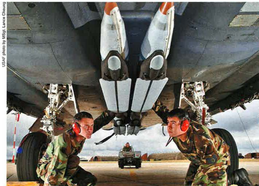
A1C Matt Aggers (l) and SSgt. Randy Broome check the stowed wings on ground-training Small Diameter Bombs loaded on an F-15E. The Air Force Operational Test and Evaluation Center was at the time evaluating the SDB weapon system.
