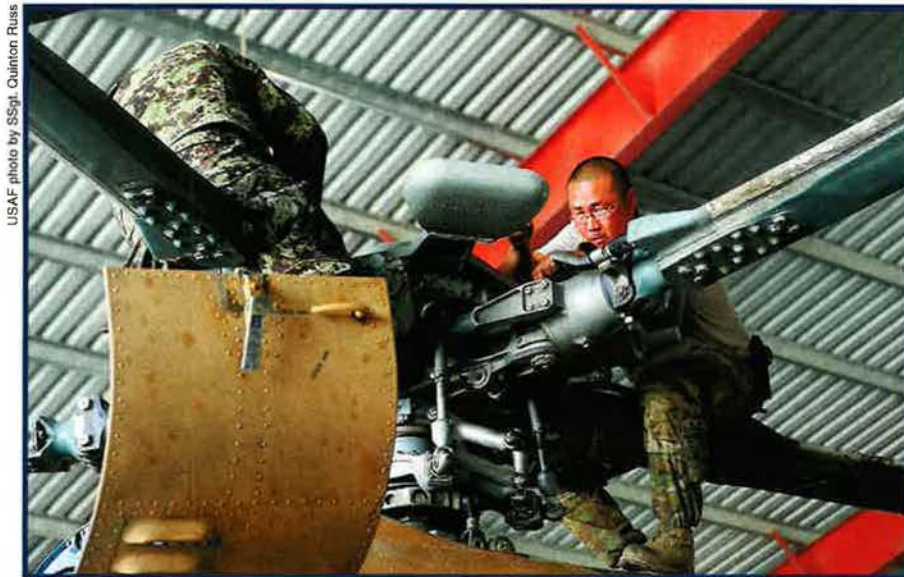
TSgt. Jin Yum (r) and an Afghan counterpart perform a seven-day inspection on the rotor of an Mi-17 helicopter during a NATO training mission in Afghanistan. After NATO passes off security responsibility to the Afghans in 2014, some US trainers will remain to try to bolster indigenous capabilities.
