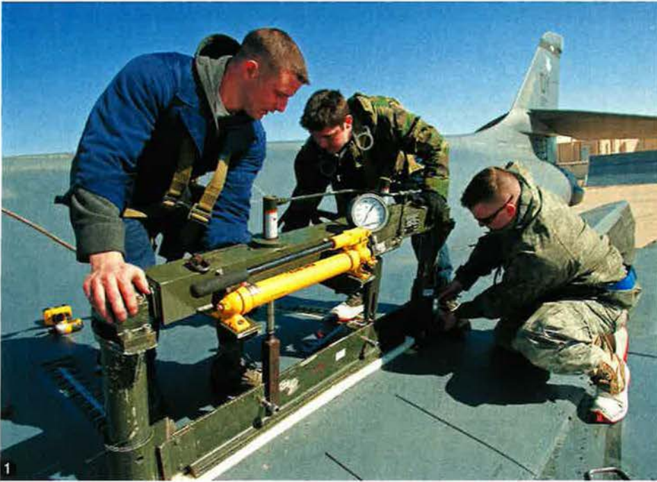
1 | (l-r) SrA. Jason Crane, A1C Jeremiah Jansen, and SSgt. Scott James, crew chiefs at Dyess, work on a B-1's wing carry-through spring panel. The aircraft has variable-geometry wings and employs its forward wing setting for takeoff, landing, air refueling, and some high-altitude weapons scenarios. For combat and high subsonic or supersonic flight, it uses the aft wing sweep configuration. 121 A 9th Bomb Squadron B-1 takes to the sky on a training mission from Dyess. The 7th Bomb Wing hosts the Air Force's only B-1 formal training unit.
