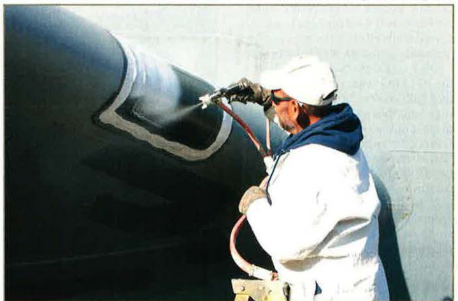
Top: It’s not just old airplanes. The tooling for the B-2 stealth bomber cockpit sits near retired bombers. A special treatment helps protect it from the elements. Above, Carlo Marinaz applies Spraylat to the forward edge of a KC-135’s wing.
