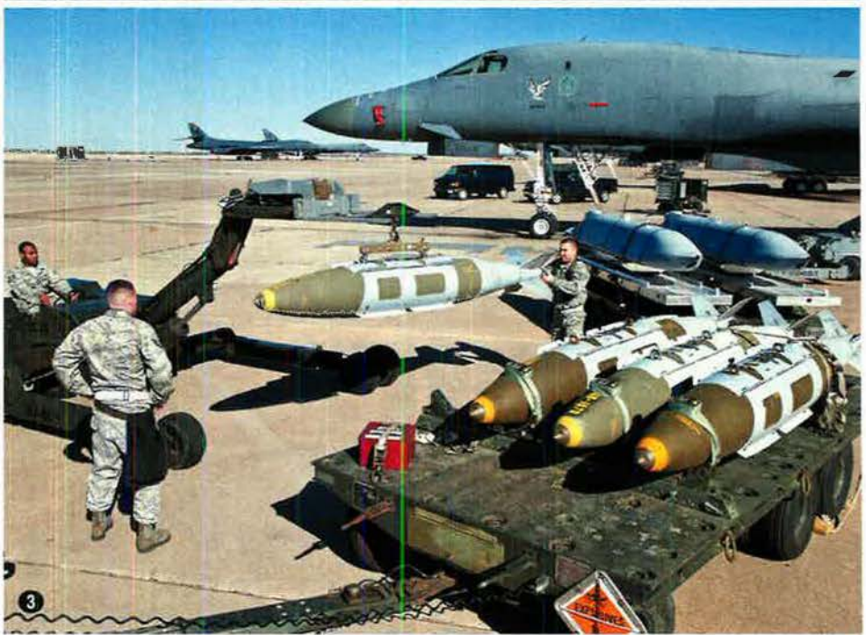
1| Capt. David Grasso demonstrates the Bone's power and agility, making a near-vertical climb over Texas in 2011. 2| A B-1B cruises over the New Mexico desert. 3| Taylor lifts a JDAM with a jammer as Rose (c) and Garza prepare to load the satellite guided bomb into a weapons bay. 4| The view from the cockpit as another Lancer lines up on the runway for takeoff.
