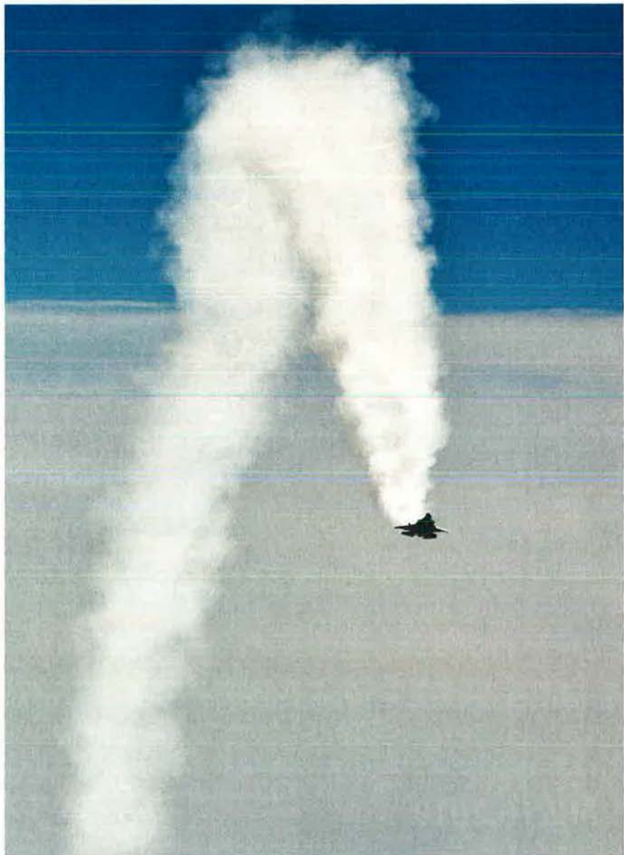
Opening the Envelope: Above, F-35 AF-4 is outfitted with a spin recovery chute at Edwards AFB, Calif. Testers have recently expanded the flight envelope of the conventional takeoff and landing variant with several high-angle-of-attack tests (right) including the first intentional departure from controlled flight on Dec. 4, followed by 50-degree angle-of-attack tests.
