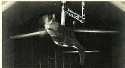
Model of FFA-2000 in wind tunnel at Swiss Federal Aircraft Factory
