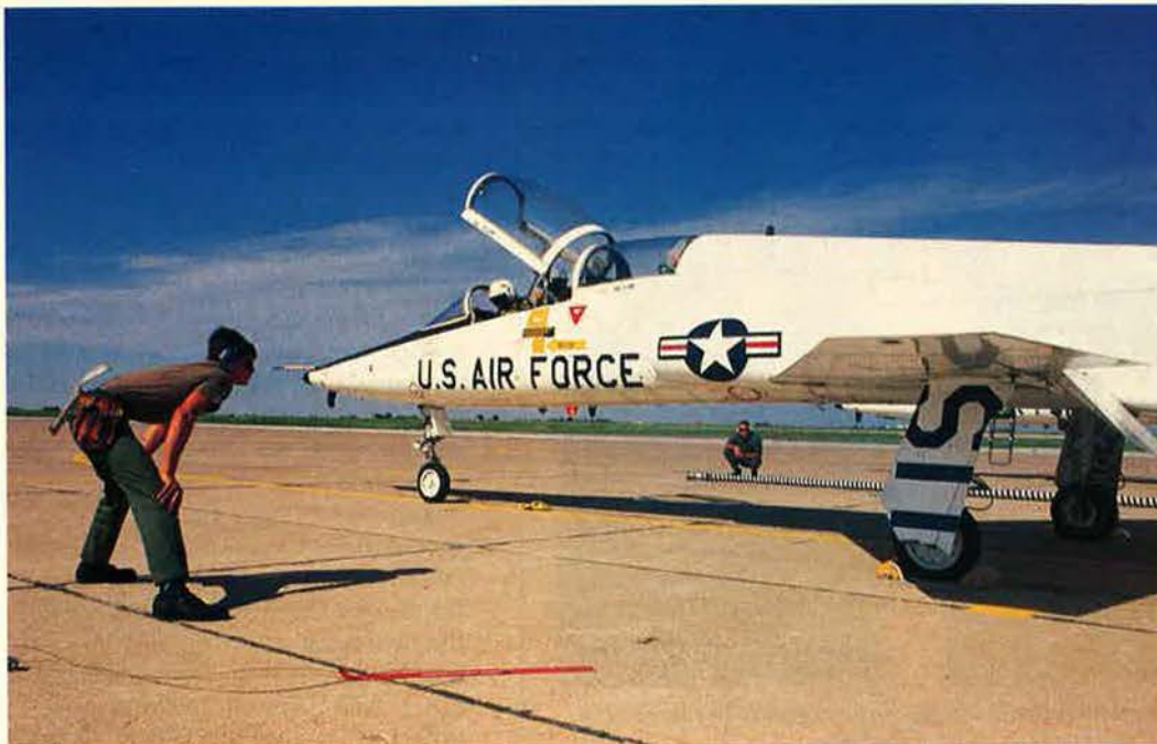
A1C James Rohlik (foreground) and SSgt. Mark Starsick do a flap-and-stab operation check before a T-38 launch. Both are assigned to the 64th OMS Eagle Flight at Reese AFB, Tex.
