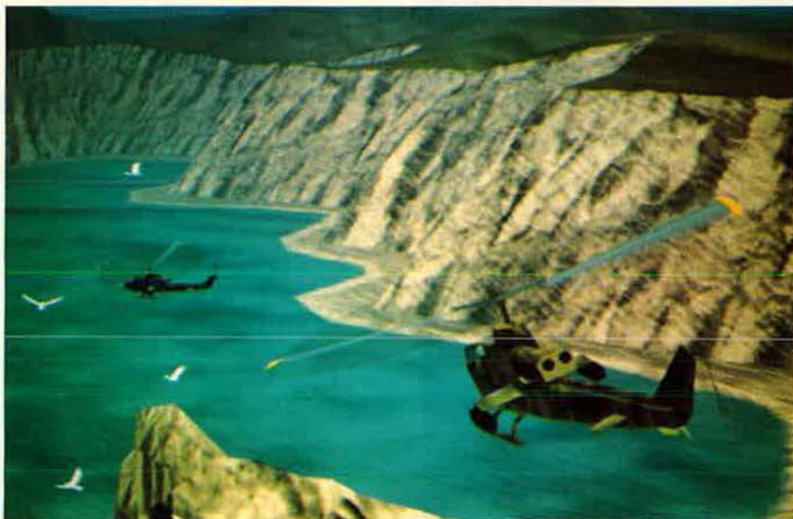
This picture of Marine AH-1Ws flying off the California coastline near Big Sur shows the level of realism computer-generated graphics have attained. High detail was required in this database to provide speed, altitude, and closure rate cues for the pilots in training while practicing low-level maneuvers near the cliffs.
