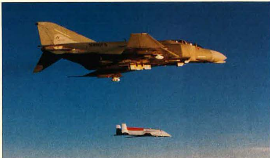
The first flight of the Teledyne Ryan Aeronautical Model 350 Joint Service Common Airframe Multiple Purpose System (JSCAMPS) unmanned aerial vehicle was completed on October 22. The UAV was recovered after a thirty-minute flight. The vehicle was launched from an F-4C operated by Flight Systems, Inc., at Mojave, Calif. The Model 350, a company-funded effort, was designed for both air and ground launching and is made of composite materials.
