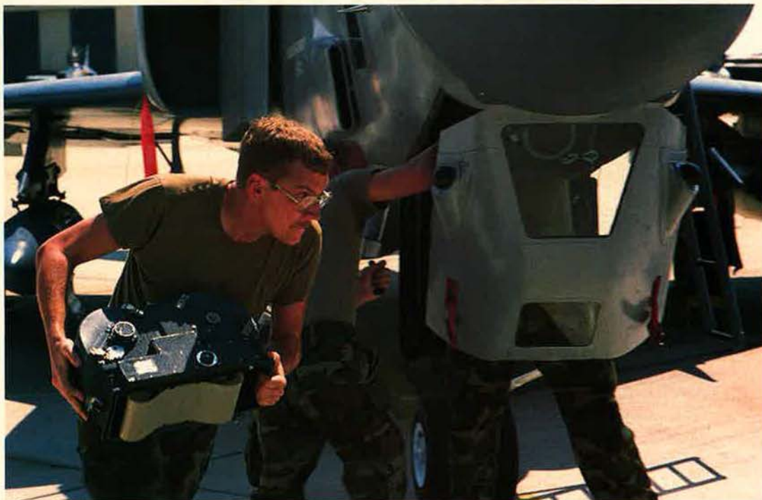
Sgt. Nick Horishny, SSgt. Jeff Morell, and SSgt. Tony Jordan of 363d TFW, Shaw AFB, S. C., download a camera after a daytime mission.
