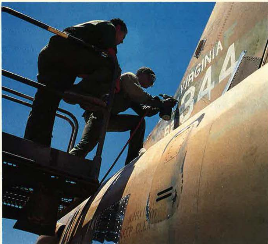
The last three days of the five-day technician's course are spent making actual repairs on the school's full-scale learning aids. Here, TSgt. Johnny Hines patches the tail of an F-105 while Sgt. Terry Hubbard observes. Eventually, the school's instructors run out of places to create new damage.
