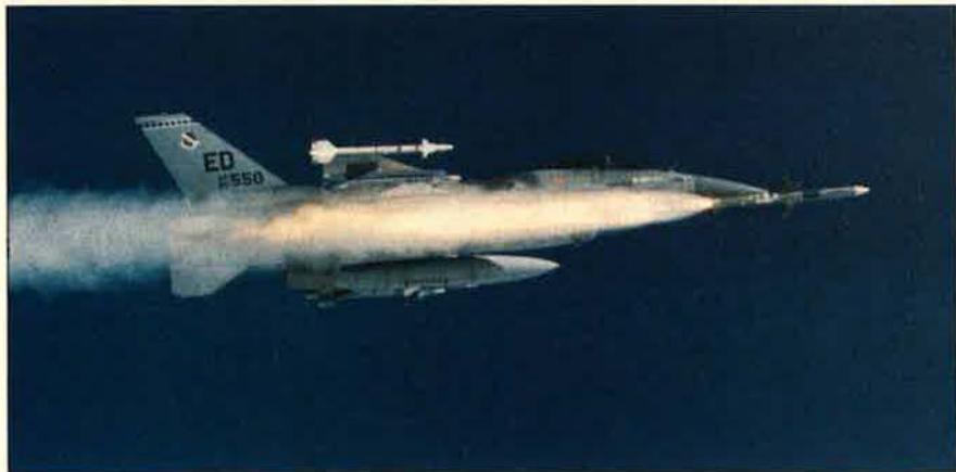
The first launch of an AIM-7 Sparrow radar-guided missile from an F-16 took place in October. This launch was the first in a series of thirteen unguided and guided Sparrow shots from an F-16. The addition of AIM-7s will give the F-16 a beyond-visual-range (BVR) capability. The first AIM-7-capable F-16 is scheduled for February delivery.
