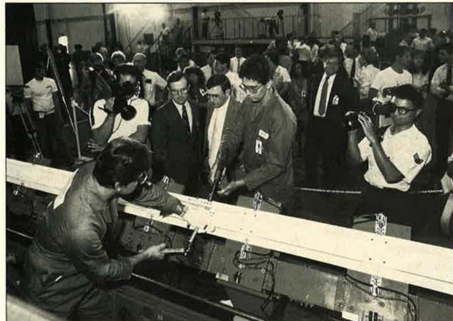
Ernest O'Campo (foreground) and Steve Ybarra (opposite O'Campo) begin assembly of the first McDonnell Douglas C-17 airlifter at the Douglas plant in Long Beach, Calif., on August 24. This initial component, a sixty-eight-foot-long tiedown rail, is the central structural member of the airlifter's cargo floor.
