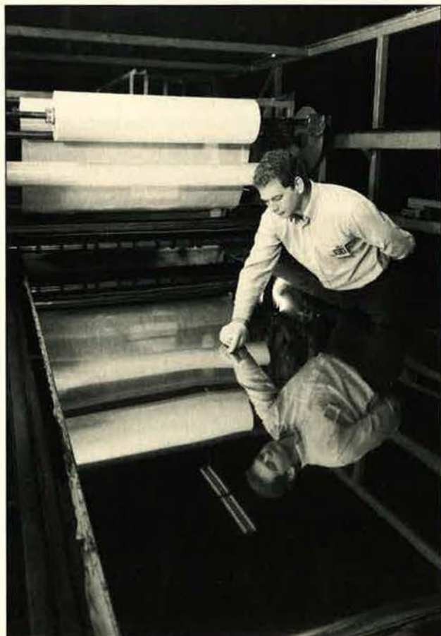
LTV has developed a unique system that applies a protective coating to keep commercial airliner parts unmarred during the manufacturing process. Before the introduction of the new applicator, which saves money and time, technicians either used a cumbersome tape machine to apply the plastic film or applied it by hand.
