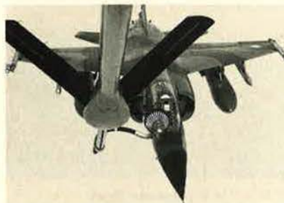
Mirage F1-CR-200, carrying Magic missiles and countermeasures pods, being flight refuelled (SIRPA "AIR")
