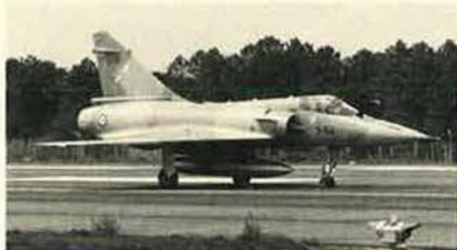
Mirage 2000C, with M53-P2 engine and RDI radar (SIRPA "AIR")
