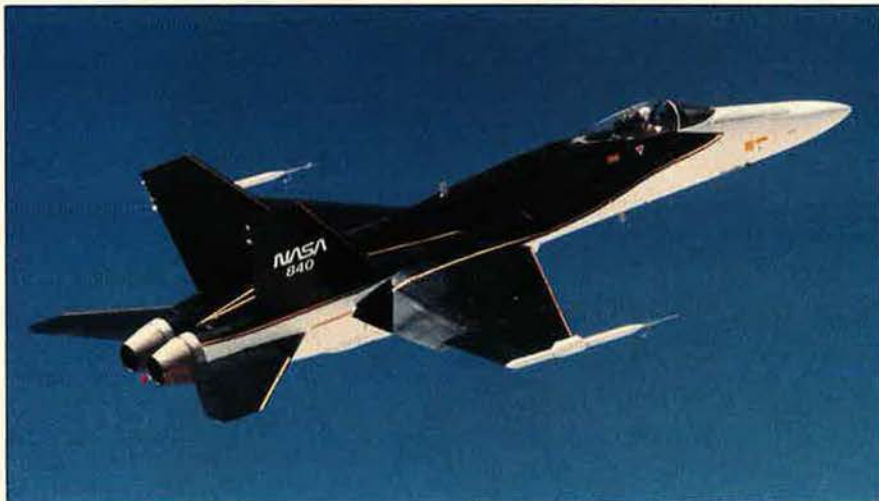
NASA's Ames-Dryden Flight Research Facility has begun its High Alpha (high angle of attack) research program with this specially equipped and instrumented F/A-18 on loan from the Navy. The program will investigate airflow in high angle of attack attitudes, nose-high flight relative to flight path, and post-stall maneuverability assisted by thrust vectoring. The High Alpha program will run until 1992.
