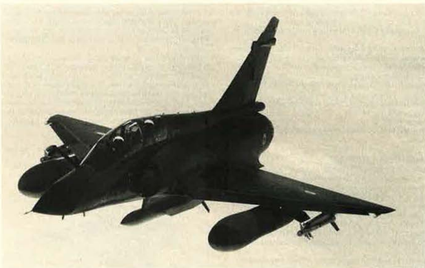
ASMP and two Magic missiles on Mirage 2000N (SIRPA "AIR")
