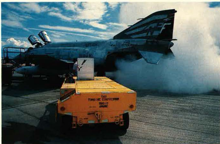
After an airplane is thoroughly examined and washed, it is defueled, and its fuel system is refilled with a lightweight lubricating oil. After several minutes of engine runup, the oil is drained, leaving a thin, preservative oil film in the aircraft's engines and systems. Shown undergoing this preservation step is a Navy F-4S, one of several versions of the venerable Phantom II now coming into the Center.
