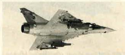
Two Magic and two Super 530 D air-to-air missiles on Mirage 2000C (SIRPA "AIR")
