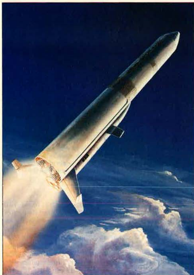
This is an artist's conception of the Martin Marietta/McDonnell Douglas Advanced Launch System (ALS) vehicle that will be capable of lifting eighty tons of payload into low earth orbit. Boeing and General Dynamics are the other two contractors selected to continue into Phase II of the ALS development effort.
