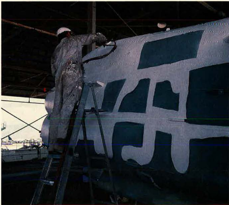
Before the aircraft are taken out to the desert for storage, they undergo a thorough preservation process. In AMARC's 600-foot-long reclamation shelter, technicians seal a plane's canopies, radomes, and most of the openings and seams with barrier paper, tape, and a material called Spraylat. Here, George Foss, a storage servicer, puts a final coat of white Spraylat on a Navy A-7.
