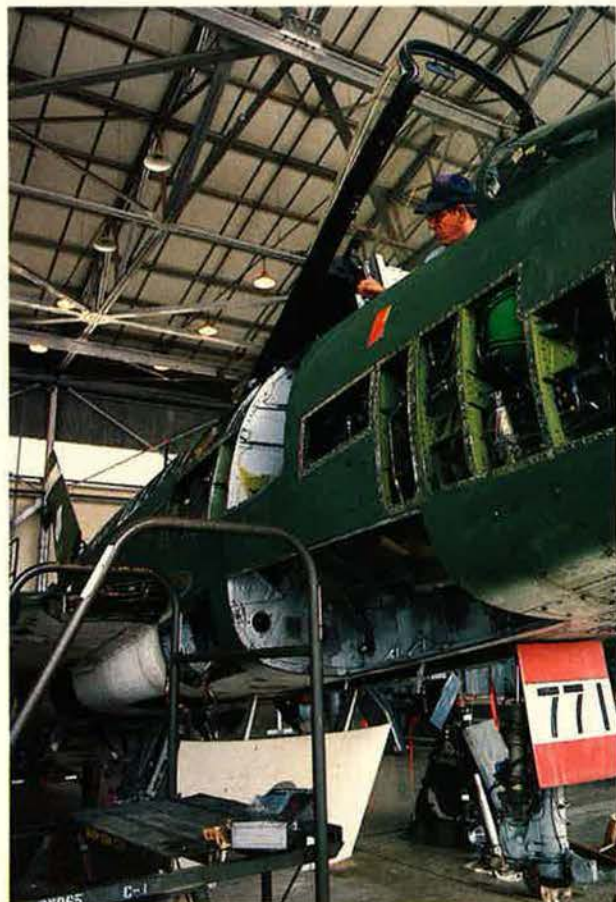
AMARC's biggest removal effort is the F-100 drone program. The aircraft, some of which have been stored for up to thirteen years, are disassembled, checked, and put back together. It takes roughly 1,900 man-hours to bring the F-100s back up to flight status, as Willard Wilkinson is doing here. Once completed, the aircraft are flown to Mojave, Calif., where they are converted into drones.
