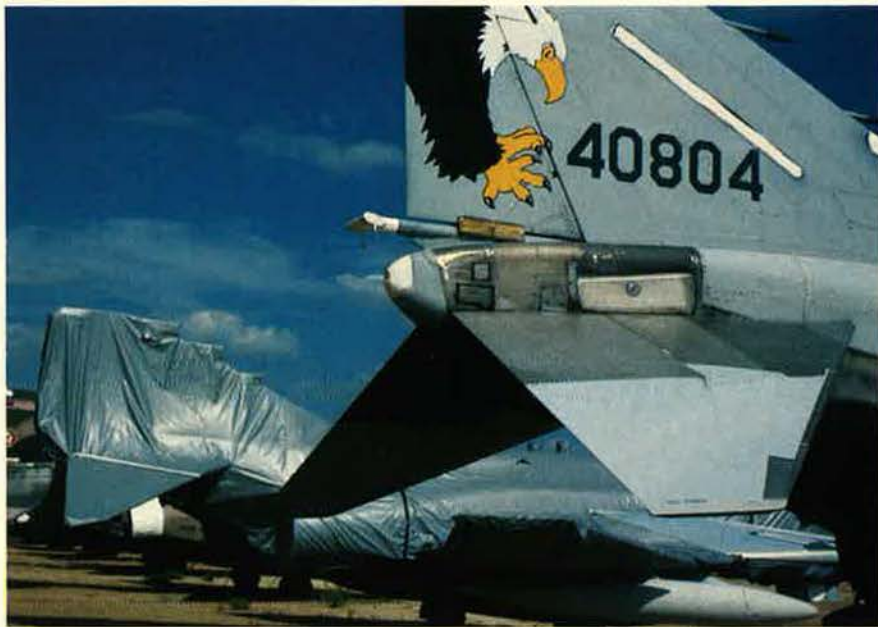
AMARC's materials laboratory is always looking for better and less expensive ways to do things. The F-4 in the background has been "bagged"—an alternative preservation method now under study. The F-4 in the foreground has been preserved with Spraylat.
