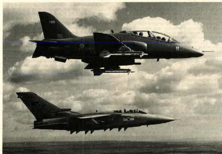
Sidewinders on a Hawk T. Mk 1A flying in company with a Tornado F. Mk 3 armed with Sky Flash missiles
