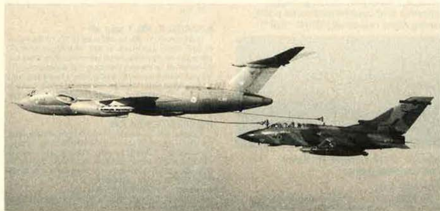
Victor K. Mk 2 of the Royal Air Force refuelling a Tornado GR. Mk 1
