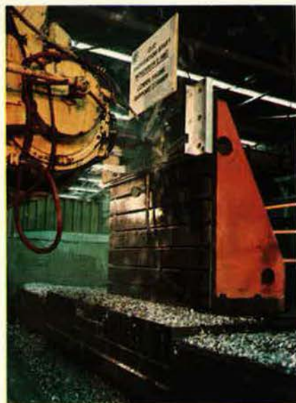
The first part for the C-17 was machined at the Douglas facility in Torrance, Calif., in early November of last year. The lower frame support corner, a part that supports the edge of the cargo floor where it joins the fuselage, weighed 9.61 pounds after being milled out of a 170-pound block of aluminum. The part, along with the remainder of the big airlifter, will roll out in July 1990.
