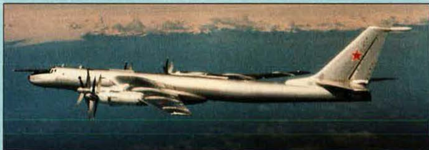
'Bear-F' Mod 3 introduced an MAD boom at the fin tip
