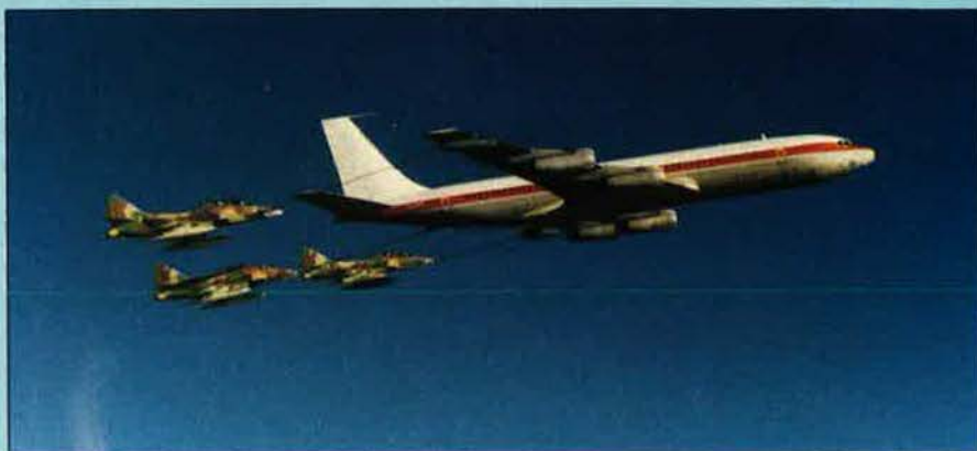
Bedek conversion of a Boeing 707 to three-point probe-and-drogue tanker with A-4 Skyhawks
