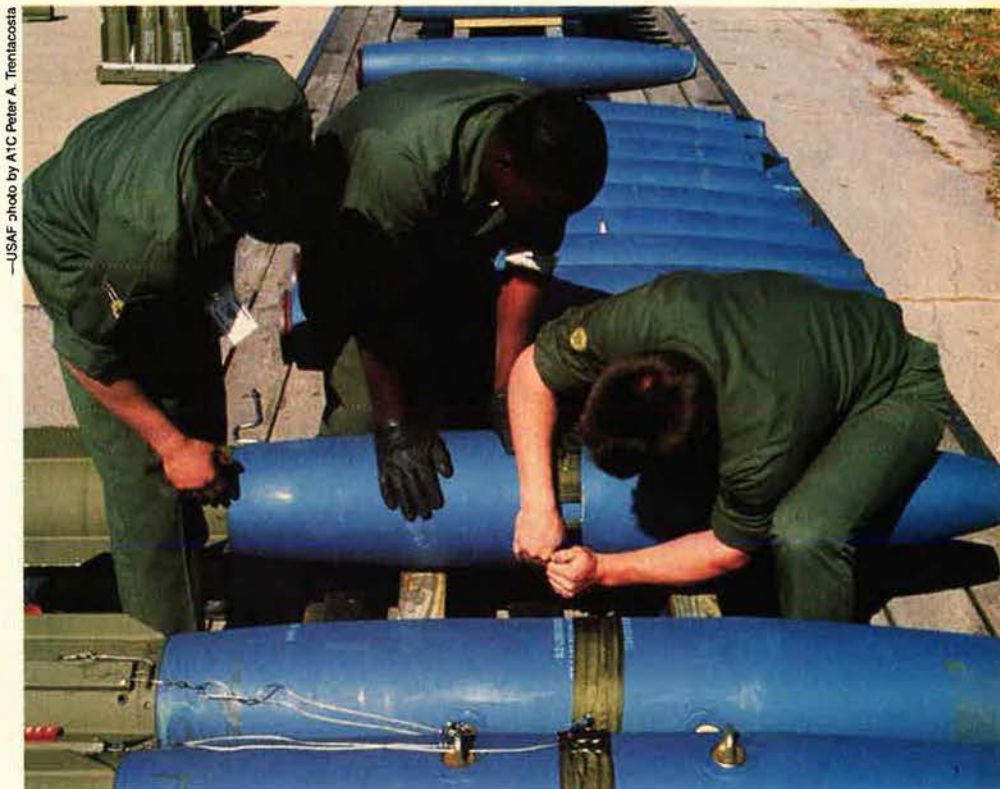
This is no drill. These maintenance troops are preparing these BDU-50 practice bombs for an actual drop. A1C Scott L. Bewkes (right) is installing a "belly band," a piece of equipment that allows the bomb to clear the bomb bay before its "ballute" opens. Airman Bewkes is being assisted by Sgt. Richard Espinoza (left) and A1C Eric L. Rose.
