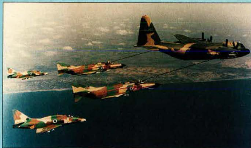
Israeli Air Force Skyhawks and Phantoms queue to refuel from a Bedek converted C-130 tanker
