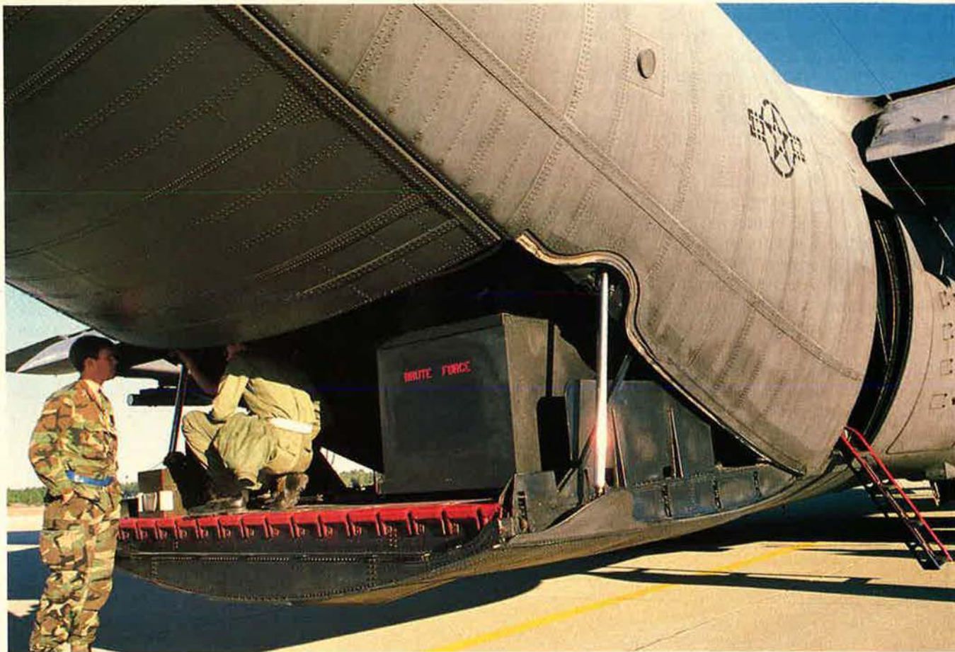
ABOVE: The odd combination of vacuum tubes and digital electronics on the AC-130s makes life tough sometimes for the maintenance troops (two of whom are shown above during a preflight inspection). BELOW: One of the most important pieces of equipment on a gunship is a snowshovel. Because of the high rate of fire of the 20-mm guns, one of the gunners has to clear the brass and links from around the gun breeches while they are firing to prevent the guns from jamming.
