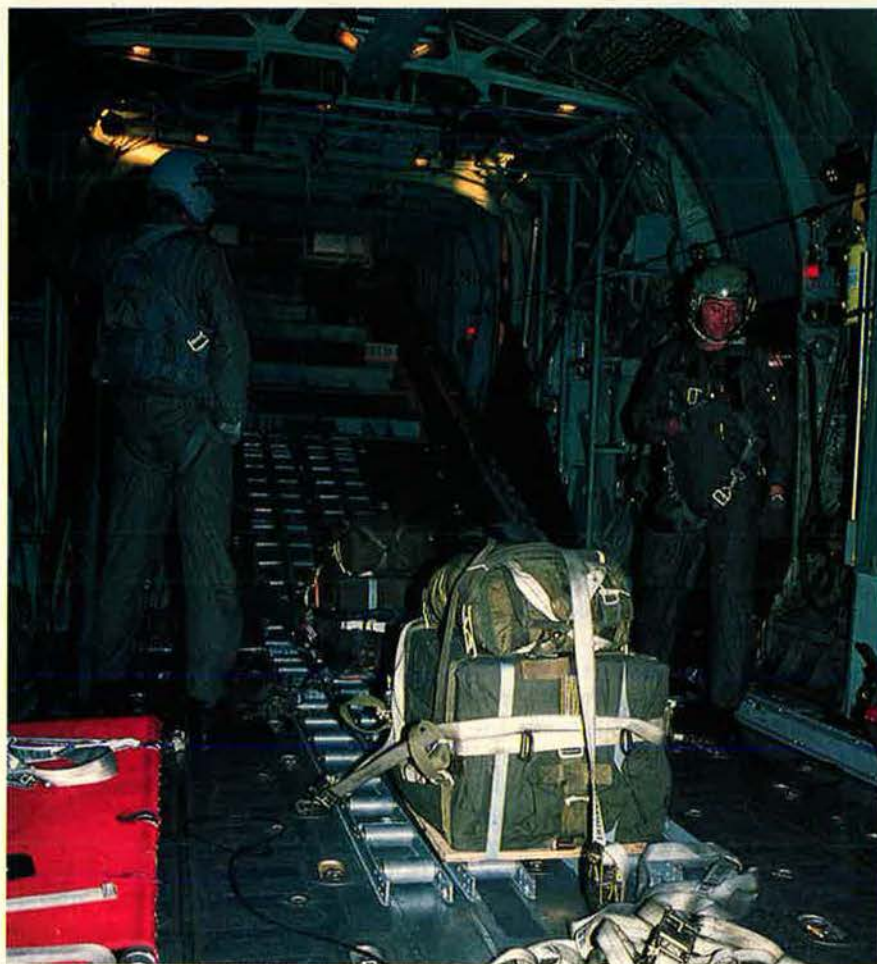
These MC-130E loadmasters are starting to prepare two High-Speed Low-Level Aerial Delivery System (HSSLADS) pallets for a drop at low altitude. Once rigged, the pallets will be catapulted off the rollers by means of industrial-size bungee cords. The MC-130E has a specially modified back end to allow for the HSSLADS drops. This system and the Combat Talon's extensive navigation suite allow for cargo drops on the top of a mountain, if need be.
