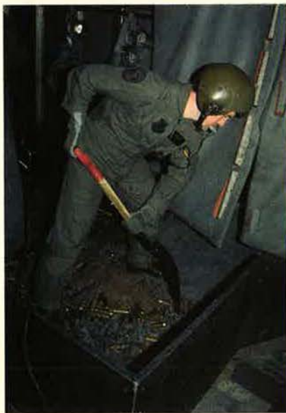
ABOVE: The odd combination of vacuum tubes and digital electronics on the AC-130s makes life tough sometimes for the maintenance troops (two of whom are shown above during a preflight inspection). BELOW: One of the most important pieces of equipment on a gunship is a snowshovel. Because of the high rate of fire of the 20-mm guns, one of the gunners has to clear the brass and links from around the gun breeches while they are firing to prevent the guns from jamming.
