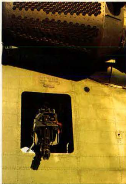
RIGHT: The Sikorsky MH-53 Pave Low helicopters have an automatic hover feature and are navigated by means of a forward-looking infrared system and a terrain-following radar (part of which can be seen in the cigar-like projection on the nose). BELOW: Because they will have to go into Bad Guy country, the MH-53s are armed with a pedestal-mounted 7.62-mm minigun (as shown here) or .50-caliber machine guns.
