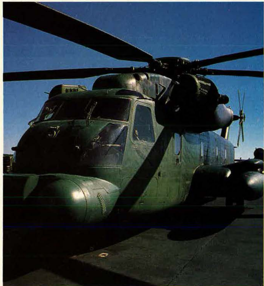
RIGHT: The Sikorsky MH-53 Pave Low helicopters have an automatic hover feature and are navigated by means of a forward-looking infrared system and a terrain-following radar (part of which can be seen in the cigar-like projection on the nose). BELOW: Because they will have to go into Bad Guy country, the MH-53s are armed with a pedestal-mounted 7.62-mm minigun (as shown here) or .50-caliber machine guns.
