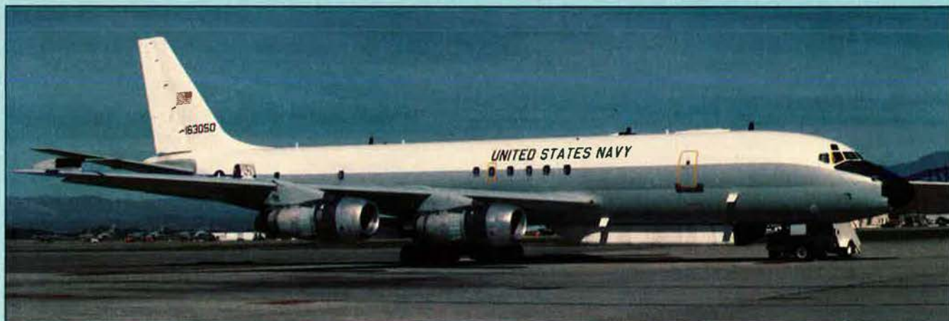
EC-24A conversion of a McDonnell Douglas DC-8-54 for fleet electronic warfare support group missions
