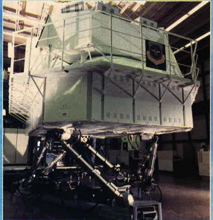
C-5B weapon system trainer developed by CAE Electronics Ltd.
