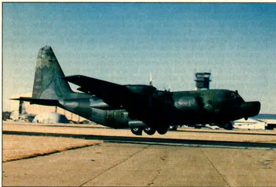
The Air Force's new MC-130H Combat Talon II special operations airlifter was introduced on March 14 in ceremonies at the E-Systems plant in Greenville, Tex. At the heart of these Improved Combat Talons is the IBM-developed avionics suite. The aircraft are new-build Lockheed C-130H aircraft.
