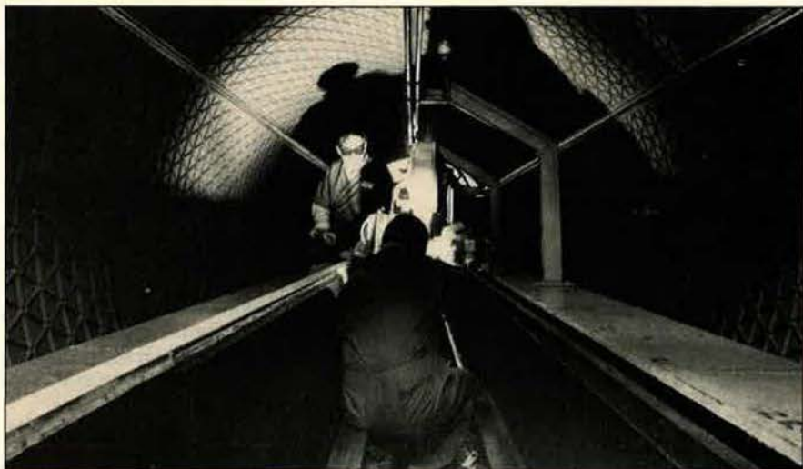
McDonnell Douglas will build an upgraded version of the reliable Delta rocket as USAF's new Medium Launch Vehicle (MLV). These workers at the company's Huntington Beach, Calif., facility are welding the liquid oxygen tank for a Delta to be launched next fall.
