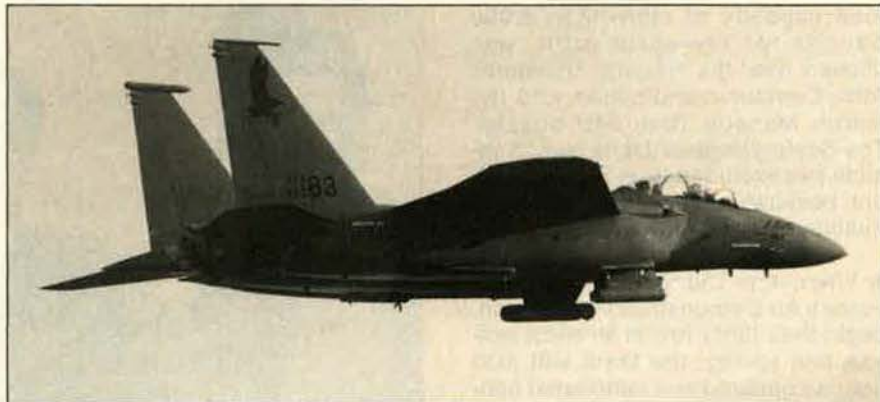
The first McDonnell Douglas F-15E dual-role fighter recently began its test program in earnest. But before the new Eagle left the factory in St. Louis, Mo., it was flown with Martin Marietta LANTIRN (Low-Altitude Navigation and Targeting Infrared for Night) pods and Dash-4 conformal fuel tanks with their low-drag, tangential stub weapons pylons.
