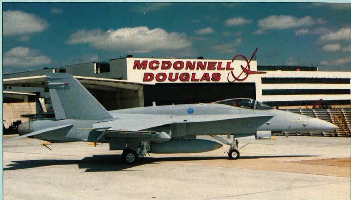
The antenna 'bumps' of the ASPJ distinguish this F/A-18C Hornet externally from the currently operational F/A-18A
