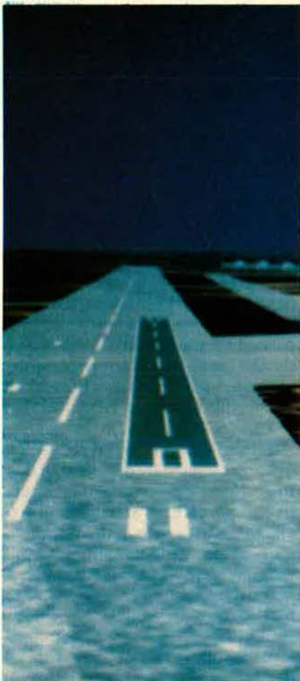
This computer-generated simulator image shows the specified area the SMTD F-15 must take off and land in—fifty feet wide by 1,500 feet long. The runway it's superimposed on is 200 feet by 8,000 feet.
