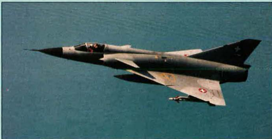
Swiss Air Force Mirage III-S evaluation aircraft, modified by F + W with nose strakes and fixed canards
