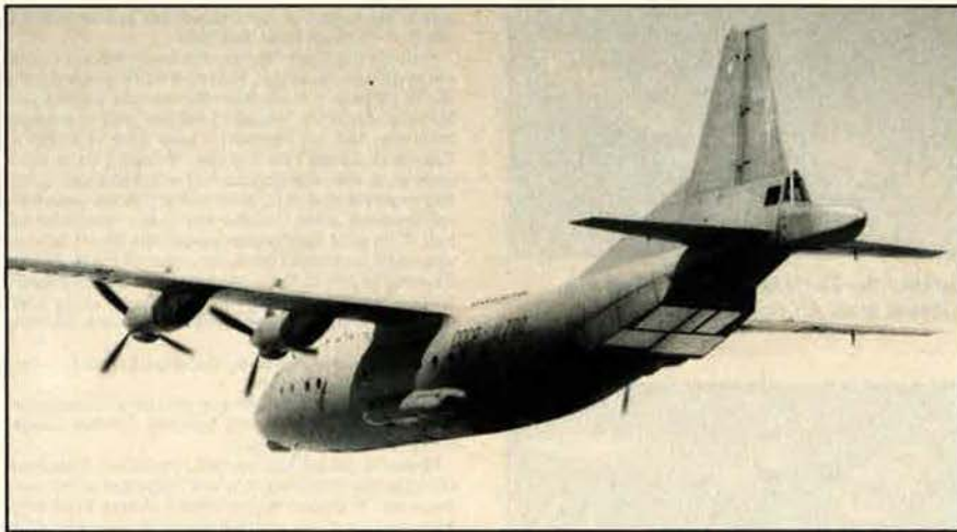
An-12 (NATO 'Cub') modified as test-bed for advanced avionics
