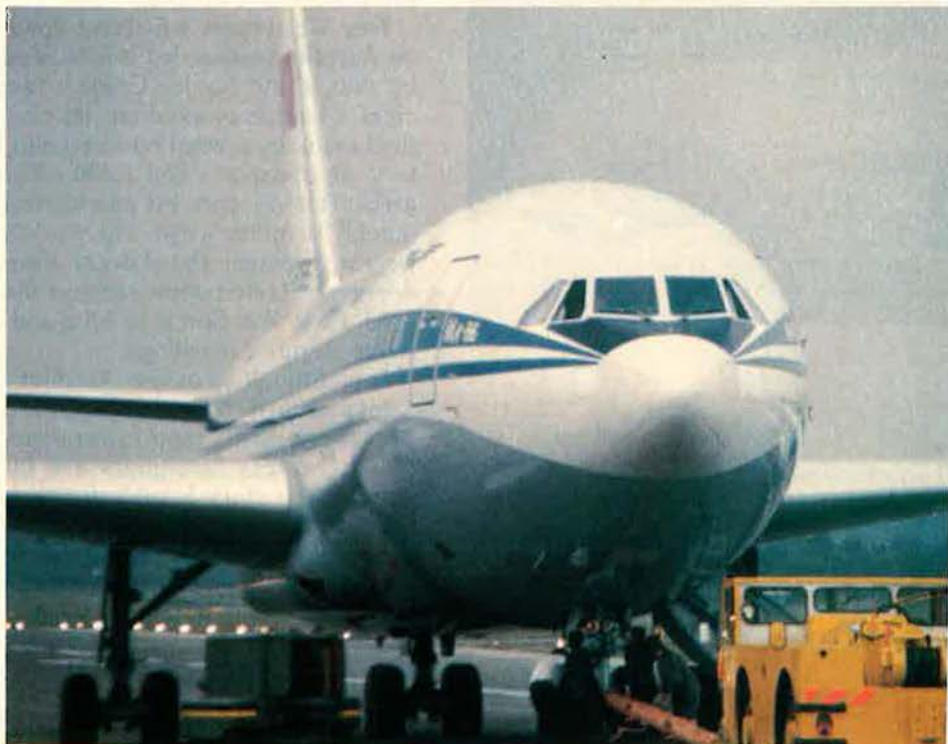
One of the mainstays of the Aeroflot fleet is the wide-body Il-86. It can carry up to 350 passengers, but the usual seating arrangement is for 234. With four turbofan engines, normal range is nearly 2,300 miles. (Photo by Norbert Neuser)
