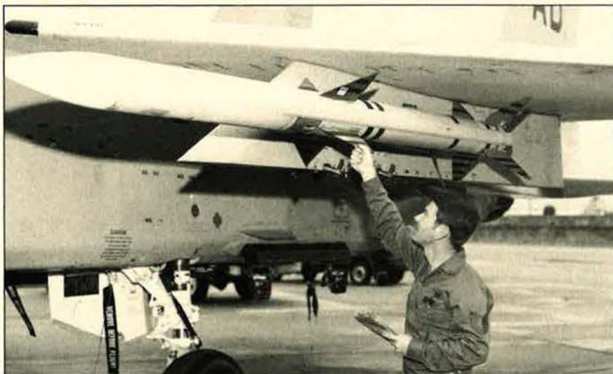
The AIM-120A Advanced Medium-Range Air-to-Air Missile (AMRAAM) test program is going smoothly, with a nearly ninety percent success rate. Here TSgt. Michael Stickle checks a fin on the missile prior to a test at Eglin AFB, Fla., last December.
