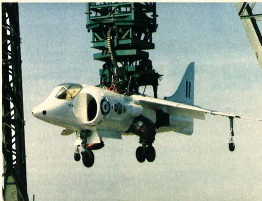
This captive Harrier airframe powered by a Rolls-Royce Pegasus engine with thrust augmentation is providing data that may ultimately lead to a supersonic vertical or short takeoff and landing aircraft.
