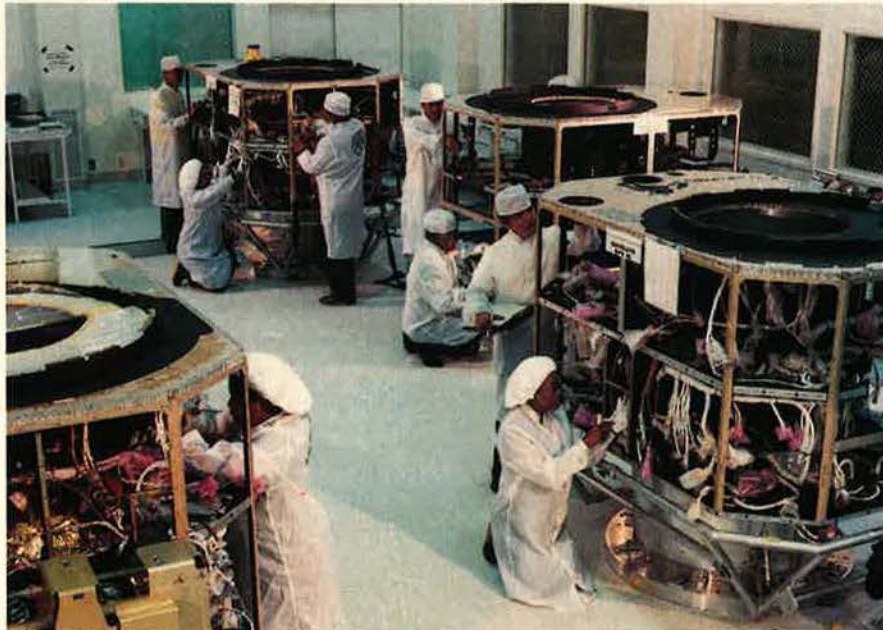
Rockwell workers assemble subsystems of Navstar Global Positioning System (GPS) satellites in the "clean room." Space Division will develop Medium Launch Vehicles (MLVs) for the express purpose of launching these vital navigation satellites.
