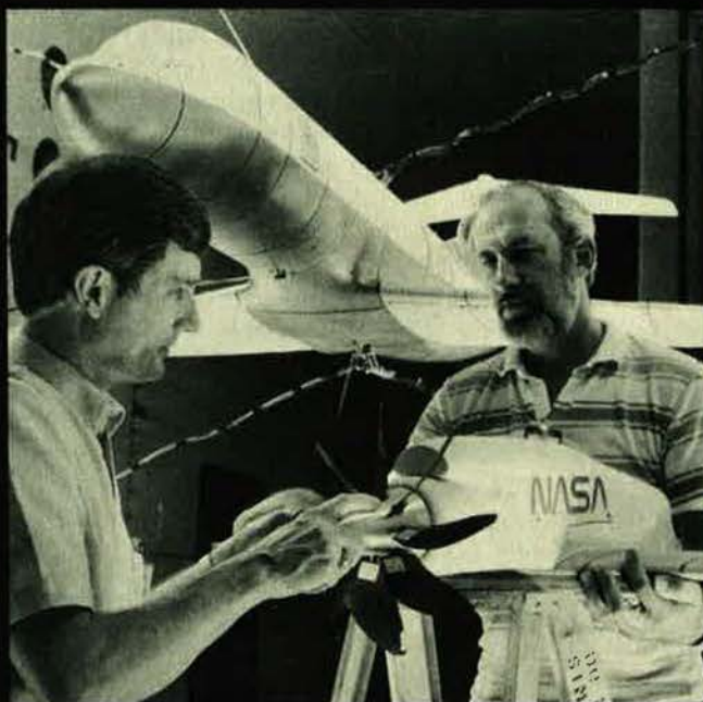
The latest revolution in propulsion may be a highly advanced throwback to the past—the propeller, or more specifically, the fuel-efficient propfan. This scale model was tested last year, and testing of the actual article will begin this month.
