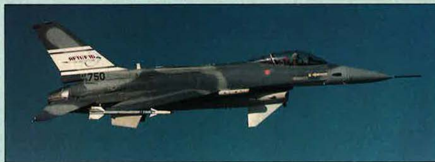
General Dynamics F-16/AFTI technology testbed aircraft, now with a Westinghouse FLIR sensor/tracker pod mounted at its starboard wingroot leading-edge
