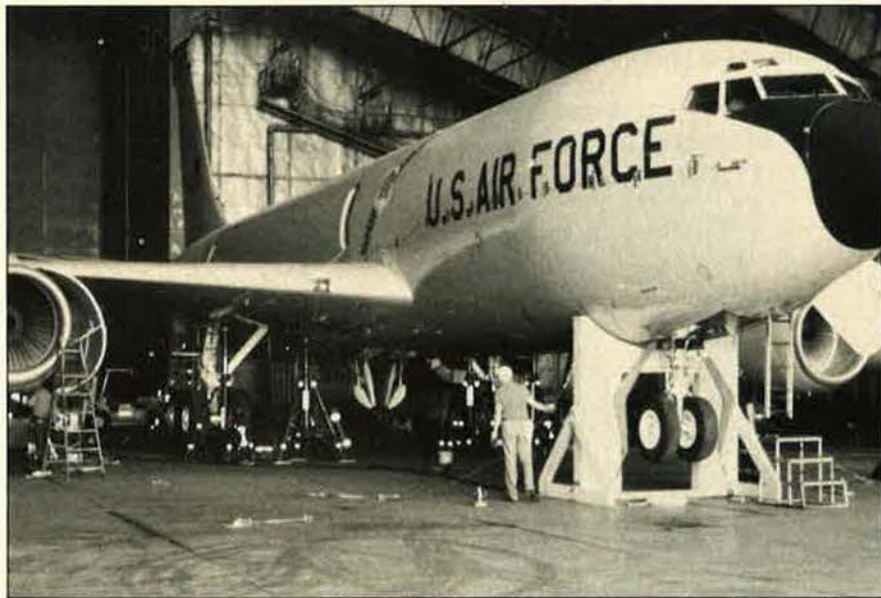
The latest model of the venerable Stratotanker—the KC-135R—recently completed a five-week test program in the McKinley Climatic Laboratory at Eglin AFB, Fla. The KC-135R's hydraulics, fuel system, CFM56 engines, and auxiliary power unit were tested in temperatures as low as -50^{\circ}\text{F} . No snow was involved in the tests.
