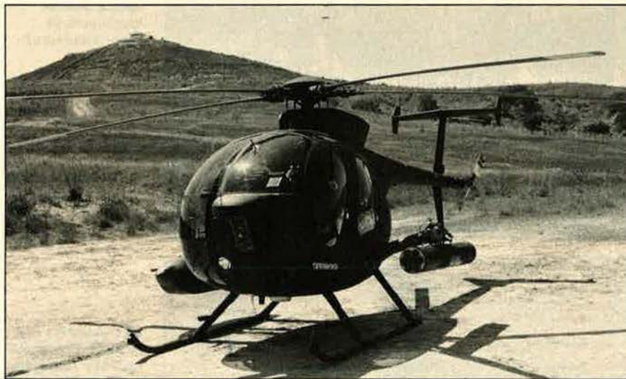
Lear Siegler Inc. recently qualified its Integrated Armament Management System (IAMS) on the McDonnell Douglas MD-530MG Defender. The IAMS provides integrated control of a variety of weapons. The Defender IAMS qualified with .50-caliber machine-gun pods, 7.62-mm twin machine-gun pods, and Mk 40 and Mk 66 2.75-inch folding-fin rockets.
