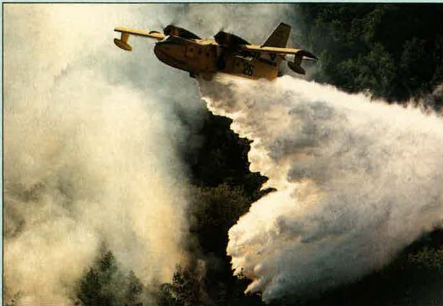
Standard piston engined Canadair CL-215 demonstrating its water bombing capability
