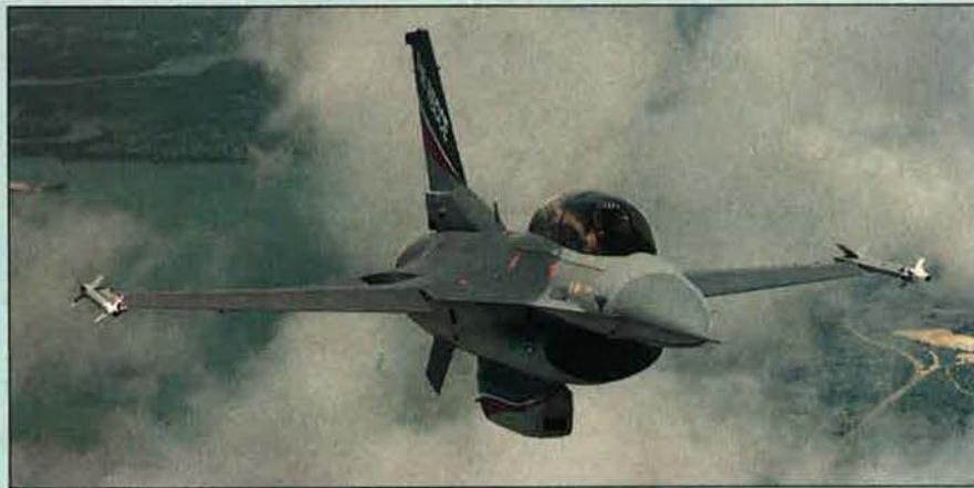
F-16R test aircraft equipped with General Dynamics reconnaissance pod
