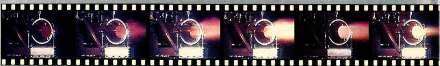
ATR firing demonstrating 10:1 turndown ratio
