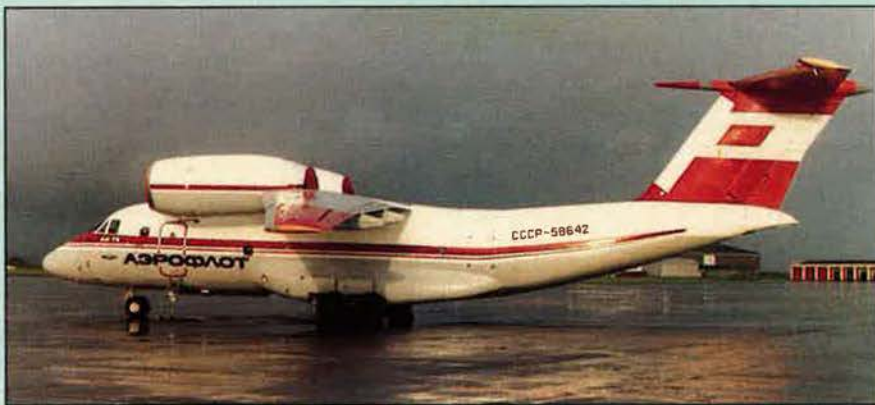
The lengthened fuselage of the Antonov An-74, compared with the An-72, is evident in this view (Paul R. Duffy)
