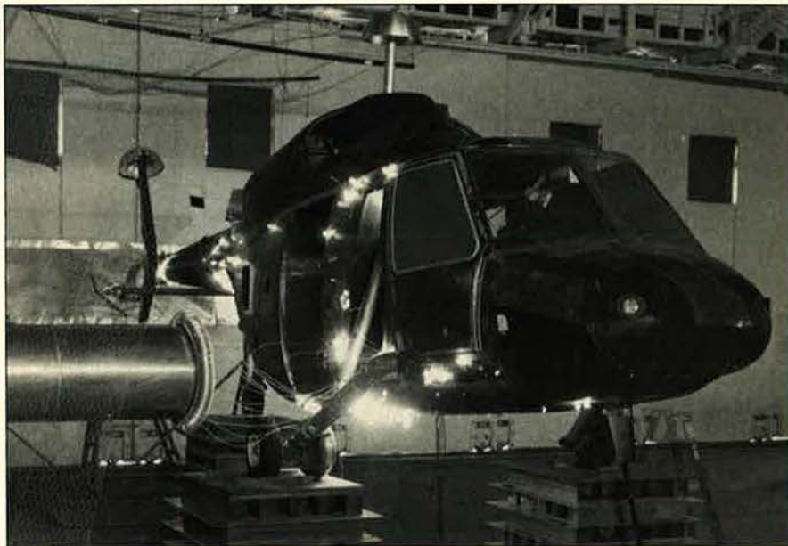
Nature's most extreme forms of weather are being simulated to help the Air Force in its ongoing battle with the elements. Here a Bell D292 helicopter is subjected to 1,600,000 volts of electricity at Boeing Military Aircraft's plant in Seattle, Wash., in order to develop guidelines for better lightning protection.
