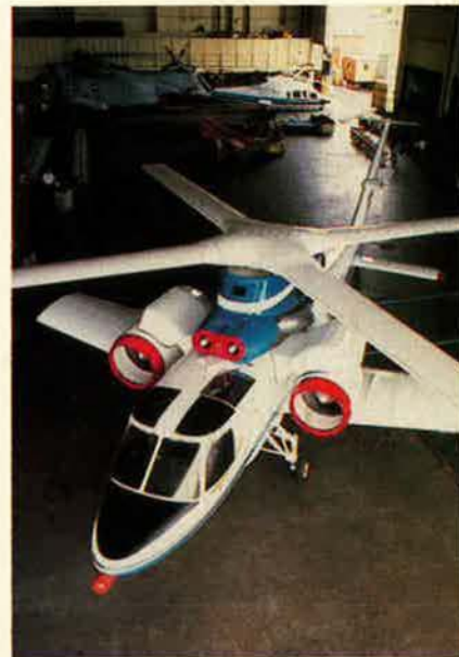
Speeds from hover to 300 knots are expected from the Sikorsky S-72 X-wing demonstrator.
