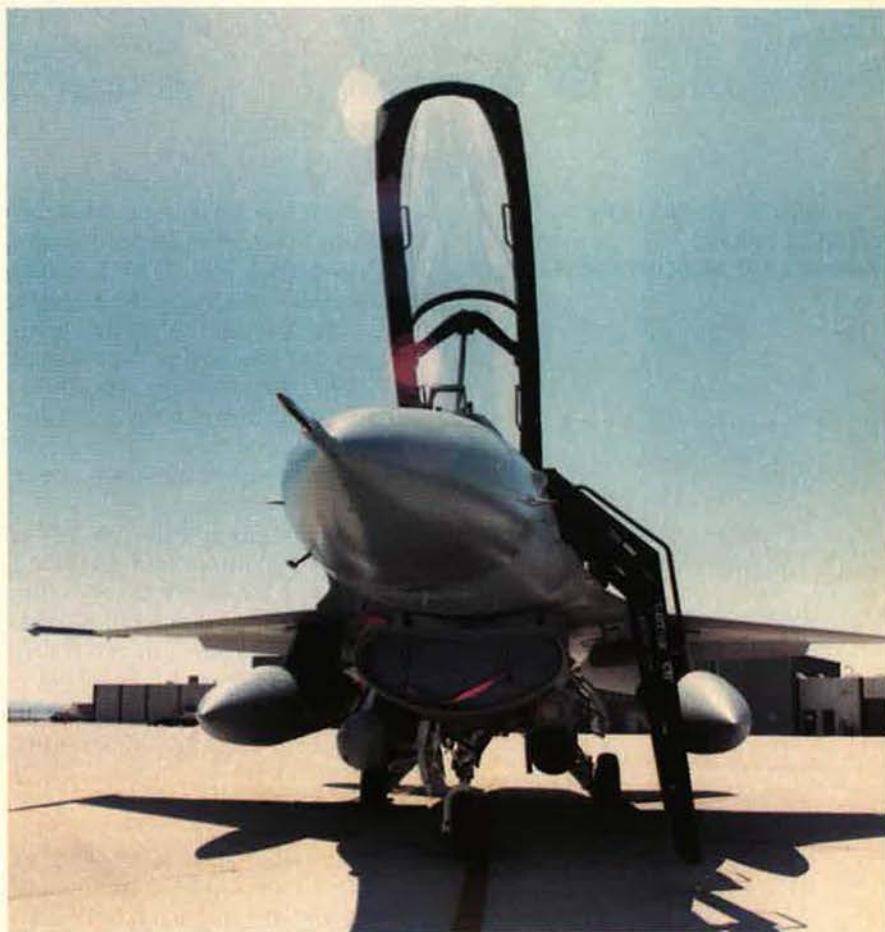
LANTIRN navigation and targeting pods mounted underneath the fuselage of an F-16. LANTIRN will have a "radical impact" on USAF's ability to wage conventional warfare and will be deployed initially on F-15E dual-role fighters about two years from now.
