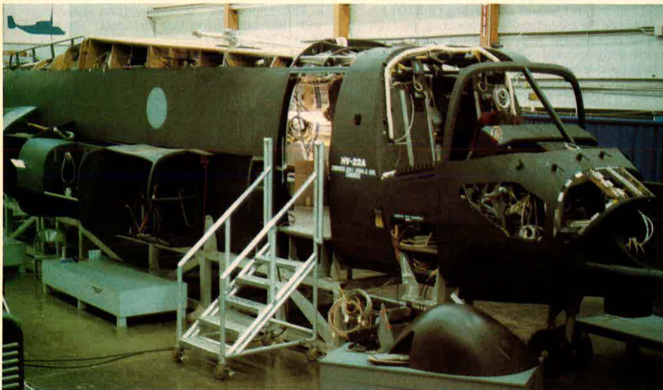
Full-scale mockups have been built to check the fit and function of the various subsystems. The weight growth that creeps into any new aircraft is being carefully watched and kept in check through the wide use of composite materials in the Osprey.
