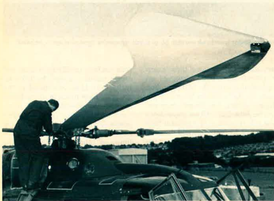
Westland's BERP III rotor, which made possible the new world's absolute speed record for helicopters.
