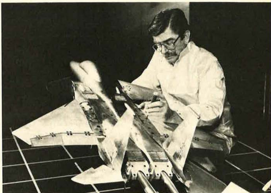
A McDonnell Douglas technician adjusts the wind-tunnel model of the F-15 short-takeoff-and-landing (STOL) and maneuvering demonstrator aircraft being developed by the company for ASD. It is scheduled to begin test flights in early 1988.
