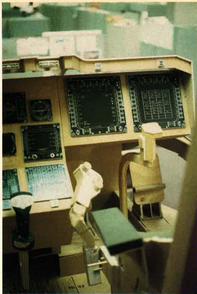
Prominent features in the CV-22's cardboard cockpit mockup include two color MFDs that show engine or flight instrumentation and, on the left, the sensor track handle for crew FLIR control.
