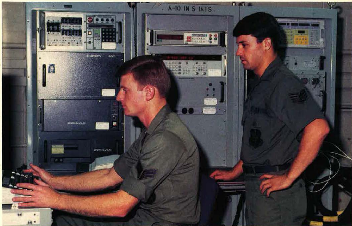
Maintenance technicians SrA. Floyd R. Studt (left) and SSgt. John R. Tushner of England AFB’s 23d Tactical Fighter Wing use some of the first delivered Modular Automatic Test Equipment (MATE) to test the INS for the A-10.
