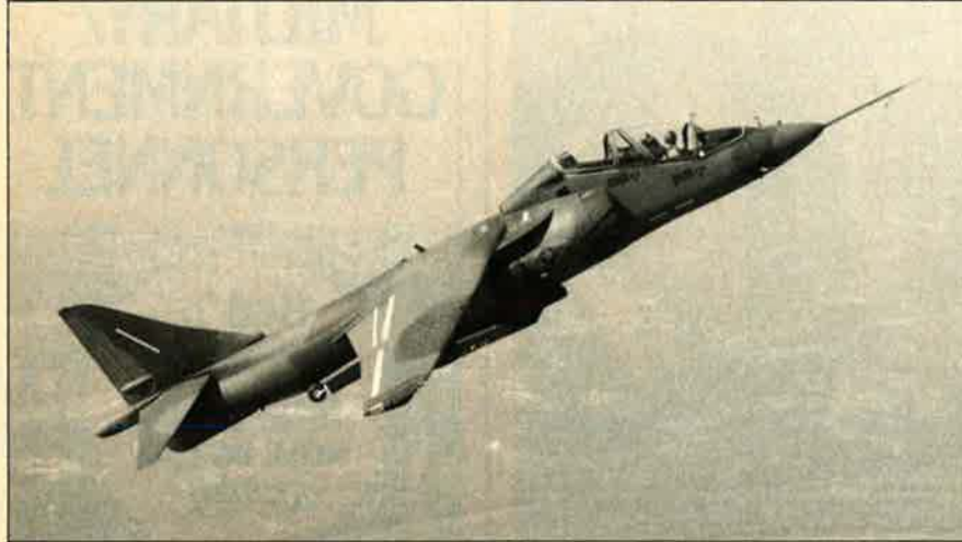
This two-seat version of the Harrier, the TAV-8B, will be used by the Marine Corps to train its pilots in vertical and short takeoff and landing.
