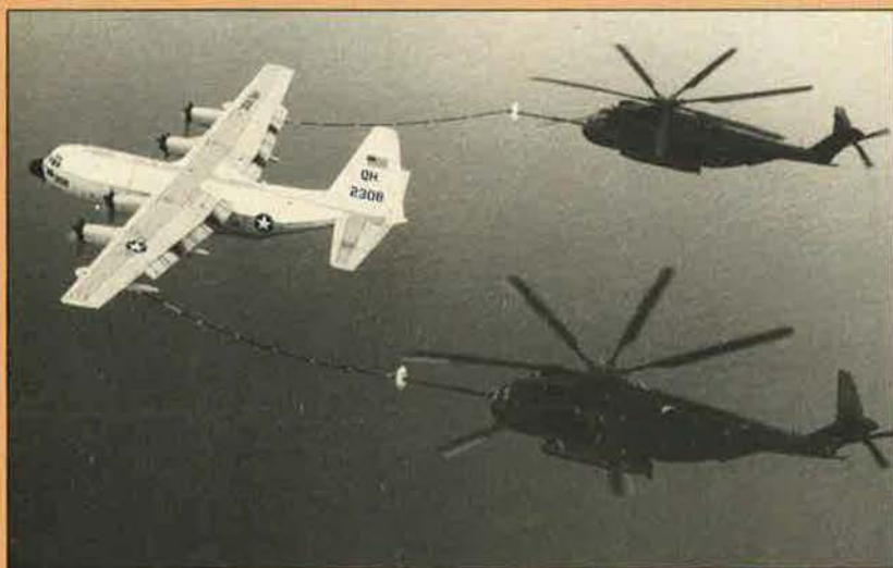
The US Marine Corps uses a tanker version of the C-130, the KC-130T, to refuel two of the world's largest helicopters simultaneously. The two Sikorsky CH-53E "Super Stallion" birds are drawing fuel from a 3,600-gallon refueling tank that could be easily removed from the propjet tanker to convert it back into a transport for cargo or troops.
