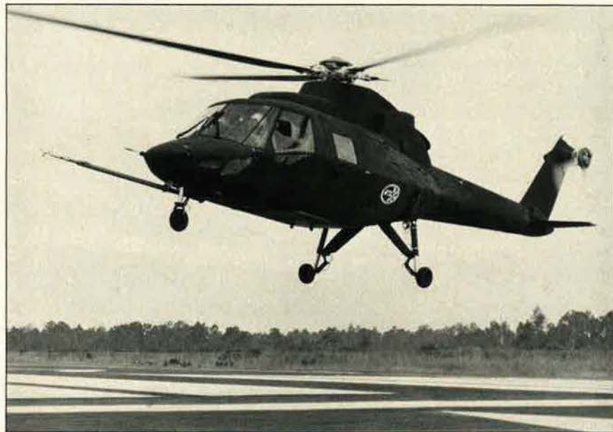
The US Army/Sikorsky Advanced Composite Airframe Program (ACAP) helicopter made its first flight recently. The ACAP, the world's first composite-fuselage helicopter, is a revolutionary departure from aluminum helicopter airframes. (See item, p. 37.)
