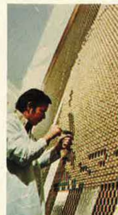
Phased array elements form the antenna of this radar for range instrumentation.
