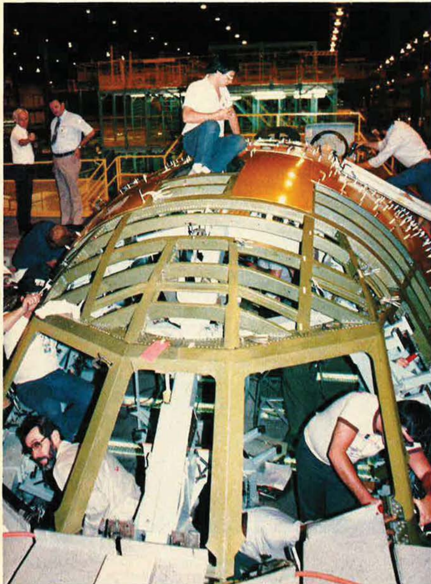
Lockheed-Georgia assemblymen prepare the forward fuselage cab top for the first of fifty new C-5B military transports. Air Force officials are relying on the C-5B and the C-17 to help meet future wartime airlift requirements. The first C-5B is scheduled for delivery in December '85.
