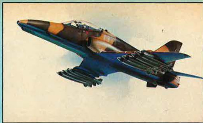
Hawk 200 equipped for night operation with FLIR and laser rangefinder
