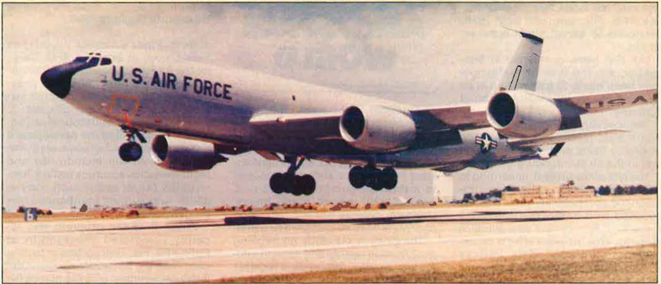
The first KC-135R tanker reequipped with CFM56 engines takes off after being delivered to USAF by Boeing in July. It'll be based at McConnell AFB, Kan., as part of SAC's 384th Air Refueling Wing.
