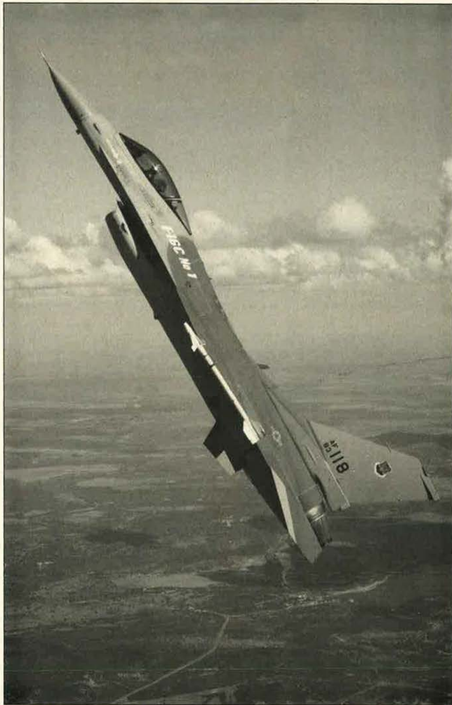
USAF's first F-16C took flight following delivery at General Dynamics Corp.'s Fort Worth, Tex., plant last July. Unlike earlier variants, which can carry only short-range, heat-seeking Sidewinders, the F-16Cs are wired for radar-guided advanced medium-range air-to-air missiles and thus will be more potent in the air-superiority mode.
