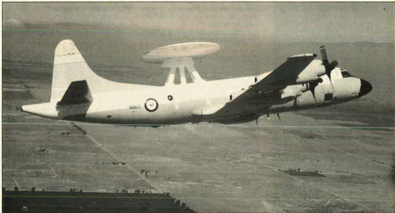
Featuring a saucer-shaped rotodome designed to house the antenna for a General Electric APS 138 radar, this specially modified P-3 Orion has begun test flights at Lockheed-California Co.'s flight-test center in Palmdale, Calif. See item.
