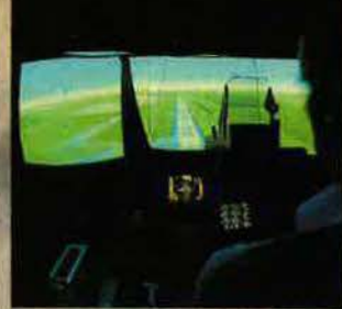
CGIVS. Computer-generated image visual system for the Tornado training simulator.
