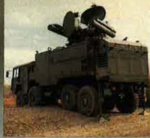
ROLAND. Guided missile system mounted on a shelter for use against low-flying aircraft.
