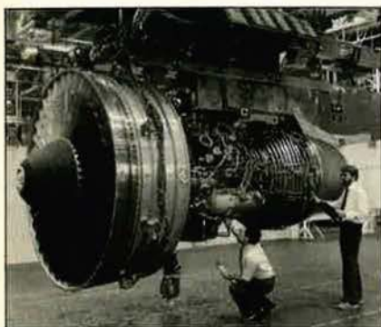
Designed as the most fuel-efficient, high-thrust engine ever, Pratt & Whitney's new-technology PW4000 aircraft engine already has reached its predicted levels of performance during recent tests. Top output of 61,800 pounds of thrust was achieved.
