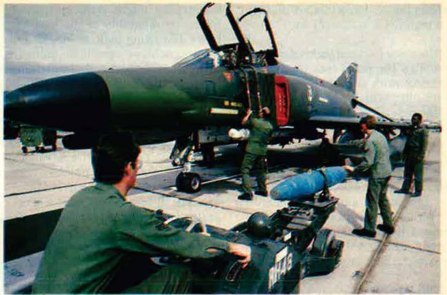
Members of the 69th Aircraft Maintenance Unit and the 347th Aircraft Generation Squadron from Moody AFB, Ga., prepare to upload Mk 82 low-drag inert bombs on an F-4E during Red Flag at Nellis AFB, Nev. The Phantom is still the most prevalent fighter in the TAF force structure. (Photo by William A. Ford, Art Director)
