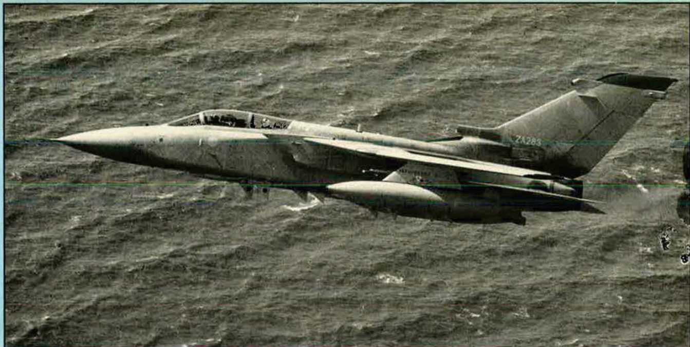
A longer fuselage gives the Tornado ADV a more attractive appearance than its stubby Tornado GR. Mk 1 interdictor/strike predecessor
