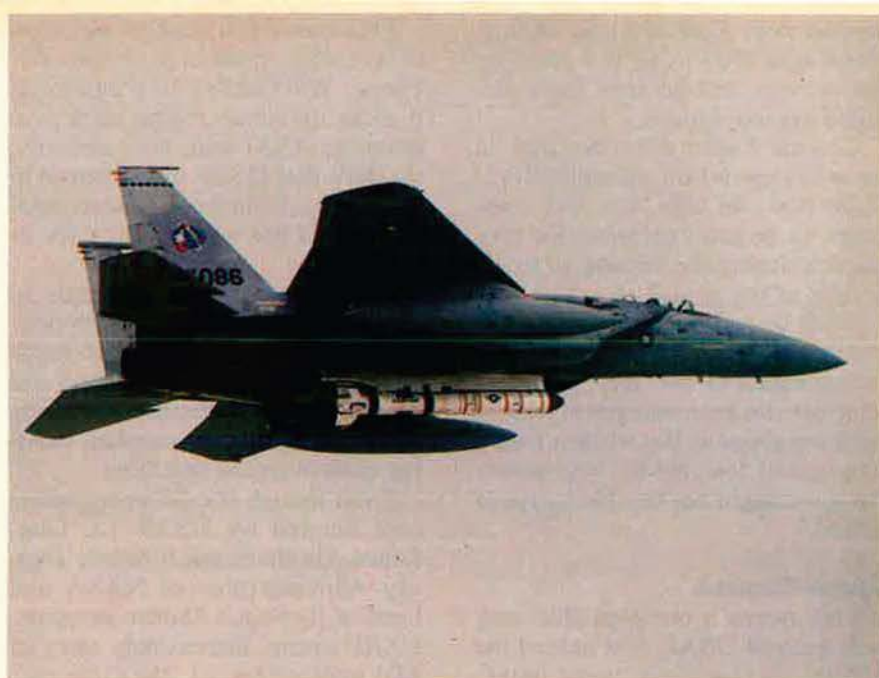
USAF's antisatellite (ASAT) weapon, shown here in an F-15 centerline captive-carry test, is crucial to the execution of the "space control" mission delineated in the US Air Force Space Plan. The TAV would benefit that plan's "force application" mission.
