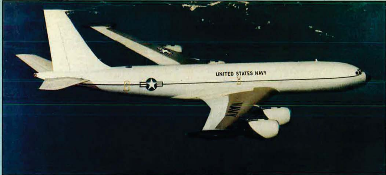
Retouched photograph of Boeing E-3/AWACS airframe with CFM56 engines, in E-6 TACAMO configuration
