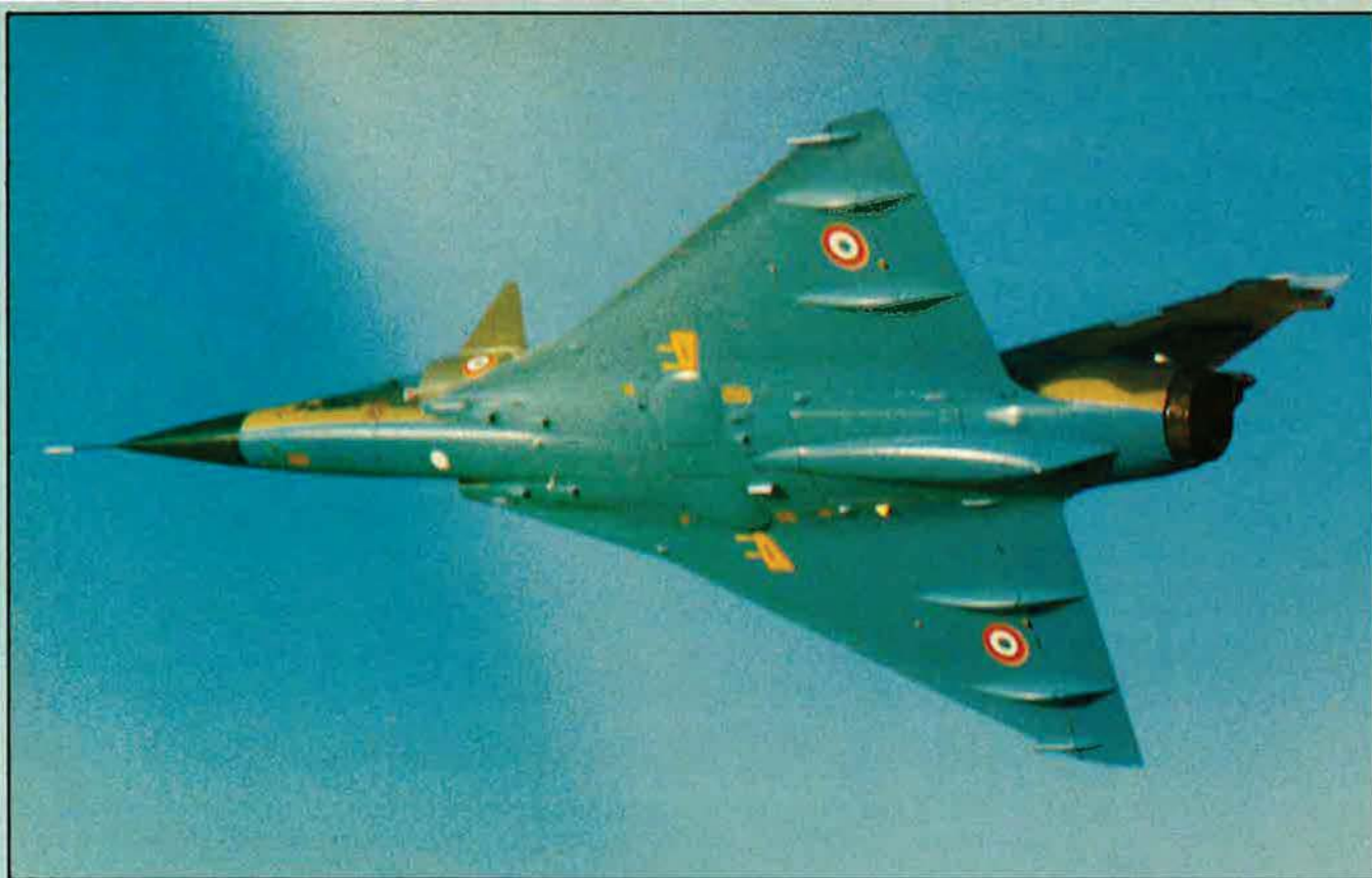
Foreplanes and wing leading-edge extensions of the Mirage 3 NG are shown clearly in this view
