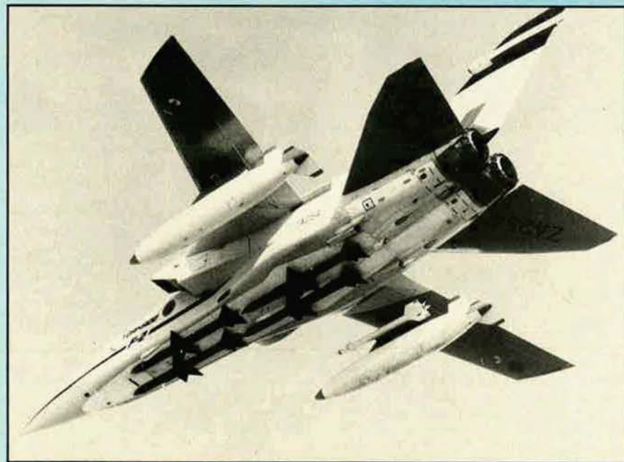
Four underfuselage Sky Flash missiles, plus a Sidewinder and auxiliary fuel tank under each wing, is standard combat air patrol configuration for the Tornado ADV
