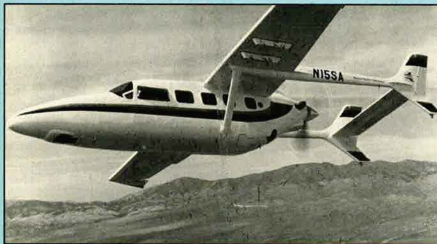
Spectrum-One, a turboprop development of the Cessna 337 Super Skymaster
