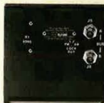
MIL-STD-1553 front-panel module allows direct interface with aircraft digital bus systems.
