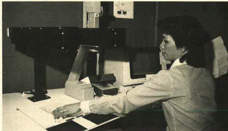
Kathy Salas of AFAFC's Directorate of Retired Pay, Lowry AFB, Colo., operates a Ragan machine. It photographs all incoming documents for computer storage.
