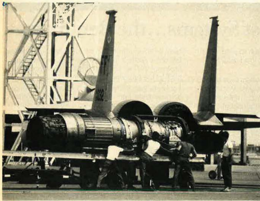
A USAF F-15 undergoes an engine change during the Arid Farmer deployment of F-15, KC-10, and E-3A aircraft to Khartoum in the Sudan last August. The deployment was in response to Libyan aggression against Chad.
