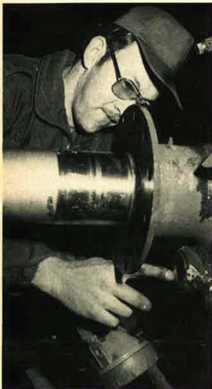
SSgt. Ricky Harmon of the 22d Field Maintenance Squadron, March AFB, Calif., inspects a main landing gear axle on a KC-135 tanker.
