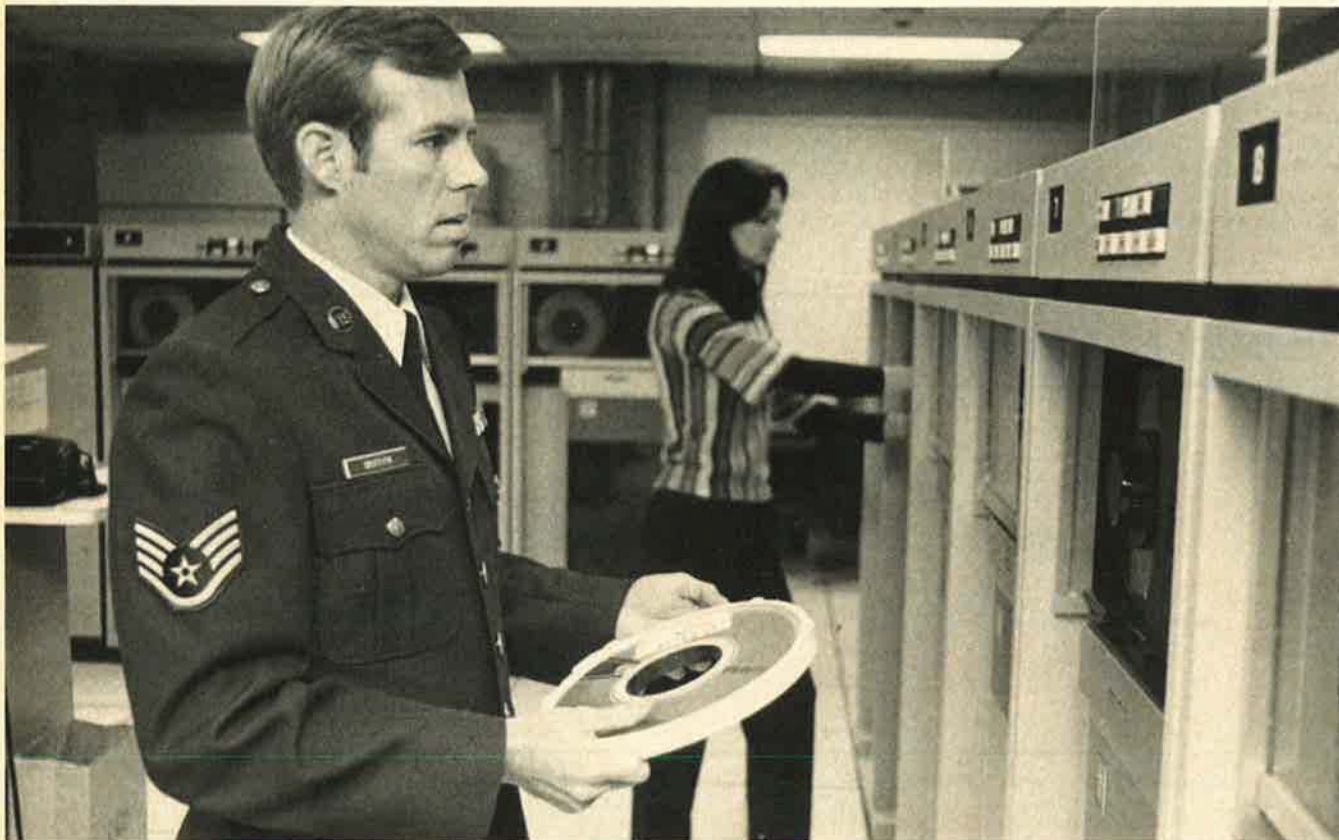
SSgt. Stanley M. Griffith prepares to install a tape in a Sperry 1100/80 computer, the newest computer system at Electronic Security Command (ESC) headquarters, Kelly AFB, Tex. The computer has sixteen tape drives for data recording.
