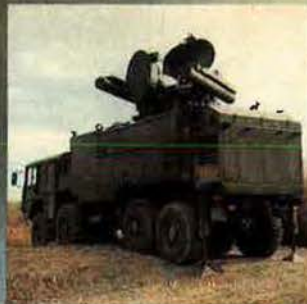
ROLAND. Guided missile system mounted on a shelter for use against low-flying aircraft.
