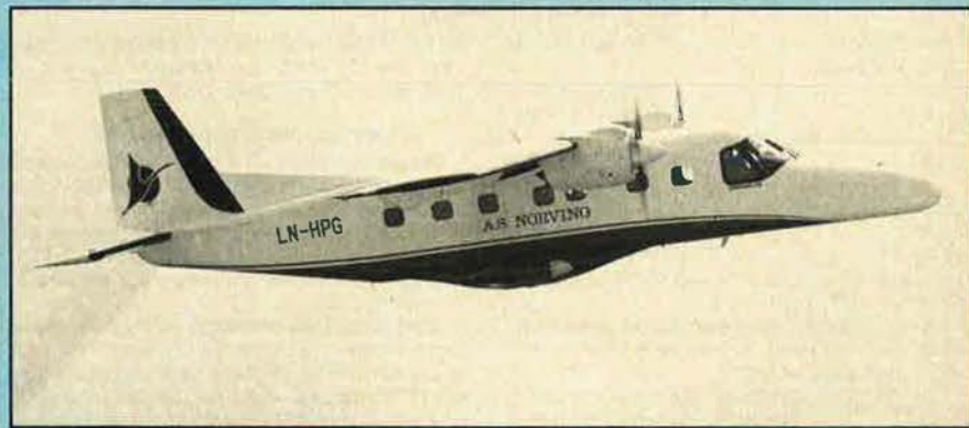
Dornier 228-100 twin-turboprop 15-passenger light transport
