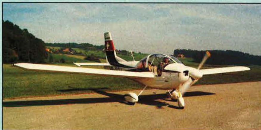
This ground shot of the Dätwyler MD-3-160 shows well the superb field of view from the side by side cockpit
