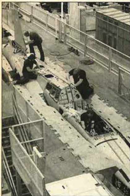
Northrop Corp.'s third F-20 Tigershark recently passed a stringent Air Force inspection of the center and aft fuselage sections without a single defect. The third Tigershark is being completed at the company's Production Development Center in Hawthorne, Calif., where the entire fuselage was recently mated on schedule. See item.
