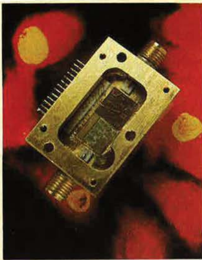
By applying technologies for large-scale integrated circuits, Rome Air Development Center has pioneered the Monolithic Microwave Integrated Circuits (MMIC) in this module.
