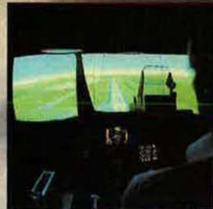
CGIVS. Computer-generated image visual system for the Tornado training simulator.
