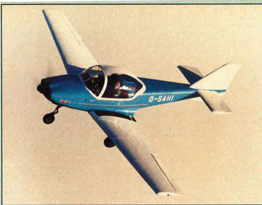
Trago Mills SAH-1 two-seat fully aerobatic light aircraft (Avco Lycoming O-235-L2A engine)
