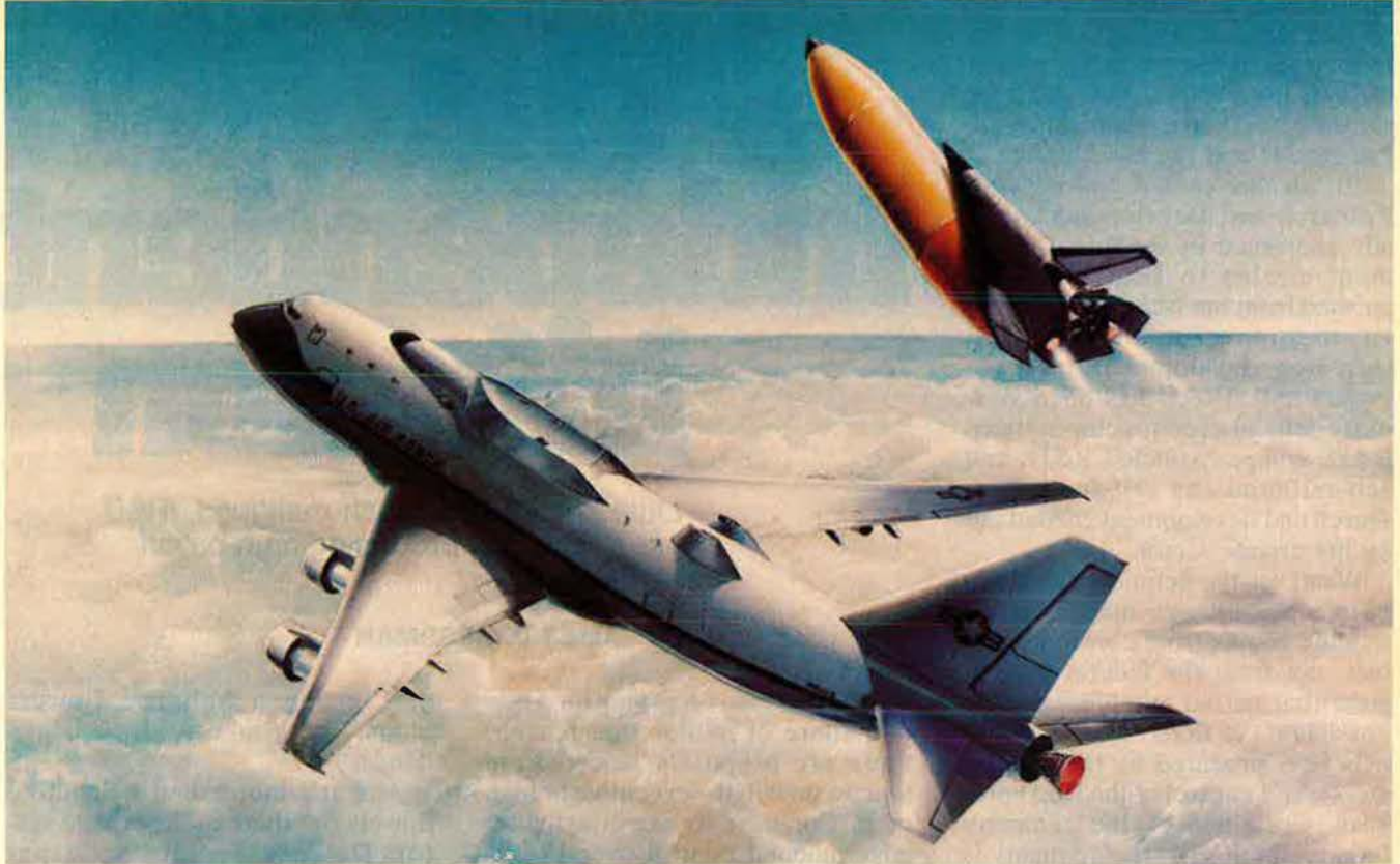
Under a USAF study contract, Boeing developed the concept of an air-launched space sortie vehicle shown here. Several companies are now joining with USAF to devise a horizontal-takeoff, multimission, manned Transatmospheric Vehicle (TAV).
