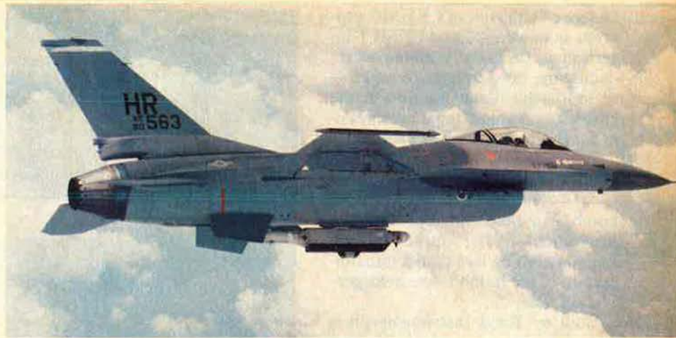
USAF's AN/ALQ-131 airborne jamming pod, here aboard an F-16, will be the first operational military system to incorporate VHSIC-based signal processors.
