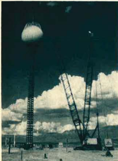
Sphere containing enough high explosives to simulate a one-kiloton nuclear blast awaits detonation at White Sands Missile Range, N. M., in a test of effects on small-ICBM model transporter/launcher vehicles.
