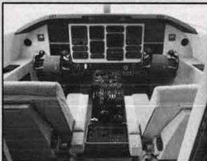
Flight deck of the Starship 1, with the multi-CRT panel specified for many next-generation business transports
