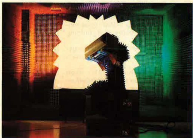
Testing phased array in compact antenna range.
