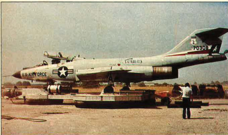
The Air Force has successfully tested the Air Cushion Equipment Transportation System designed to move aircraft—on ducted air—over rough terrain or damaged taxiways or runways. The platform was designed and built under a joint US/Canadian program. See adjacent item.
