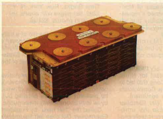
Modular packaging of array electronics.
