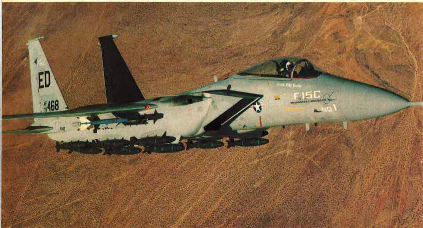
Over Edwards AFB, an F-15C sports its new "tangential carriage" of air-to-ground ordnance. Placing bombs front-to-rear on conformal fuel tank pylons increases the range and greatly cuts the drag of the aircraft, McDonnell Douglas claims.
