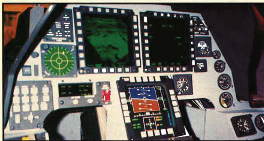
Rear cockpit mockup of F-16XL dual role fighter candidate highlights three five-inch-square multifunction displays. On the top two screens, the F-16XL weapon system officer (WSO) can display and control video and descriptive text from radar, FLIR, and other sensors as well as stores management, navigation, and other functional information. The lower color multifunction display can show Color Moving Map with superimposed navigation data, color-coded flight information (top photo), and color-coded external configuration information (bottom photo). Complete sets of hands-on system controls, backup flight instruments, integrated left-hand operated communication, navigation, and identification controls and displays, along with a selectable flight-control capability, round out the WSO's cockpit capabilities. (Air Force Magazine photos)
