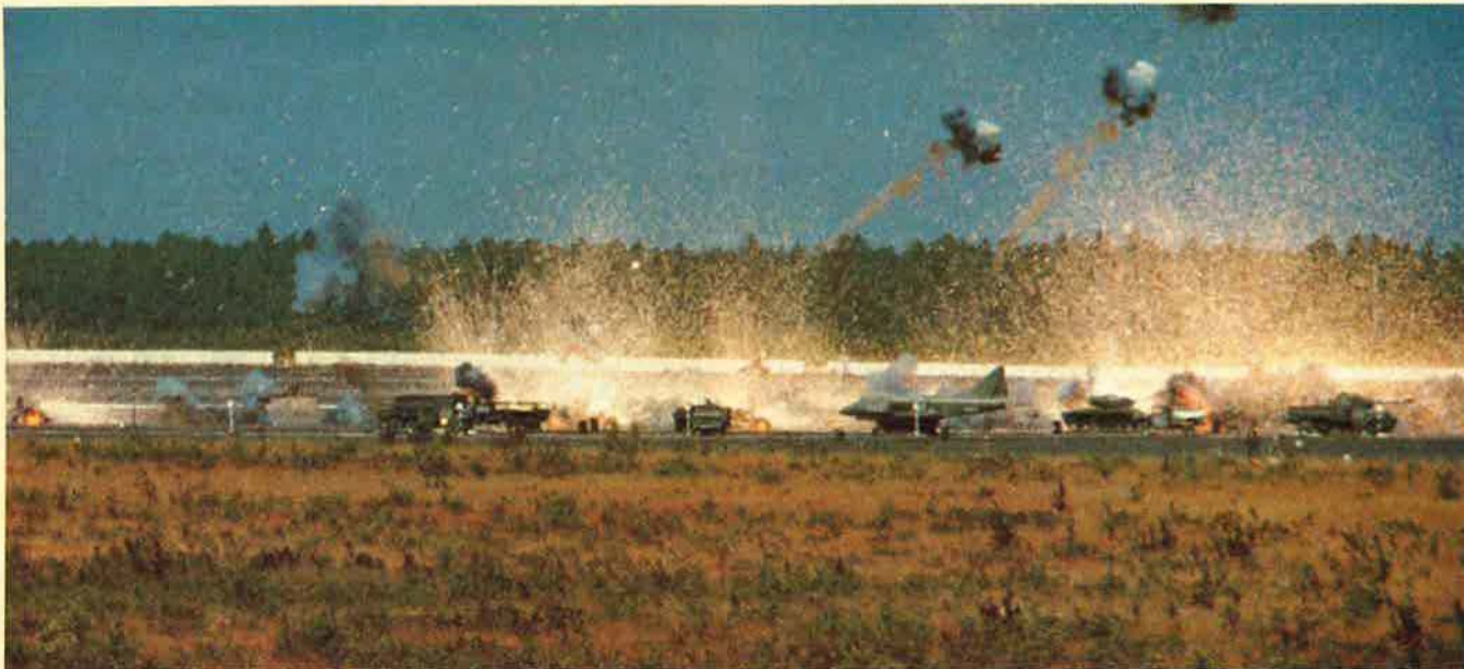
The Combined Effects Munition consists of three types of specialized bomblets to cover a wide spectrum of mobile targets, ranging from personnel to armor. The individual bomblets are equipped with small inflatable sleeves to provide stabilization.
