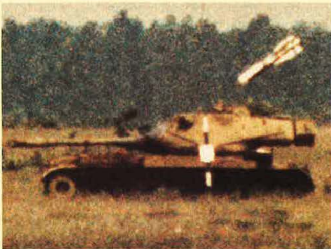
The Wasp minimissile uses millimeter wave guidance that enables the weapon to operate in adverse weather and fog. This "smart" missile has a reliable standoff capability.
