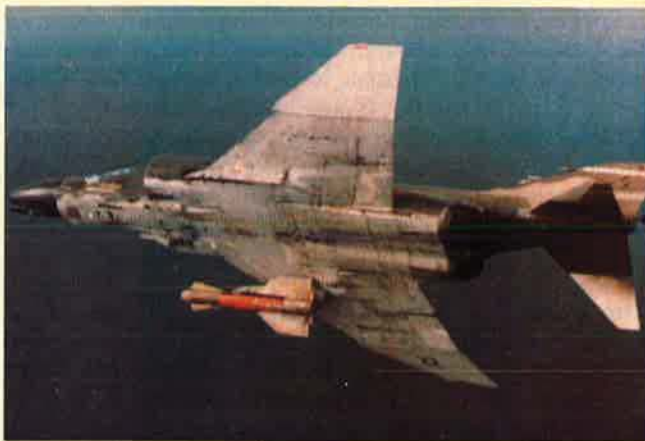
The GBU-15 Modular Guided Weapon will be given greater range when a rocket motor is added. The new version will be equipped with terrain-avoidance features and an altimeter.
