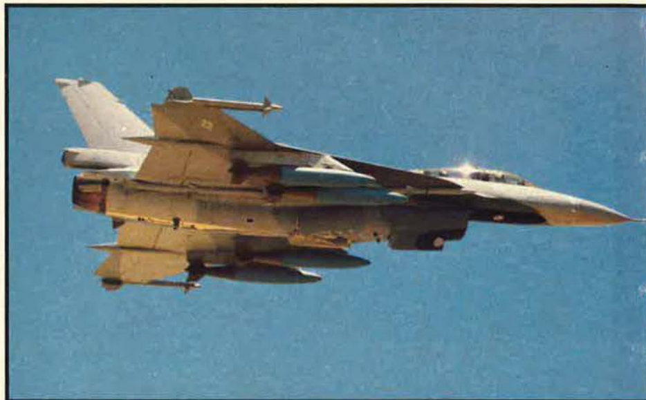
The two-seat version of the F-16XL carrying four Mk 84 2,000-pound training bombs, two AIM-9 Sidewinders, and four AMRAAM missiles.
