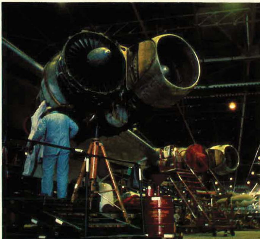
Programmed depot maintenance, seen here on a B-52, can include everything from stripping and painting to engine overhaul.
