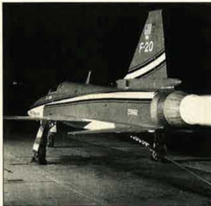
Northrop Corp.'s Mach-2 class F-20 Tigershark demonstrates the power of its 17,000-pound-thrust GE F404 low bypass turbofan engine. The nighttime test took place recently at Edwards AFB, Calif., where the aircraft is being developed with company funds.
