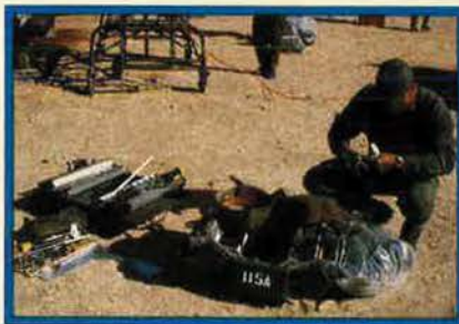
Rapid battle damage repair, above, is a concept pioneered by AFLC that has spread to USAFE. Major components are repair kits containing the required tools and matériel, left.
