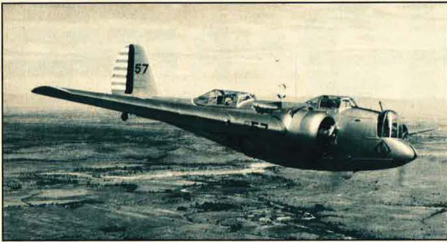
The Martin B-10 was the first modern bomber, with enclosed cockpit and retractable landing gear. It was nearly as fast as pursuits of its day, but was too small for the long-range offensive missions Air Corps strategists foresaw.
