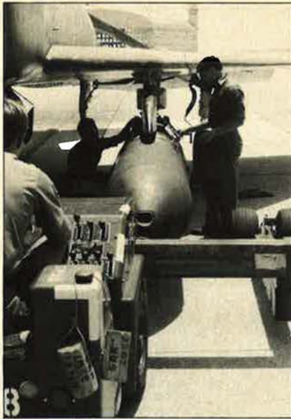
Designed to destroy enemy armor, a GPU-5/A Gun Pod is mounted on an F-4 Phantom at Moody AFB, Ga. The pod gives tactical aircraft other than the A-10 tank-killing capability.
