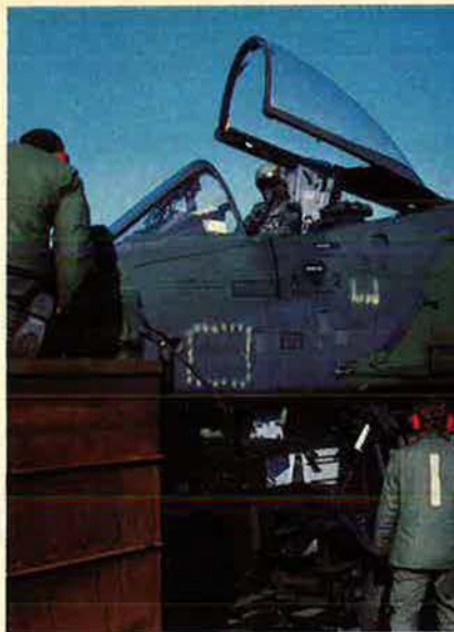
During a combat quick turn at RAF Bentwaters, two munitions specialists use the Automatic Loading System to arm an A-10's GAU-8 Gatling gun with 30-mm ammunition.
