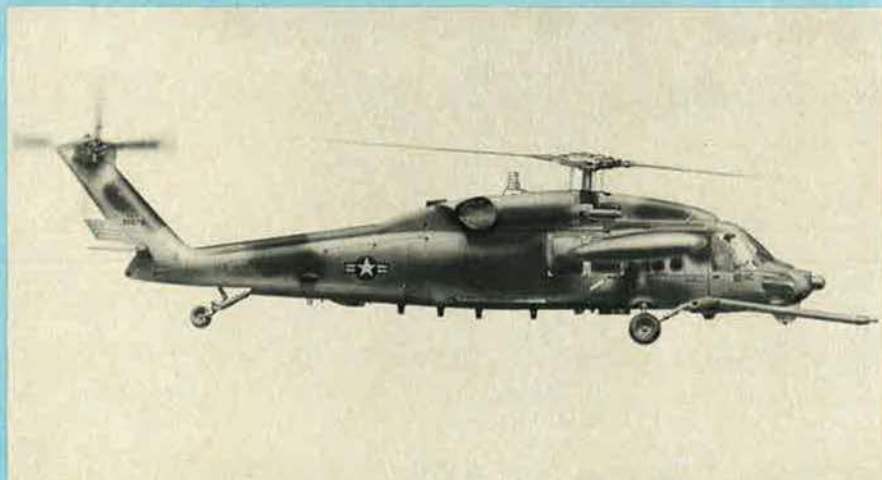
Features of the HH-60D Night Hawk, including the retractable flight refuelling probe, external fuel tanks, nose radar, and other avionics, are shown in this drawing
