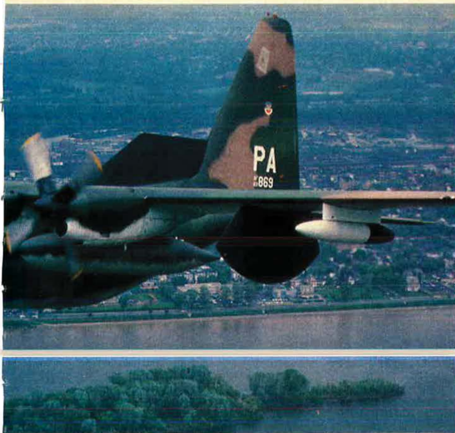
The EC-130H Compass Call aircraft is the heavyweight of the tactical jamming arena. Developed as a quick reaction project, it is constantly being improved, both in hardware and tactics.
