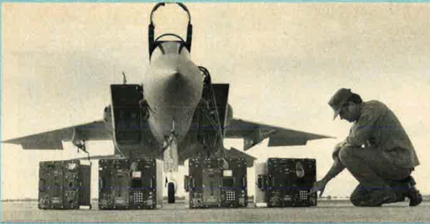
The AN/APM-427 Improved Radar Simulator can be used on the flight line.
