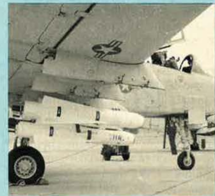
AGM-65D IR Maverick extends ground-attack capabilities into low light and adverse weather.
