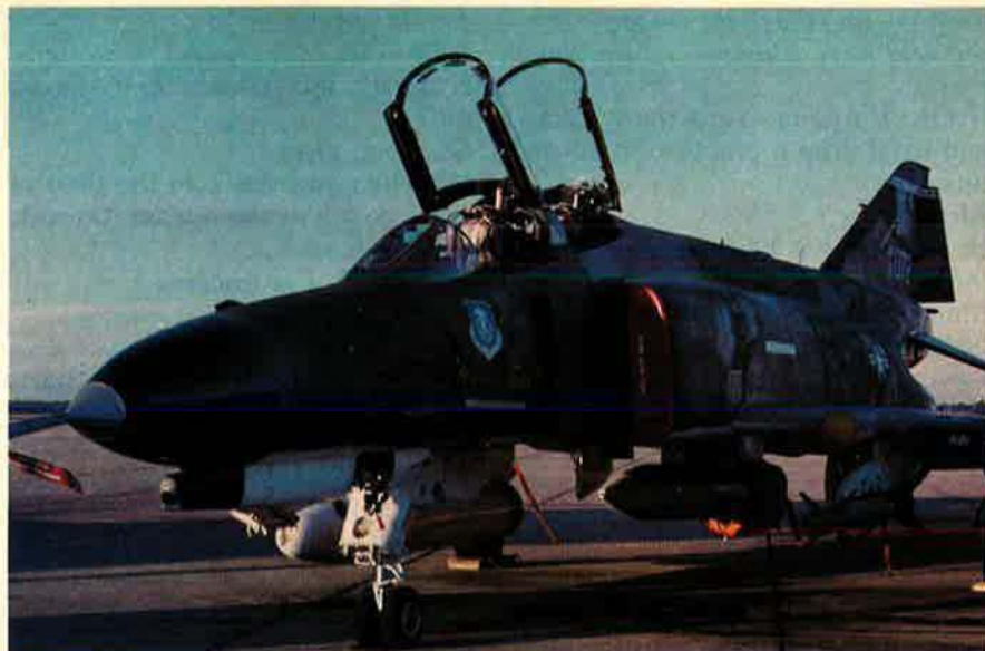
ABOVE: Air Force Systems Command F-4E with Pave Tack pod on centerline. The TISEO (Target Identification System, Electro-Optical) "eye" can be seen on the left wing's leading edge (yellow circle). LEFT: Closeup of Pave Tack pod on F-4E in flight. (AIR FORCE Magazine photo)
