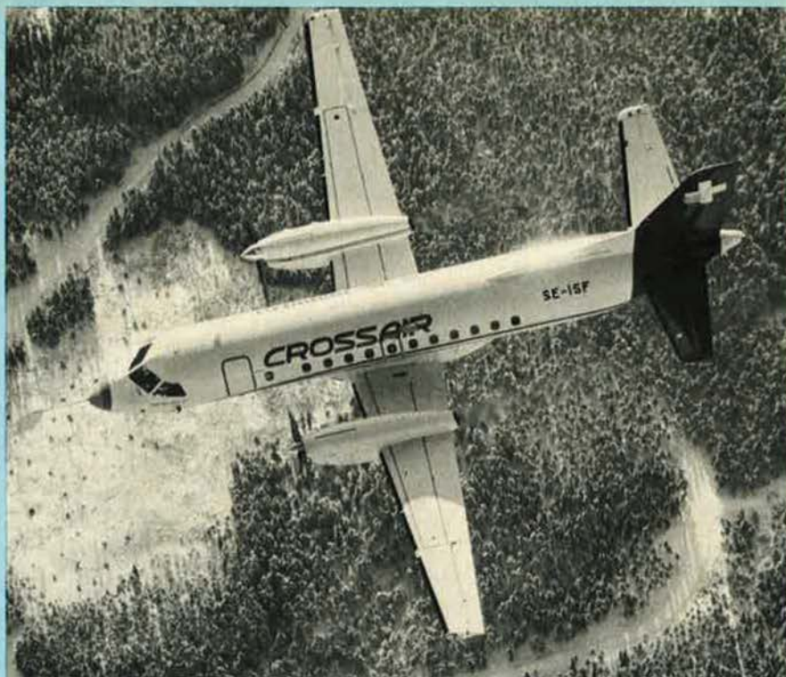
Prototype of the Saab-Fairchild 340, with test boom on nose
