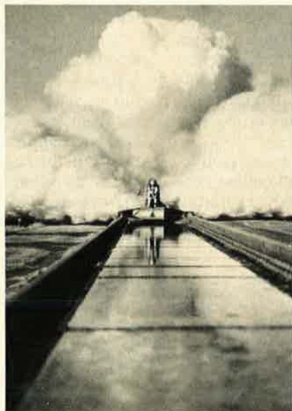
Stapp hits the water brake at the end of a 632-mph rocket sled run.
