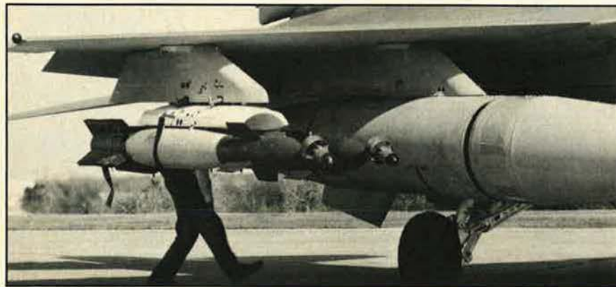
This F-16 was recently used for flight tests of a low-drag, dual-store bomb-release system designed by Alkan/Texas Instruments. Being considered for acquisition by the French Air Force and other services, the Alkan system permits near-vertical release to reduce weapon dispersion and is readily adaptable to a variety of aircraft.
