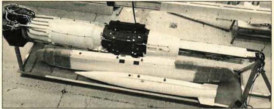
A full-scale functional mockup of Grumman Aerospace Corp.'s entry in the competition for a Common Strategic Rotary Launcher for SAC aircraft. It is unique in having a fixed composite material center beam and in that no pyrotechnics are used in the ejection of missiles from the aircraft's bomb bay. Instead, the device relies on a single proprietary hydraulic system designed for the purpose. The launcher is capable of carrying a full complement of five base-line weapons and prospective growth weapons in the bomb bays of the B-52H, B-1B, and forthcoming Advanced Technology Bomber (ATB). The five weapons include several types of gravity bombs, SRAM, and ALCM-B.
