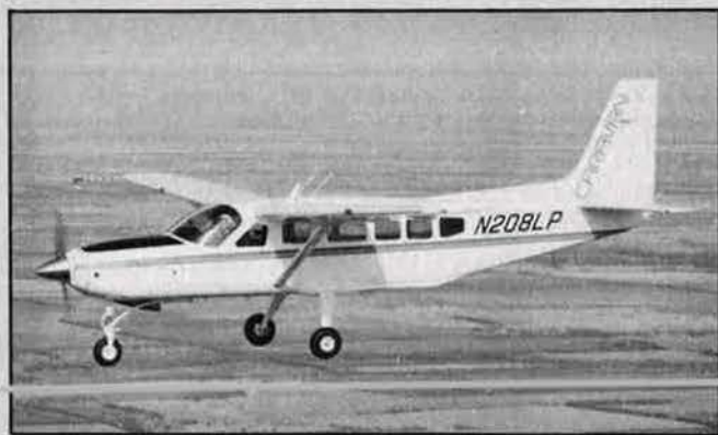
Prototype of the all-new 14-passenger Caravan utility aircraft, first flown last December
