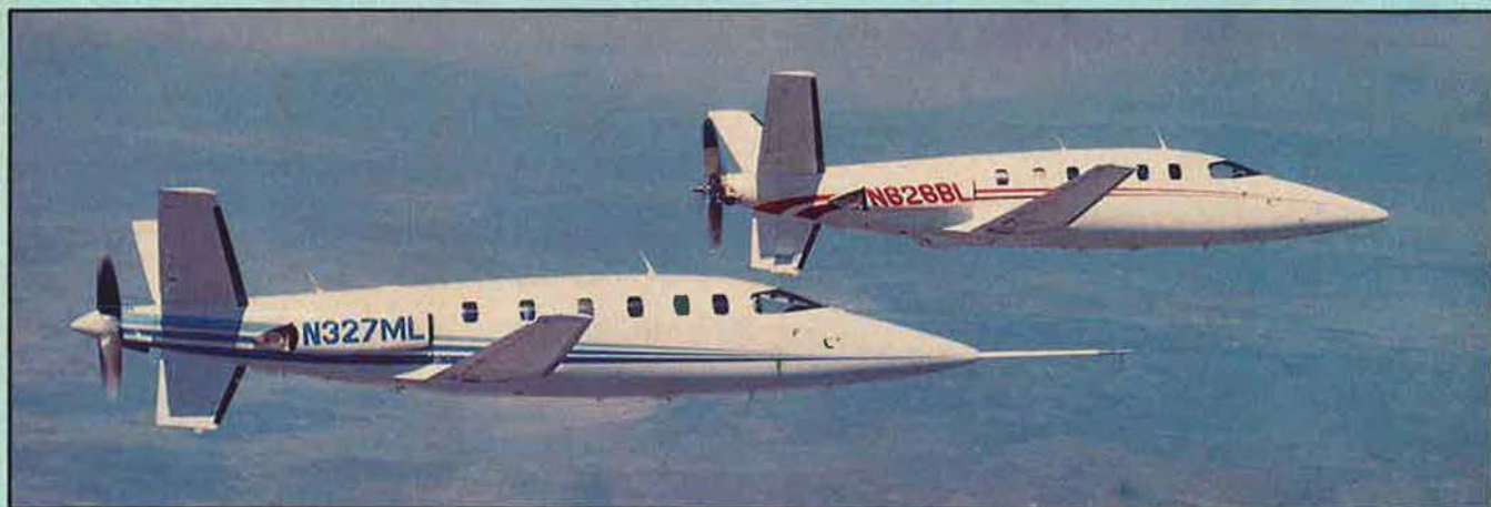
Production-configuration prototype of the Lear Fan Model 2100 (foreground) flying alongside the original prototype. Nose probe is temporary test equipment
