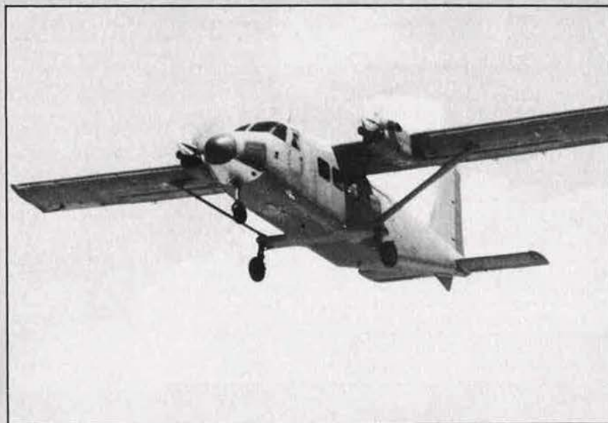
Prototype Harbin Y-11T1 Turbo-Panda 17-passenger STOL transport, photographed during first flight (David Ward)
