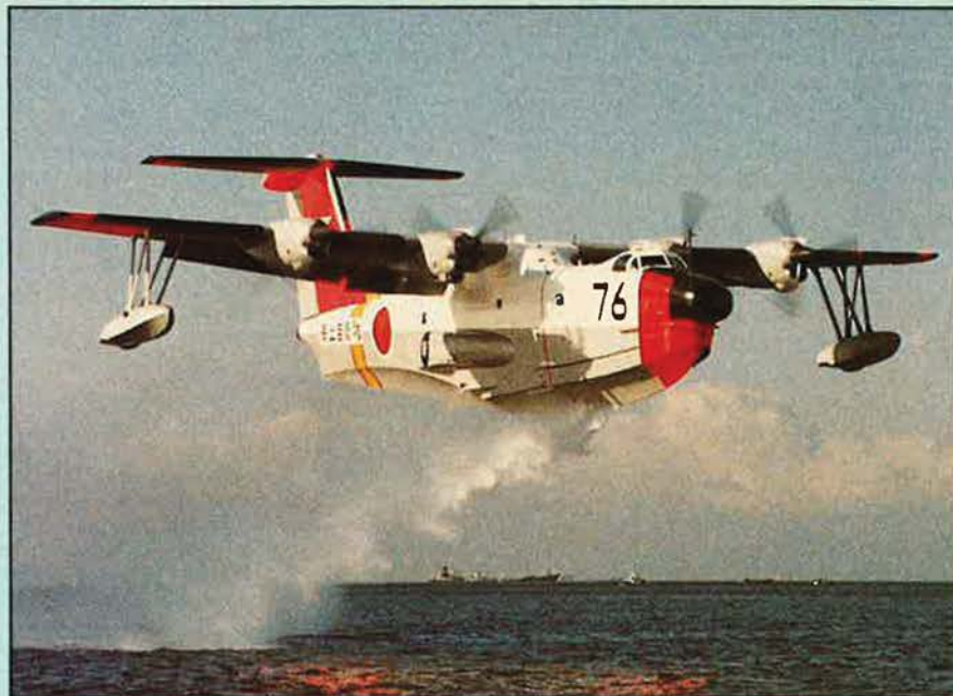
Shin Meiwa US-1 air/sea rescue amphibian (four Ishikawajima/General Electric T64-IHI-10 turboprop engines)
