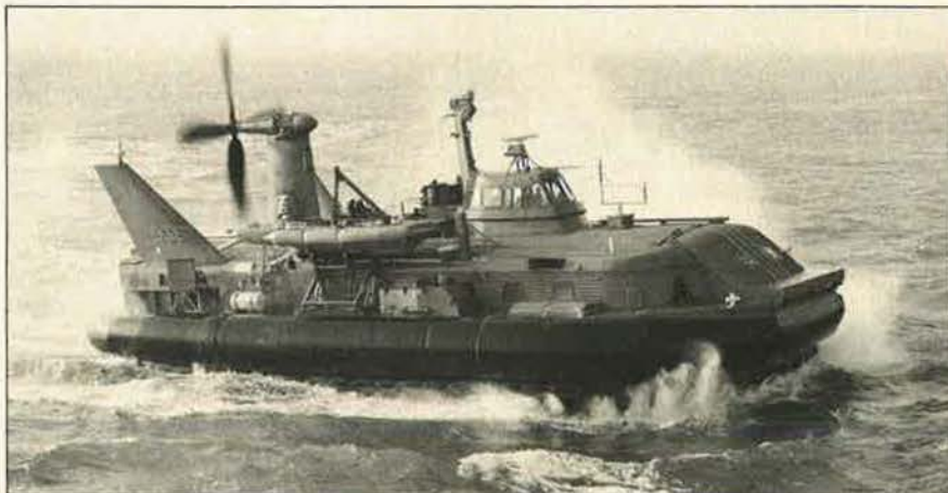
This Royal Navy Hovercraft BH7 Mk2 has successfully completed a series of mine countermeasures trials. According to officials, the Westland-built craft proved highly controllable, attained high transit speeds, demonstrated its ability to cross shallows and sandbanks, and operated from unprepared sites. With low underwater magnetic, acoustic, and pressure signatures, the craft is unlikely to explode mines although tests showed it virtually immune to underwater explosions. Another advantage: half the operational cost of conventional antimine vessels.
