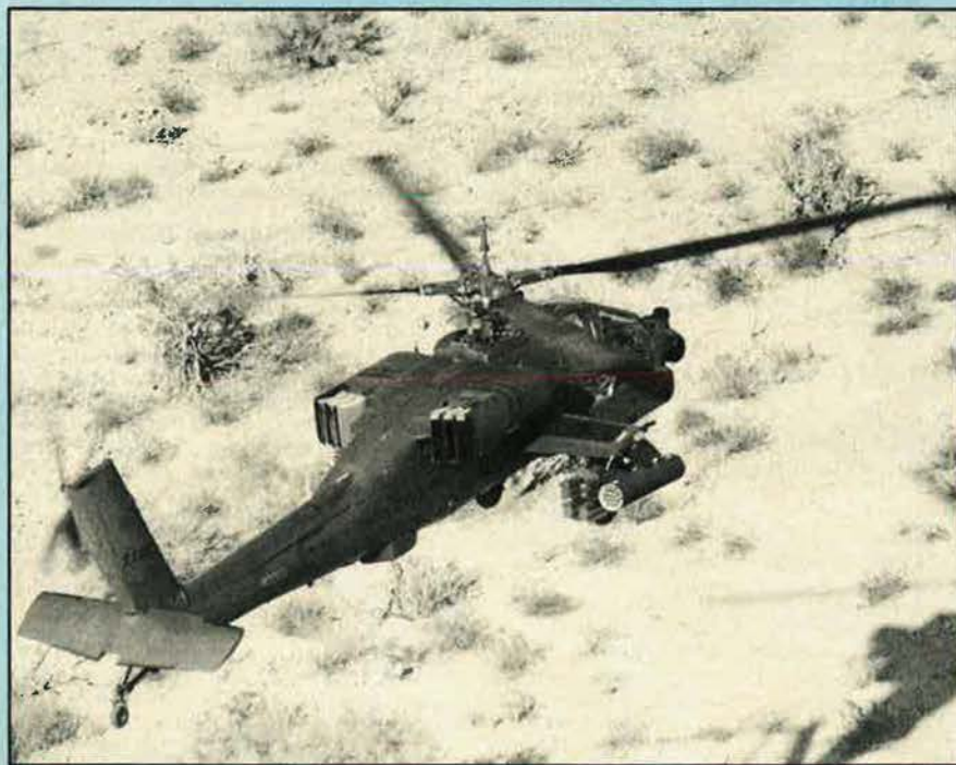
Low-flicker main and tail rotors, low-glint canopy, composite structural materials, IR suppression, and special paint to reduce the Apache's IR signature, cut detectability in nap-of-the-earth flight
