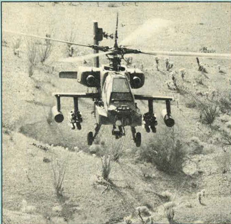
An Apache in typical nap-of-the-earth flight, armed with eight Hellfire missiles, 38 rockets, and a 30 mm Chain Gun automatic cannon
