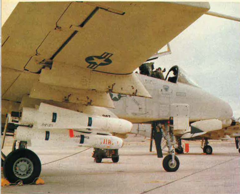
The IR Maverick, here mounted on an A-10 aircraft, is just over eight feet long and weighs about 500 pounds. Its digital centroid tracker picks up heat generated by a target, calculates the target's center, and guides the missile. The A-10's cannon and the IR Maverick complement each other. The gun is a certified tank-buster, but does not have the missile's standoff range.
