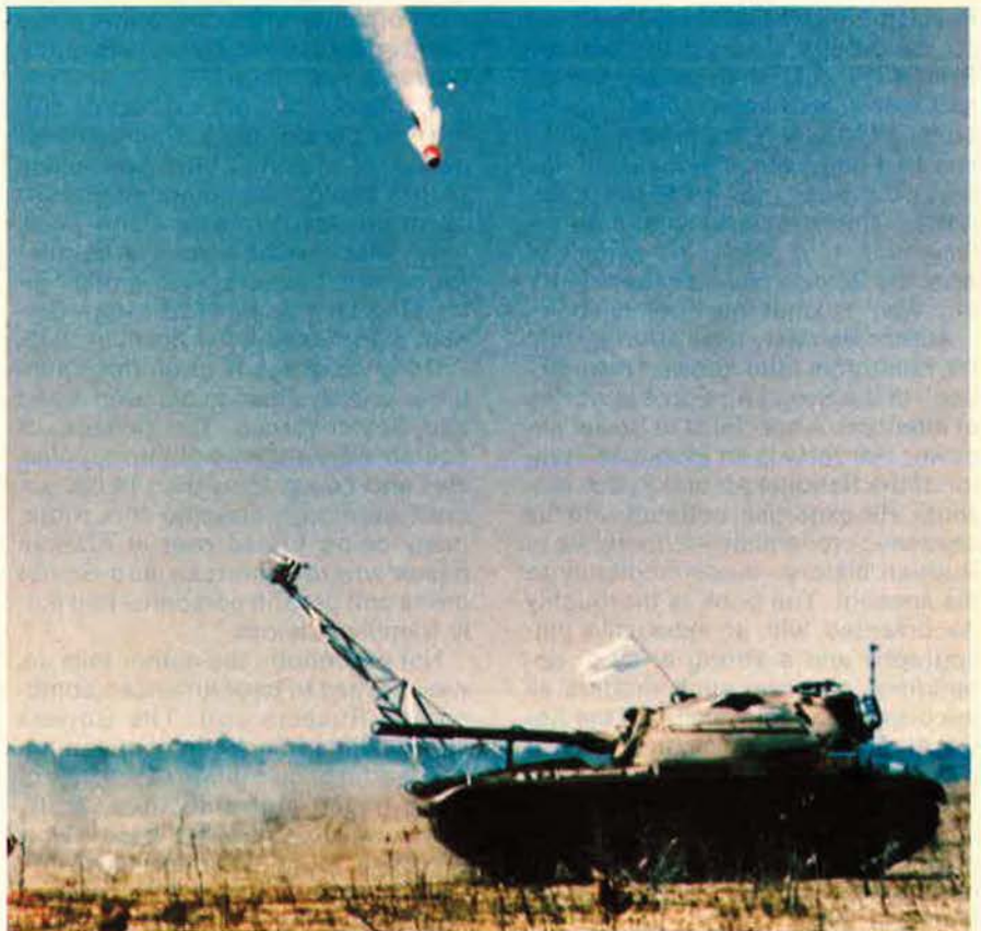
The Laser Maverick homes on a moving tank target. Its accuracy is impressive, but requires that a laser beam be played on the target until impact. The Air Force is acquiring Laser Maverick for the Marines, but does not plan to buy any for itself.
