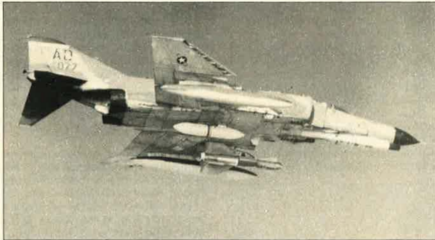
The GBU-15 Modular Guided Weapon System and its data link pod (located in center of the F-4's undercarriage) during flight tests at Eglin AFB, Fla. (See item below.)
