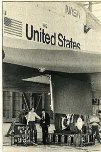
The main landing gear on this Space Shuttle vehicle is perched atop a platform of Goodyear air springs that serve as an isolation device, allowing the vehicle to "float free" from ground interference during tests.
