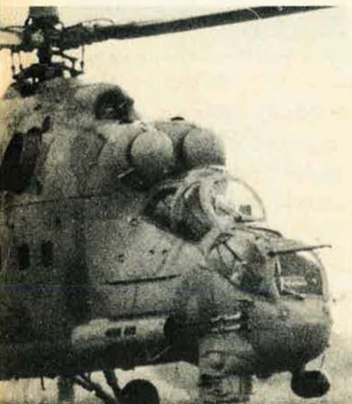
New version of 'Hind' with twin-barrel cannon in place of nose turret
