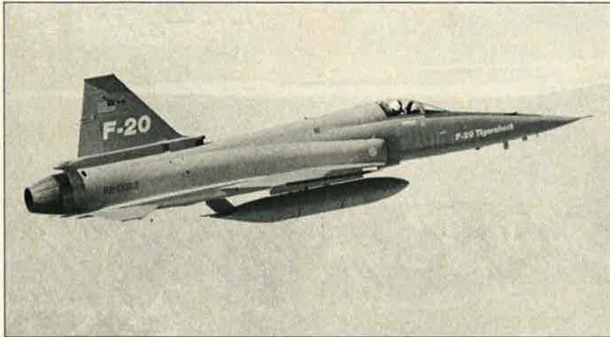
Northrop's new F-20 Tigershark tactical fighter carries an external fuel tank on its centerline station during a verification test to validate specific fuel consumption. As of late January, the F-20 had logged 124 sorties in its Flight Demonstration Program that started in August 1982 at Edwards AFB, Calif.
