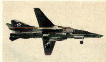
MiG-27 (NATO 'Flogger-J'). Note restyled nose, leading-edge extensions, and depressed barrel of gun in pod
