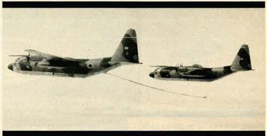
ABOVE: Hercules tanker and receiver, modified very speedily by Marshall of Cambridge for operations in the South Atlantic. LEFT: For Falklands service, RAF Nimrods were adapted quickly to carry bombs and missiles, in addition to installation of flight refueling probes.
