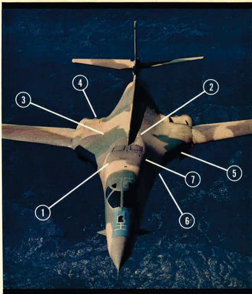
The main differences and improvements between the B-1B and the B-1A are listed here (the aircraft pictured is, of course, a B-1A): (1) new offensive avionics system; (2) movable weapons bay bulkhead; (3) simplified over-wing fairing; (4) simplified nozzle and neutral engine; (5) low radar cross section inlets and redesigned nacelles; (6) increased external stores capability (weapons and fuel); and (7) revised defensive avionics system. Other major differences (not shown) are: increased takeoff gross weight (477,000 pounds); composite structural Mode Control System, weapon bay doors and flaps; tail warning radar; air turbine starter revised gearbox; Advanced Centrally Integrated Test System and Electrical Multiplex.
