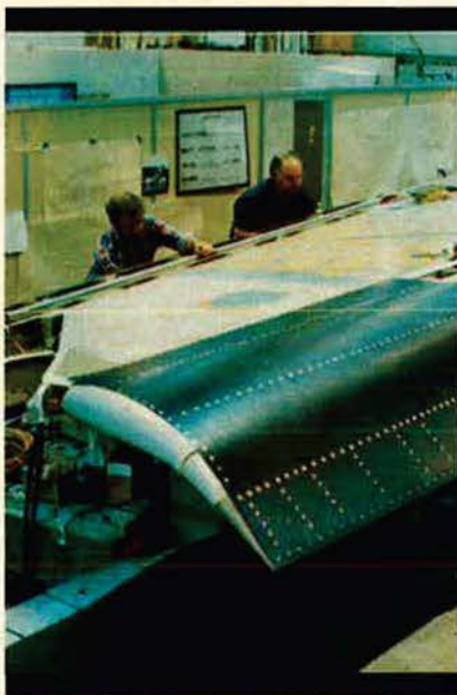
The mission adaptive wing, under fabrication by Boeing, will be able to vary its shape in flight with no break in the smooth contour of its upper surface.
