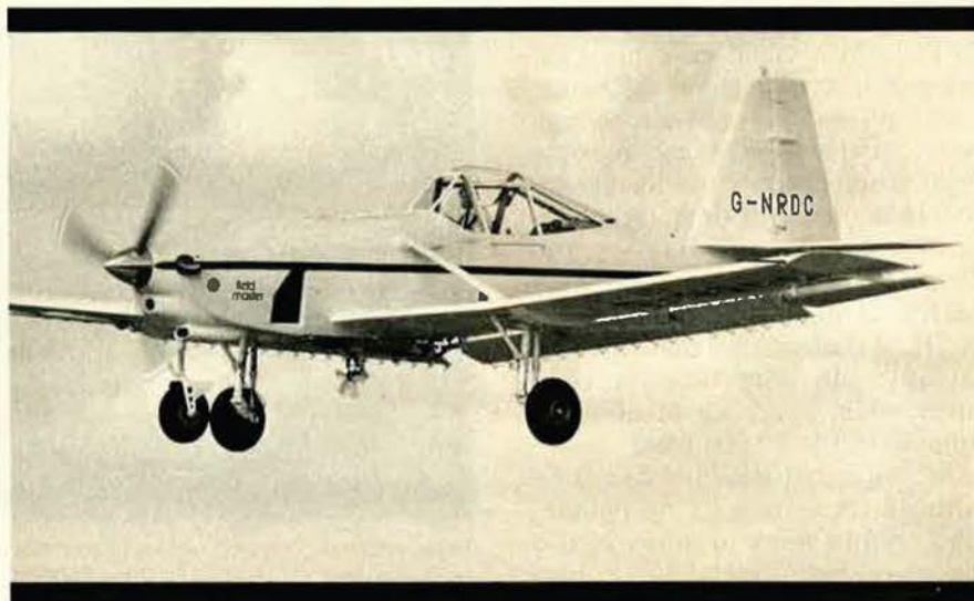
Carrying more than two tons of chemical in its titanium hopper, which forms an integral part of the fuselage structure, the NDN Fieldmaster makes a formidable addition to the world's fleet of agricultural aircraft. Some 26,000 fixed-wing aircraft and helicopters are used in agriculture worldwide. (Brian M. Service)
