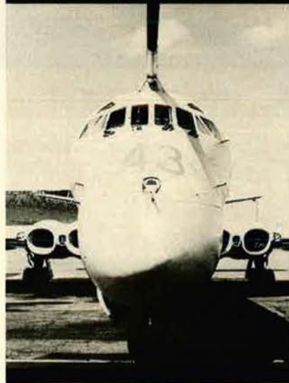
ABOVE: Hercules tanker and receiver, modified very speedily by Marshall of Cambridge for operations in the South Atlantic. LEFT: For Falklands service, RAF Nimrods were adapted quickly to carry bombs and missiles, in addition to installation of flight refueling probes.
