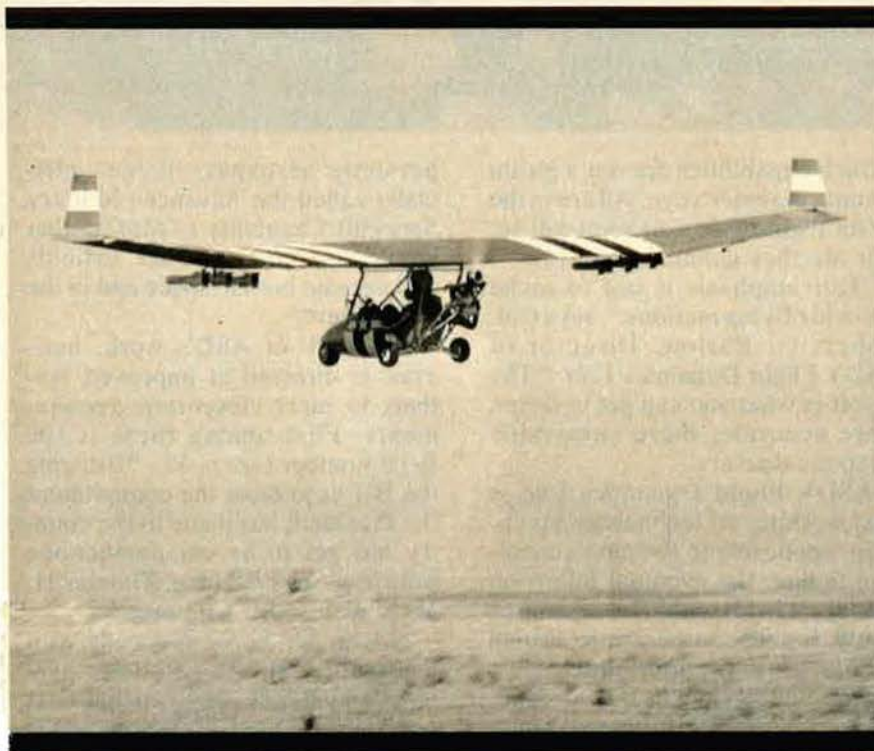
The "missiles" under the wings of this Mitchell SR-10 microlight are made of wood, but aircraft as simple and inexpensive as the SR-10 may soon become combat equipment of at least one Middle Eastern air force. Such aircraft could operate as pilotless "kamikazes," diving into their target armed with a warhead.
