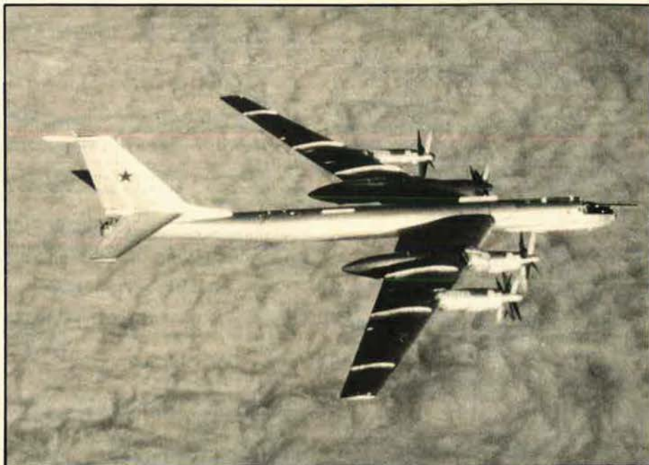
The Soviet Bear F is a much-refined antisubmarine version of the Tu-142. Like other models of the Bear, it has long range and endurance. The purpose of the projection from the rear of the fin tip is not known.
