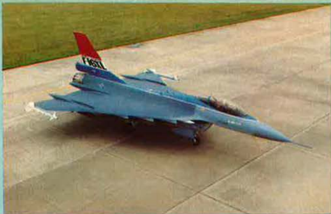
The new 'cranked-arrow' wing and lengthened fuselage of the F-16XL are evident in this view
