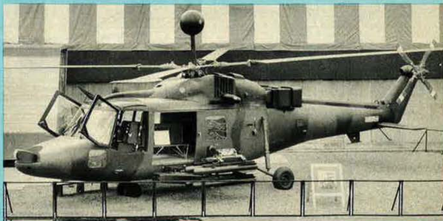
Impressive mockup of the Westland Lynx-3 at the Farnborough Air Show displayed mast-mounted sight and Hellfire missiles (Brian M. Service)
