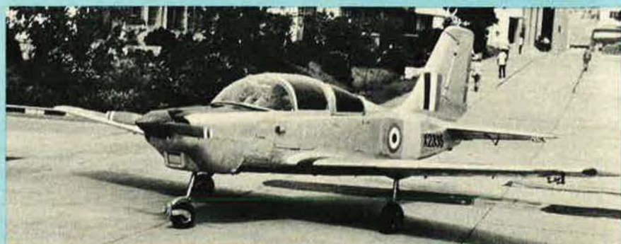
Third prototype of the HAL HPT-32 multi-role trainer, representative of 40 ordered for the Indian Air Force
