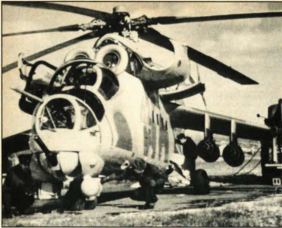
The Soviet Mi-24 Hind helicopter began as a platform to ferry troops to the battlefield, but recent versions—such as this D model—have been redesigned as gunships.
