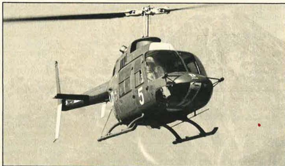
Among its seven helicopter squadrons, the Austrian Air Force has thirteen Agusta-Bell 206A JetRanger IIs for communications and other specialized duties.
