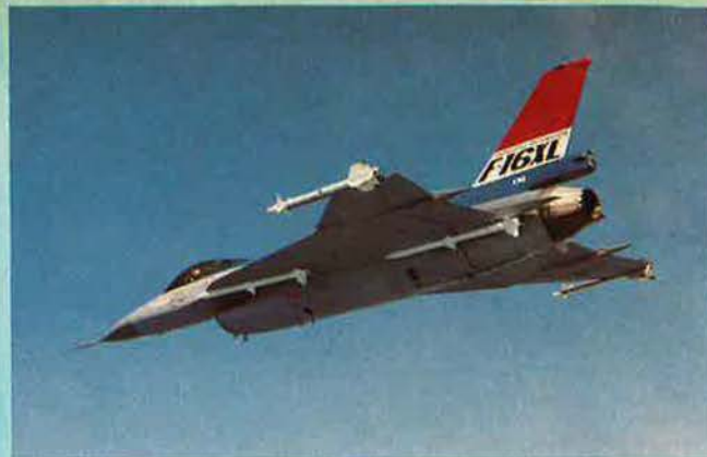
The F-16XL offers a doubled weapons load and 45% greater combat radius on internal fuel compared with the standard F-16A
