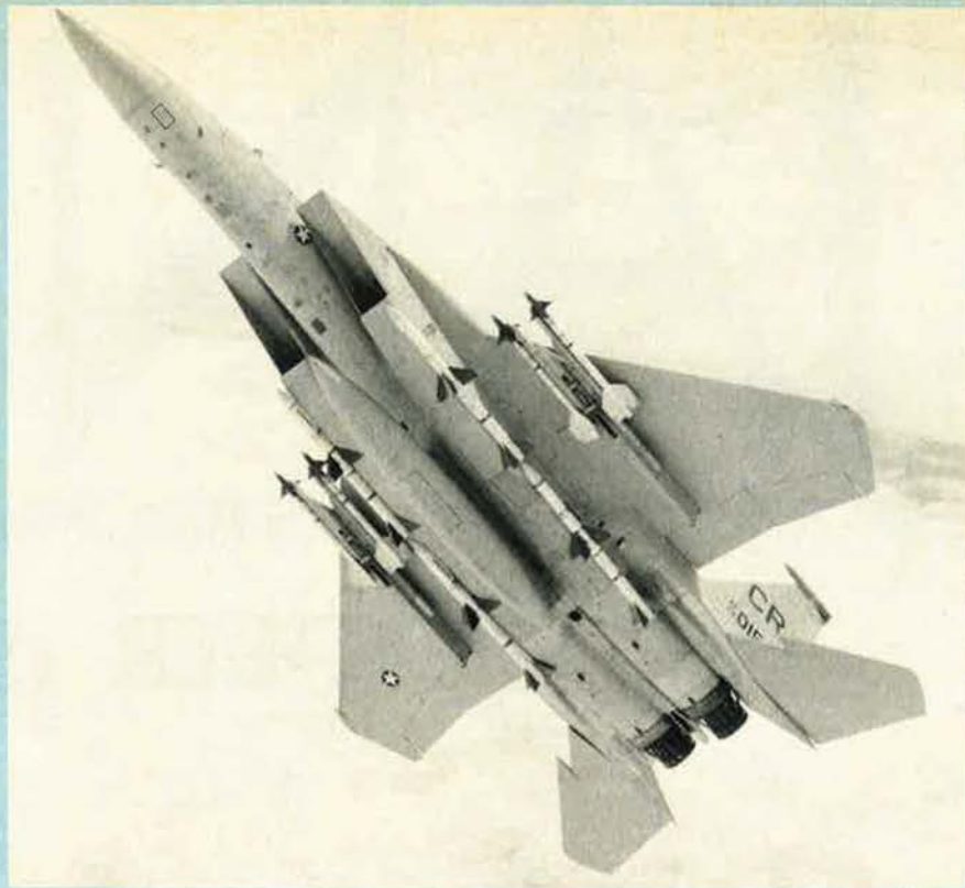
This F-15C of the 32d TFS demonstrates the climb rate that enabled an Eagle to set six current world time-to-height records. Armed with weapons like these AIM-7 Sparrows and AIM-9L Sidewinders while in service with overseas air forces, Eagles have scored impressive victories over opposing MiG-21s, -23s, and -25s
