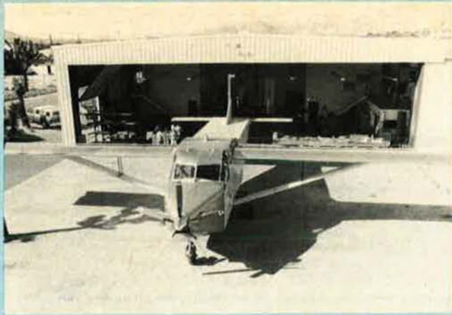
GafHawk 125, designed to haul a useful load equivalent to its own empty weight on the power of a single turboprop engine
