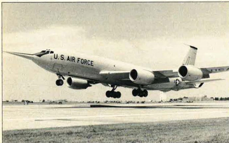
The first Air Force KC-135 tanker to be equipped with the new, fuel-saving CFM56 turbofan engine shown on its maiden flight. The reengined aircraft will provide one-and-a-half times the fuel offload capacity of the present KC-135As. (See item.)
