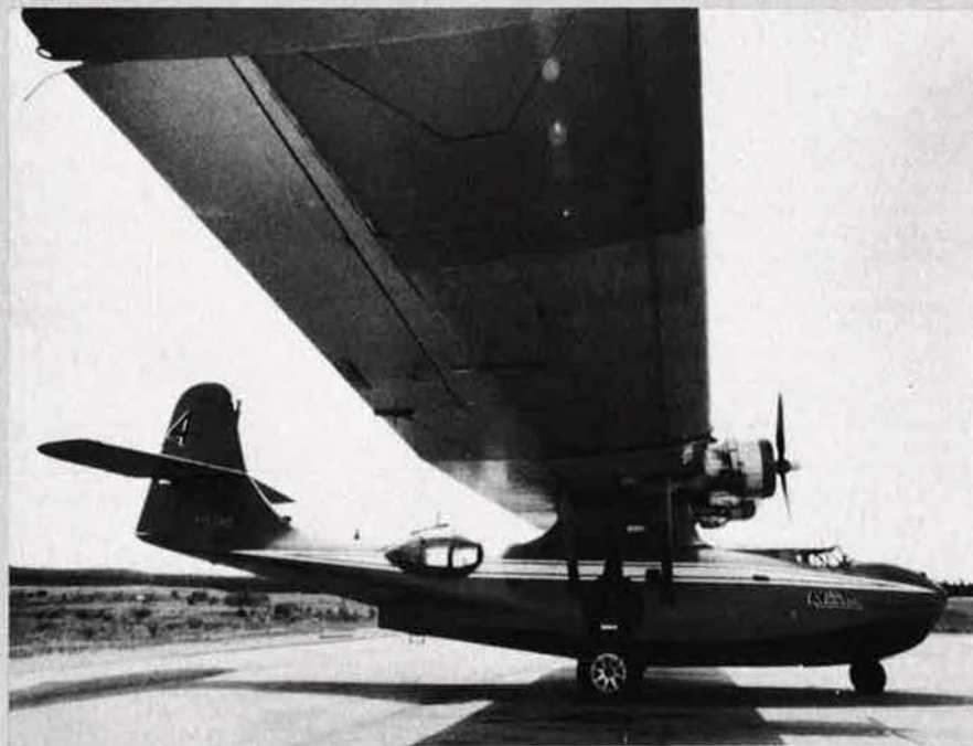
Avalon Canso water-bomber, converted from a Consolidated/Convair PBV Catalina-type maritime patrol amphibian
