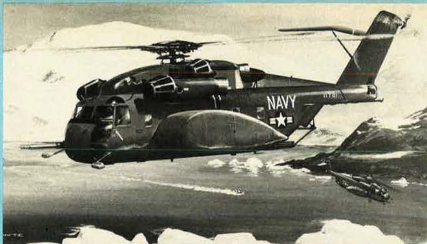
Artist's impression of the fully-developed MH-53E mine-sweeping helicopter, with increased fuel in oversize spsonsons
