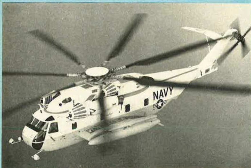
The Sikorsky CH/MH-53E, a production CH-53E Super Stallion which has been modified to flight test features of the mine-sweeping MH-53E
