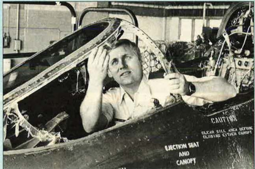
Idaho ANG Lt. Fred Wilson inspects the shattered windscreen of the F-4C he landed from the backseat following a bird strike. A navigator, he had never before landed a Phantom. (Photo by David R. Frazier)
