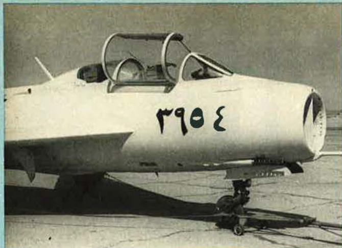
Close-up of front of the Chinese-developed tandem two-seat trainer version of the MiG-19 (Denis Hughes)
