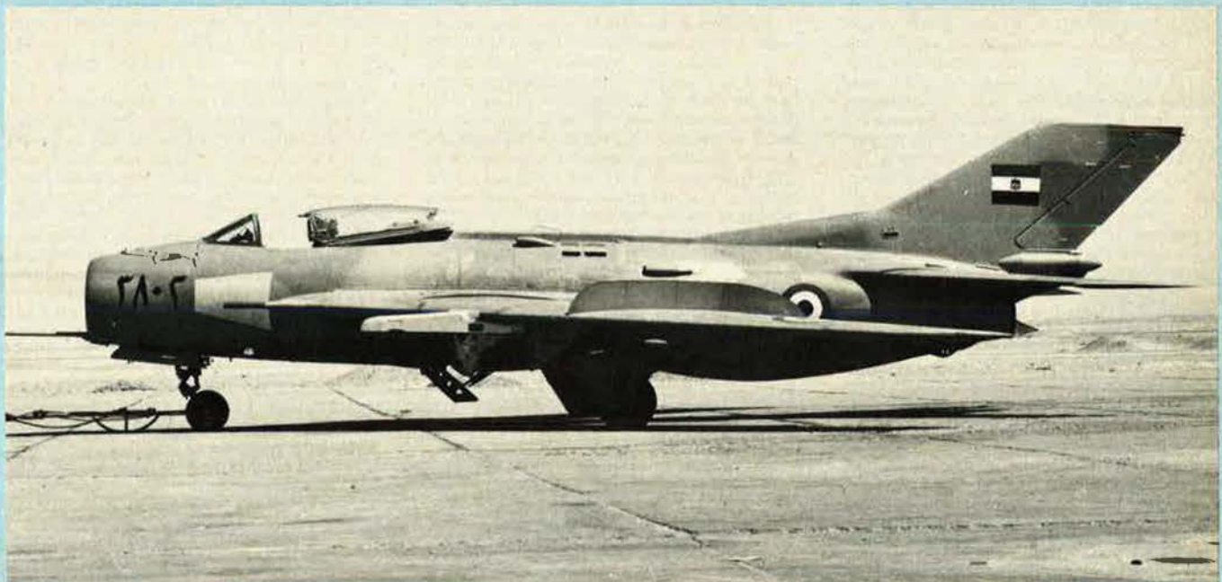
Jian-6 (MiG-19SF) single-seat day fighter of Egyptian Air Force; late production version with relocated brake-chute (Denis Hughes)
