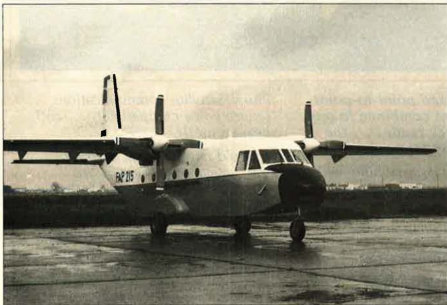
Spain's CASA aircraft manufacturer has delivered this first of three STOL-capable C-212 series 200 military transports to Panama. Other Central American nations interested in the light transport are Costa Rica and Nicaragua. Although designed primarily to deliver military cargo, troops, and parachutists, the aircraft can be quickly reconfigured for civil flights. Some 220 have been built thus far to fill orders by twenty-seven countries worldwide.
