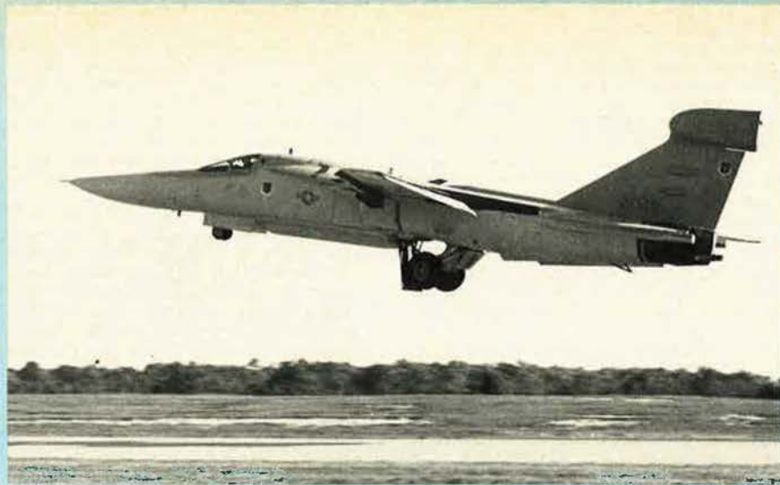
Second prototype (66-049) of the Grumman (General Dynamics) EF-111A electronic warfare aircraft was used for flight testing the complete jamming system
