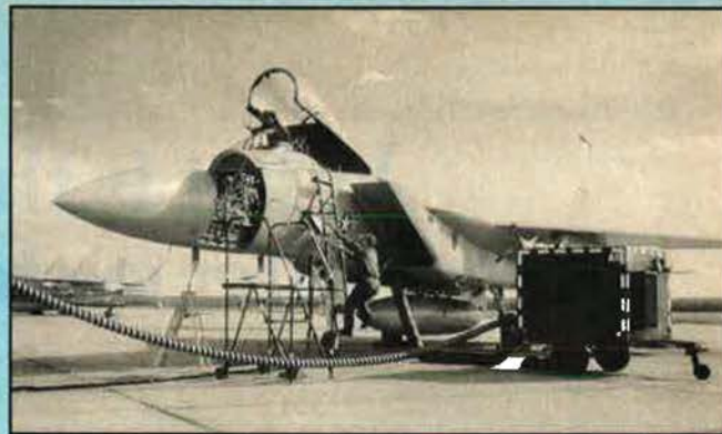
The F-15, with greater combat effectiveness, requires only three-fourths the maintenance time of the F-4, as seen here at Cold Lake, Canada, during an exercise.
