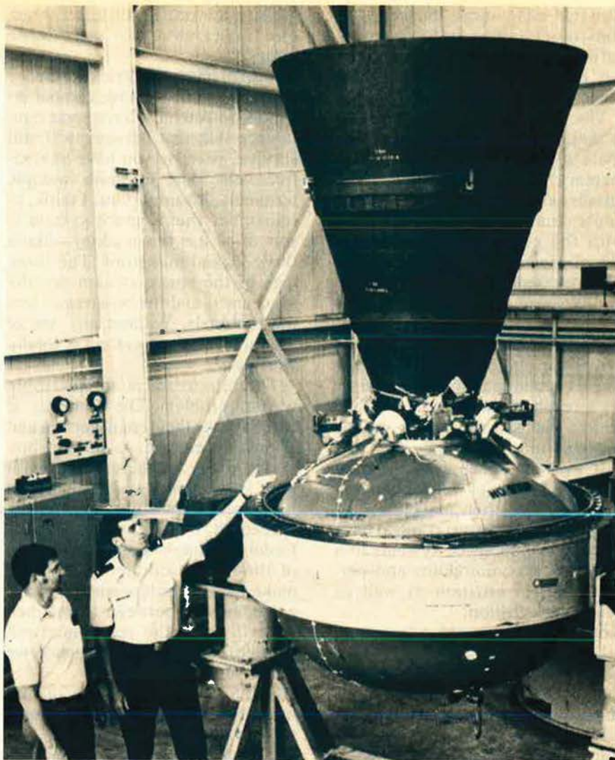
Inertial Upper Stage (IUS) motor. USAF is developing and producing the IUS, which provides the capability to deliver spacecraft from the Shuttle parking orbit to higher orbits, such as geosynchronous.
