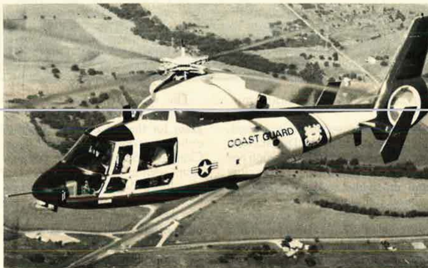
Coast Guard Aviation, in performing its wide range of missions, relies on the workhorse HC-130 and the HH-3F (opposite page). An equipment upgrade is in progress, with the introduction of the HH-65A (above), which is slated for the primary role of short-range search and rescue.
