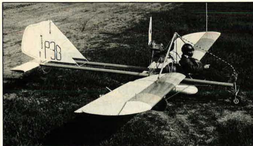
Built by Mitchell Aircraft Corp., Porterville, Calif., an ultralight for other than recreational flying. This full three-axis aircraft can carry a pilot and fifteen gallons of agricultural chemicals for low-volume application. The ultralight, powered by a thirty-hp engine, can cruise at fifty-five mph and is also designed for fence patrol and irrigation surveillance. The plane lands at thirty mph and its wings can be folded in less than five minutes for storage.
