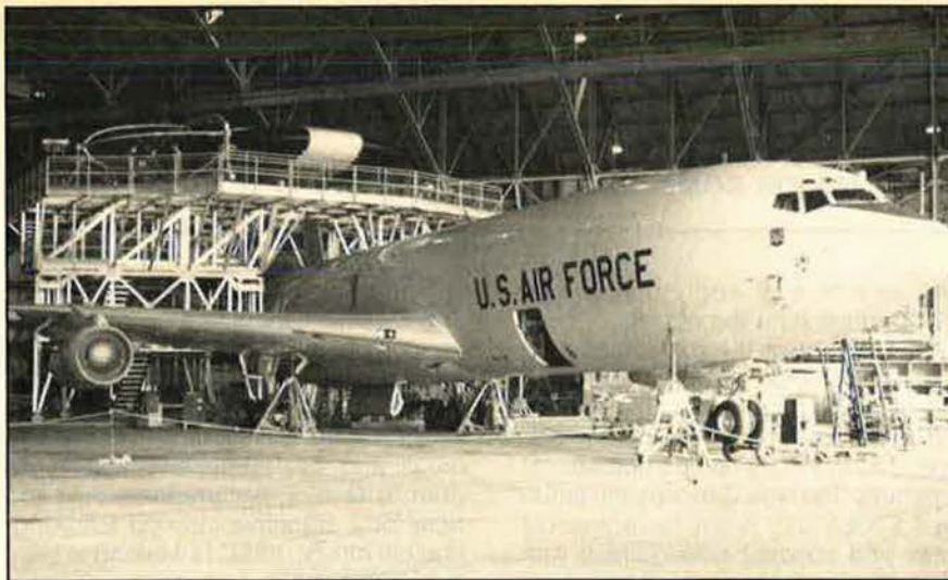
The Erector-Set-like structure allows work to be done on the radome of an E-3A Sentry aircraft at the AFLC Oklahoma City Air Logistics Center. The Center has worldwide logistics management responsibility for the E-3A as well as the -135 series and the B-52 fleet. It also has been designated logistics manager for the new B-1B.
