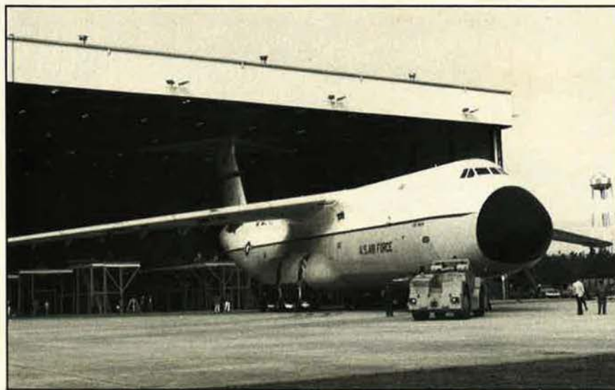
Powerless giant bird with its wings removed, the first of seventy-six C-5As to receive new wings is backed into a hangar at Lockheed-Georgia Co. facilities in Marietta. The aircraft's new wings are constructed of new aluminum alloys specially heat-treated to extend the aircraft's life well into the next century.
