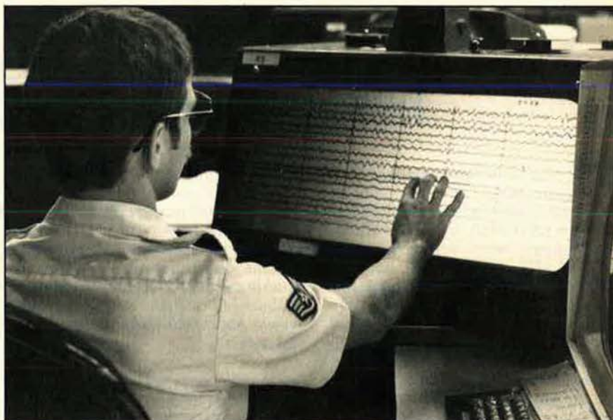
AFTAC conducts an extensive seismological research program to detect nuclear weapons testing underground: here, an AFTAC technician measures seismic signal waves.
