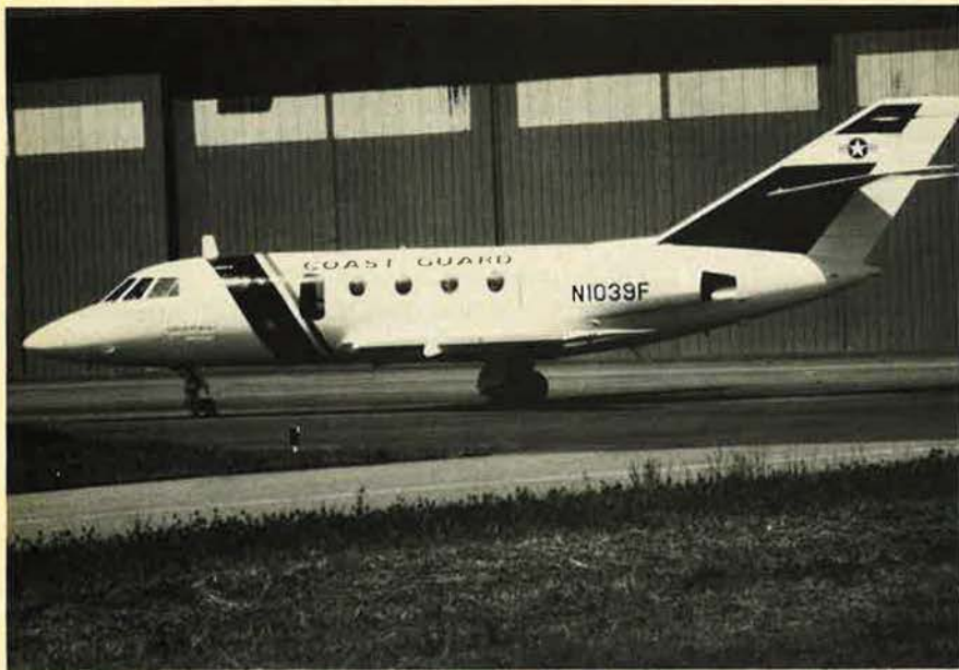
Coast Guard Aviation is also acquiring the HU-25A, capable of high dash speeds. Besides its search-and-rescue role, the aircraft will haul oil pollution sensor systems to aid in locating and identifying spill sources.
