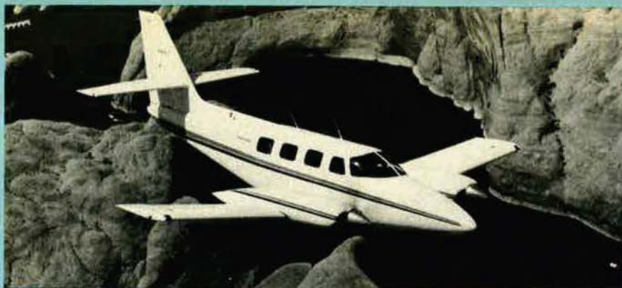
Features of the Crusader include bonded construction, a cruciform tail, counter-rotating propellers, and full equipment for IFR operation
