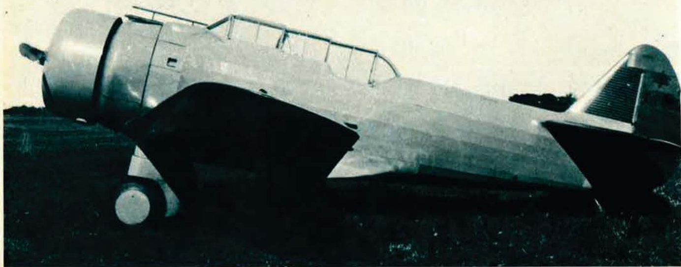
The beginning of more than 20,000 successful trainer aircraft: Prototype NA-16, photographed on August 26, 1935, after being modified with an enclosed canopy and wheel fairings. (Norm Avery)
