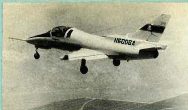
The Peregrine prototype, shown here at the time of its first flight is single-engined; the production model has been redesigned around two Williams FJ44 turbofans
