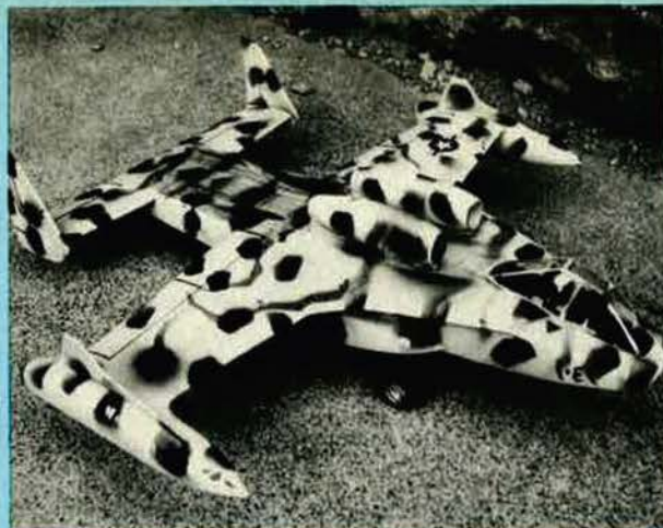
IML AX in desert camouflage scheme. The long-range tip tanks give the aircraft range comparable to that of the F-111
