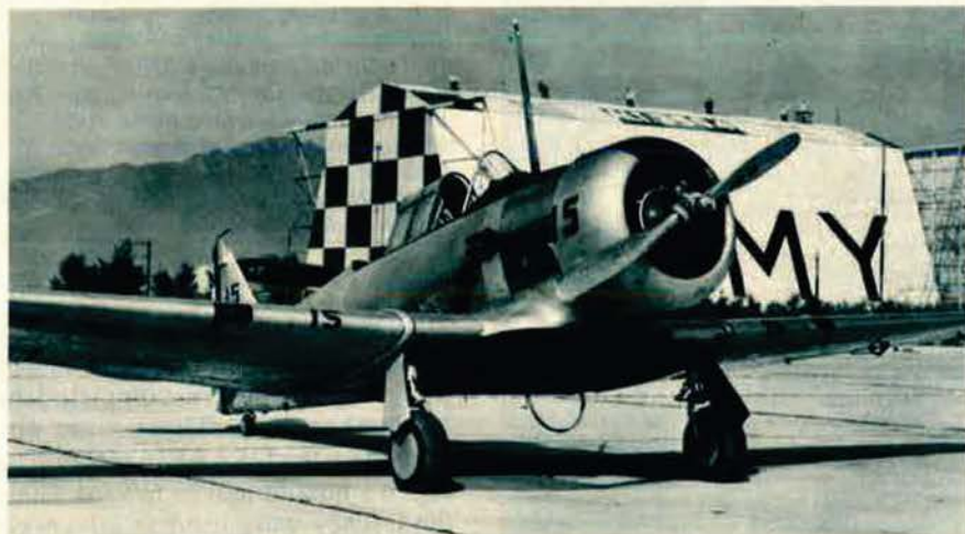
ABOVE: The BC-1, with a fabric-covered fuselage, was the first version of the trainer to have retractable landing gear. The Basic Combat designation allowed AAC to order the aircraft, as there was no money in the trainer budget. (Dusty Carter/AAHS) LEFT: The BC-1A took on all the characteristics of the future AT-6, excepting the DF loop, fuel selector blister under the center section, and the venturis on the sides. (USAF photo)
