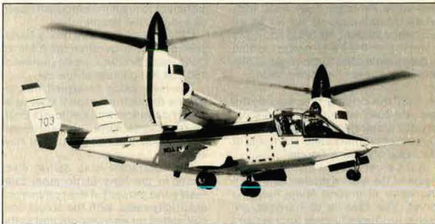
The Bell Helicopter Textron XV-15 tilt-rotor aircraft is being developed by the Army, Navy, and NASA. The XV-15 ascends and hovers like a helicopter, and, with rotors tilted forward, flies like a fixed-wing aircraft. See item below.
