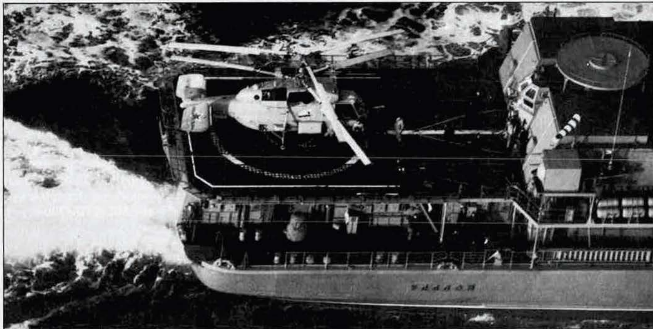
In the Baltic Sea, this high-angle photo shows the Soviet "Helix" helicopter on the hangar deck of the Soviet guided-missile destroyer USSR Udaloj. The helicopter is an apparent variant of the Kamov Ka-25, and is cited in the "Gallery of Soviet Aerospace Weapons," March 1982 issue, p. 105. (US Navy photo)
