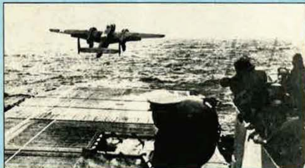
A B-25 struggles into the air off the deck of the carrier Hornet on April 18, 1942, on its way to bomb Japan. Pilots were instructed to keep the nosewheel and left wheel on the white lines at left of the deck to ensure clearing the superstructure.
