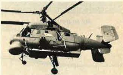
Kamov Ka-25 with underbelly container for wire-guided torpedoes
