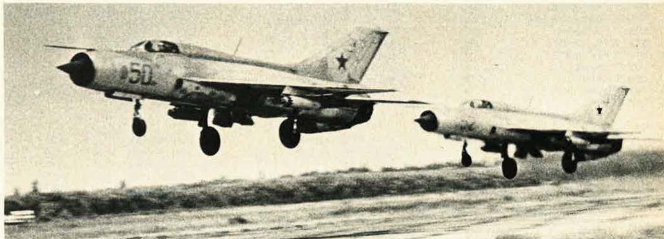
MiG-21PF aircraft, Fishbed-Ds, have no gun, but carry a variety of external ordnance and have enhanced all-weather capability.
