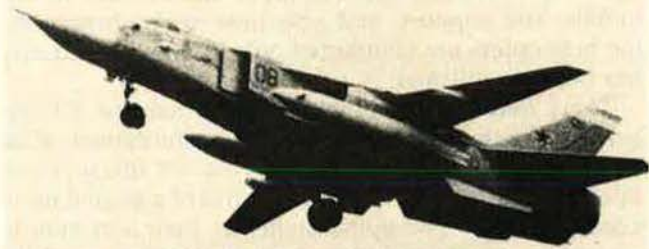
The most formidable Soviet fighter, the Su-24 or Fencer, is a ground attack aircraft carrying pilot and weapon system officer.
