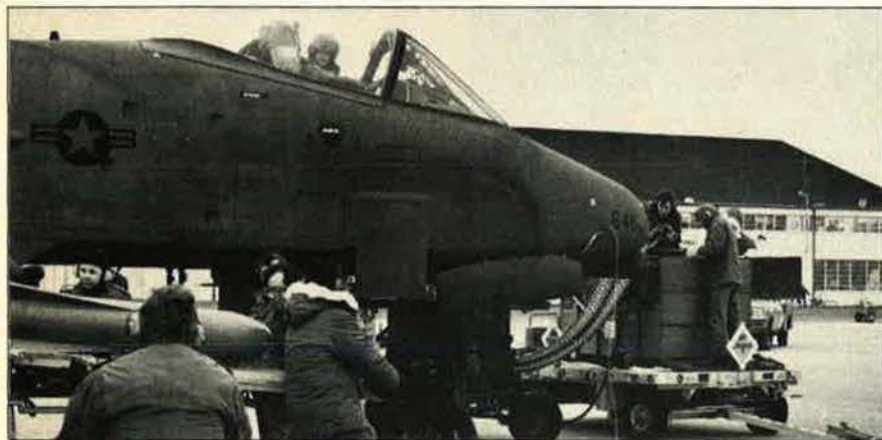
"Flying Yankees" of Connecticut ANG's 103d Tactical Fighter Group at Bradley IAP, Windsor Locks, practice rapid "Integrated Combat Turn" on a unit A-10, during which the aircraft is refueled and rearmed simultaneously. All actions—including the pilot's intelligence or flight-plan briefing—are conducted at the revetment.
