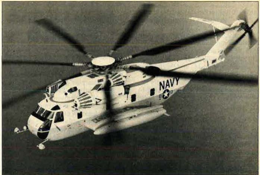
Latest in a series of Sikorsky helicopters being built for the Navy and Marine Corps, the CH-53E is a preproduction prototype designed primarily to tow magnetic or electronic gear in a minesweeping role. The triple-turbine, heavy-lift Super Stallion, the free world's largest helicopter, is also equipped for in-flight refueling for long-range, long-duration missions.
