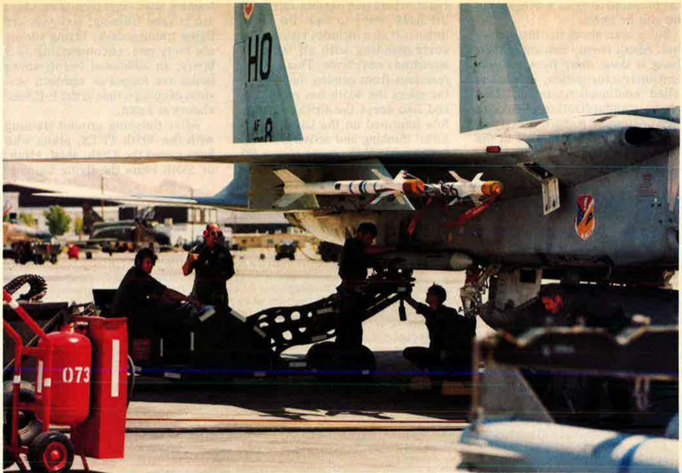
Fighter training also includes building ties with the men and women who make the missions possible. Here, at the operational 49th TFW, munitions experts upload Sparrow and Sidewinder missiles on an F-15.
