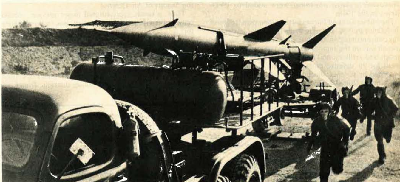
An SA-2 surface-to-air missile, NATO code name Guideline , on its mobile transporter-launcher. The SA-2 is a medium-range (40–50 km), radio-controlled air defense missile in service in the USSR and some twenty other nations.
