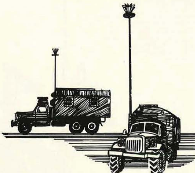
UHF radio links for strike control would be jammed by the mobile basket-antenna jammer unit.
