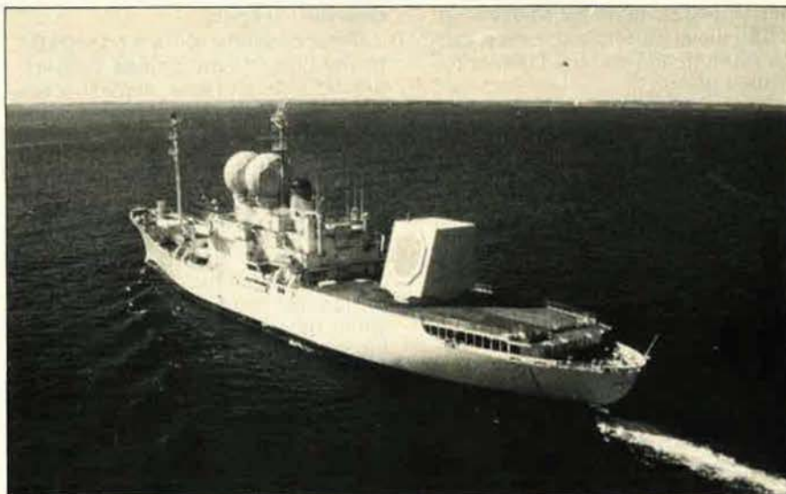
Following trials in the eastern Atlantic, the Air Force's shipborne phased-array radar COBRA JUDY is now slated for a test session in the Pacific. Operating out of its home port of Pearl Harbor, Hawaii, the radar station aboard the USNS Observation Island will accumulate data on ballistic-missile flights. The largest such sensor system afloat, COBRA JUDY stands four stories tall and weighs 250 tons. It was developed by Raytheon Co. for AFSC's Electronic Systems Division.
