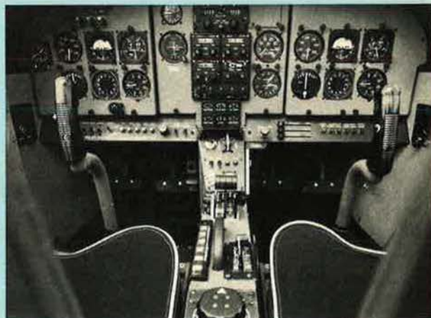
The cockpit of the new Finnish L-70 miltrainer is equipped so that night and instrument flying can be taught.
