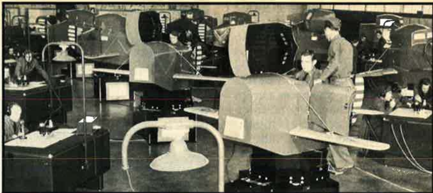
With the hood down, the Link trainer provided an overheated and uncomfortable ride—but proved to be a technological breakthrough and the precursor of today's cockpit simulators. (National Air and Space Museum photo)
