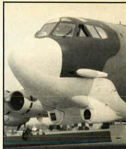
Night and adverse weather terrain avoidance penetration is possible through use of the B-52's electro-optical viewing system, shown here.
