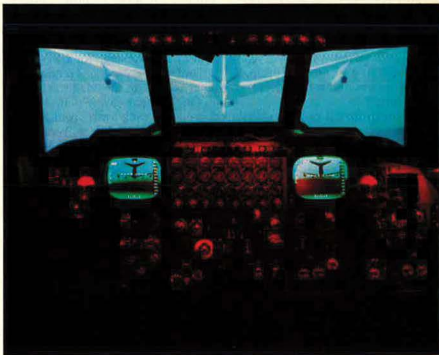
Realistic simulation in a B-52 WST cockpit with digital-image generated aircraft underbody during aerial refueling scenario.
