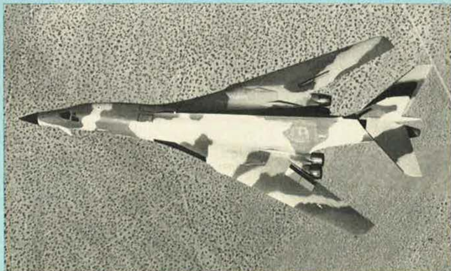
With its variable-geometry wings fully swept, the B-1 was designed to fly a Mach 2 when required. Such performance is not specified for the new B-1B version
