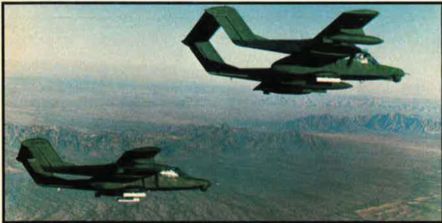
Two Marine Corps OV-10D Bronco night observation surveillance aircraft bank in formation over the maneuver area. The Bronco was first used by USAF and USMC as forward air control aircraft. The North American-built aircraft carries a wide range of weapons and sensors in the NOS role.
