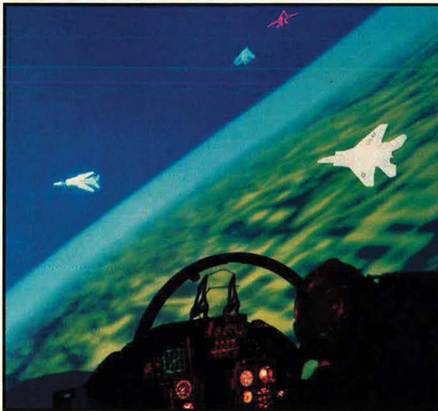
An F-15 pilot and his wingman pursue simulated enemy projected on the interior dome of this Manned Air Combat Simulator at McDonnell Douglas Corp.
