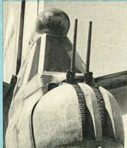
Above: Port wingtip extension device for engaging flight refuelling hose trailed by Tu-16 tanker. Above and below are red lights protected by heavy mesh guards.
