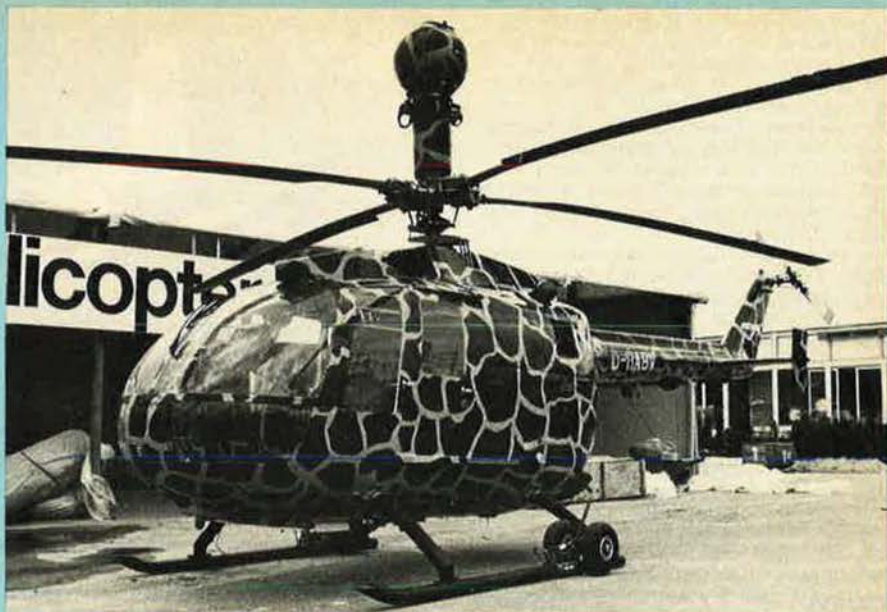
When the tall mast-mounted sight of this BO 105 scout helicopter caused it to be named 'Giraffe', MBB added unique and appropriate camouflage (Air Portraits)
