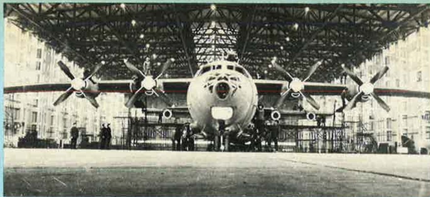
Assembly line of Hanzhong Y-8 transports, Chinese versions of the Antonov An-12BP
