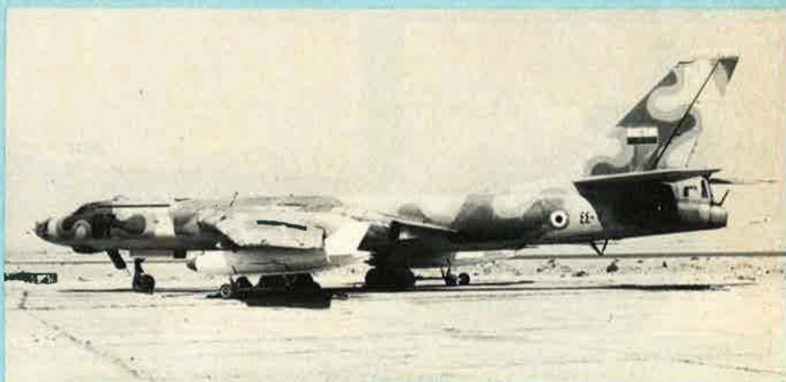
Tupolev Tu-16 ('Badger-G') of Egyptian Air Force, photographed at Cairo West aerodrome. Small wheels visible under the wings belong to handling trolleys for the 'Kelt' missiles on underwing pylons (Denis Hughes)
