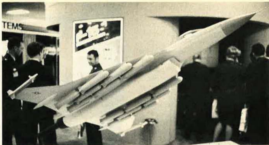
Visitors to the AFA briefings and displays saw and were briefed on the General Dynamics F-16XL, a cranked-arrow wing version of the "Fighting Falcon" slated for first flight in July 1982.
