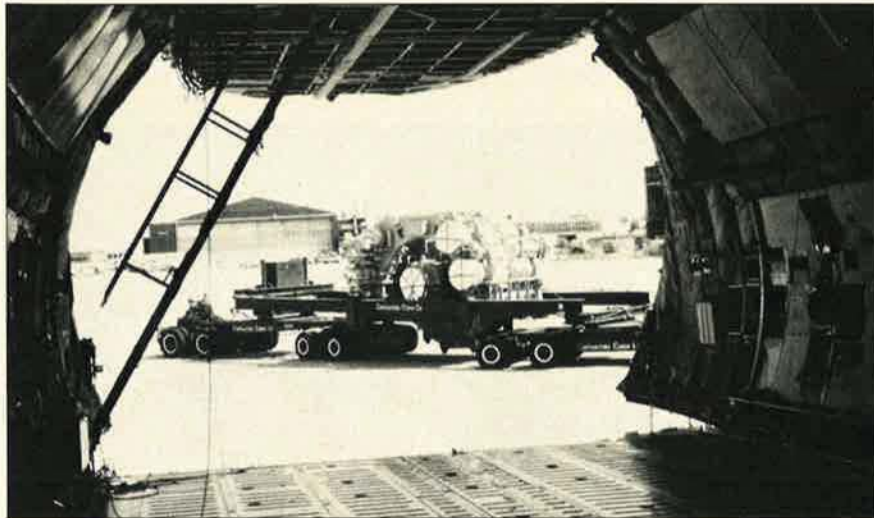
A long-term program that is saving the US Navy time and money involves Air Force C-5s transporting sixty-five-ton ships' transmissions from the manufacturer in California to Maine, where some of USN's new frigates are being built. Another benefit is that the transmissions can retain their "assembled-as-tested" status. The program, begun in early 1978, should continue for the next six to ten years. The transmission payload has set a record for weight carried in the C-5.
