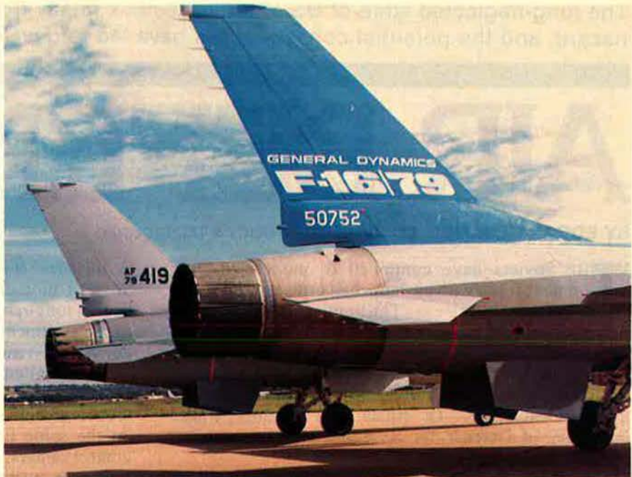
This side-by-side photo shows the eighteen-inch longer J79 engine compared with the F100 (background, on 79419). Tail cone fairing is also seen. Inside the airframe, different mounting points in the engine cavity accommodate the J79.
