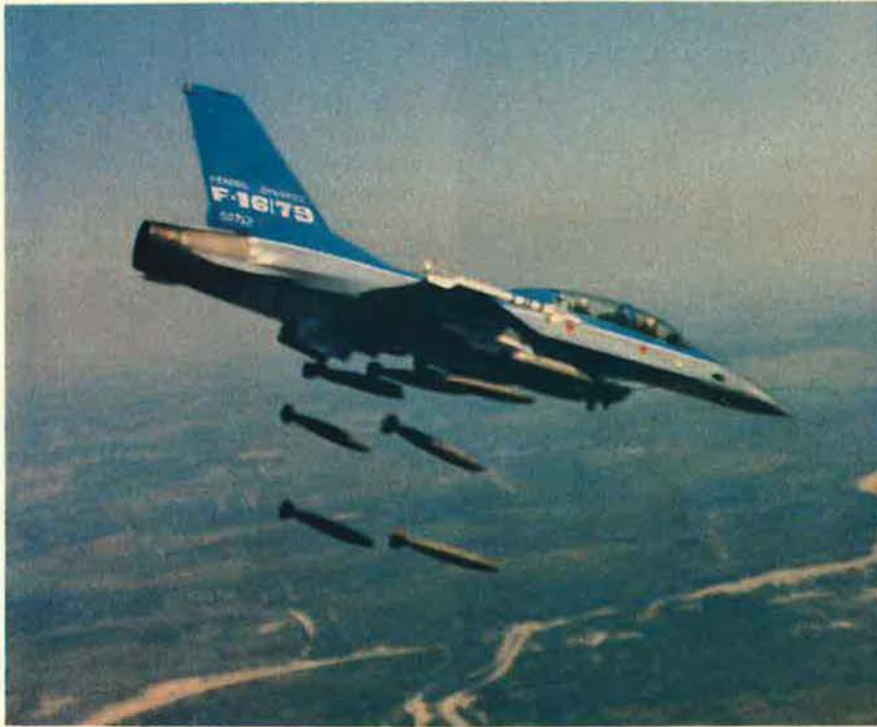
F-16/79 drops a partial load of Mk-82 500-pound bombs during its certification and qualification flight test development program.
