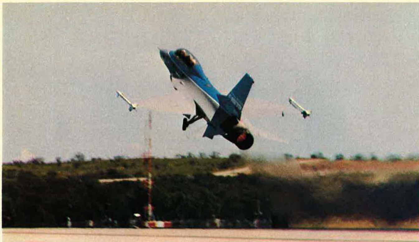
Sharp nose-up pitch angle and heat waves from afterburner are clearly shown in this takeoff photo of the F-16/79. Aircraft rotated after eight-second ground roll, and was passing through 1,500 feet within twenty seconds after brake release.
