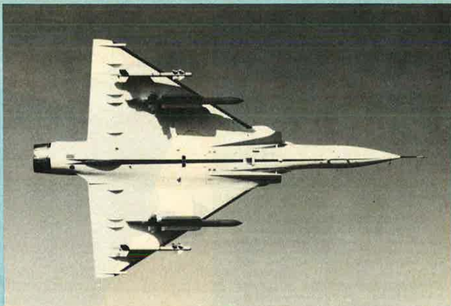
Mirage 2000 with basic interceptor armament of two Super 530 and two Magic air-to-air missiles
