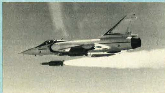
Launch of a Matra 530 long-range air-to-air missile from a Mirage 2000
