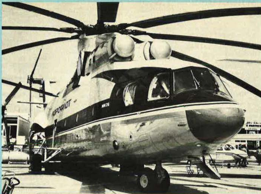
The blistered flight deck windows are shown clearly in this close-up of the Mi-26 taken at the recent Paris Air Show (Brian M. Service)
