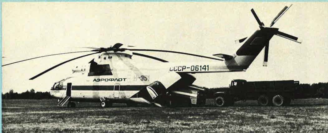
Heavy vehicles boarding the Mi-26, which has a payload and cargo hold comparable in size to those of a C-130 (Tass)
