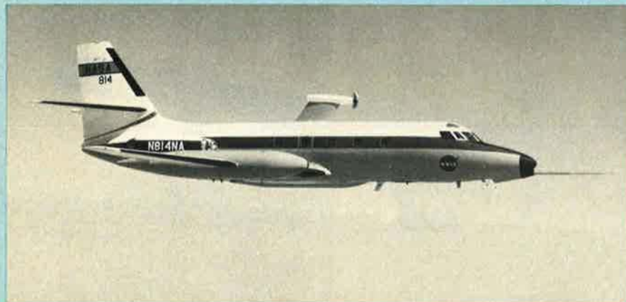
NASA's C-140 JetStar as modified for propfan acoustical tests
