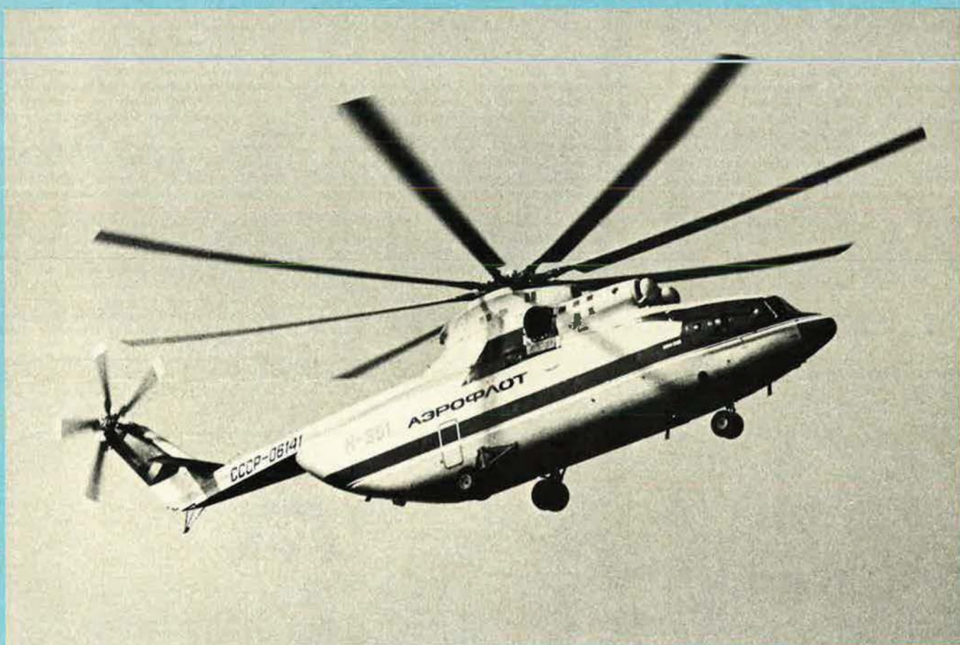
Mil Mi-26 heavy-lift helicopter (two Lotarev D-136 turboshaft engines) (Tass)
