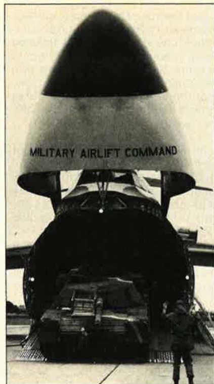
The first operational C-5 refitted with new wings unloads a sixty-ton Abrams tank during flight evaluation. The aircraft has logged more than 550 hours in worldwide missions during the test program.
