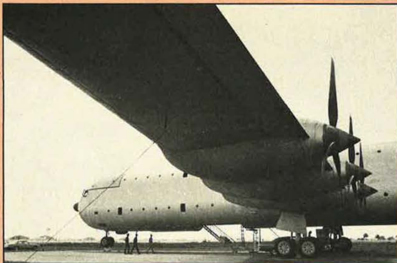
Above, at 230 feet the XC-99's wingspan is seven feet longer than that of the C-5. Left, a view of three of its six "pusher" Pratt & Whitney Wasp engines. (Photos by William A. Ford) Below, on takeoff long ago.
